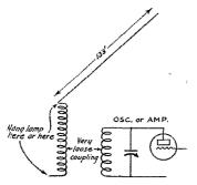
FIG. 5 — USING A RESONANT COUPLING COIL WITH THE END-FED HERTZ ANTENNA
