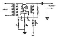
FIG. 2-GRID AND PLATE DE-COUPLING TO ELIMINATE A.F. TROUBLES
