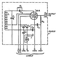
FIG. 1 — THE NEW FREQUENCY METER USES THE ELECTRON-COUPLED CIRCUIT
