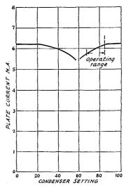
FIG. 2 — SHOWING THE EFFECT OF THE SETTING OF C ON THE OSCILLATOR PLATE CURRENT
