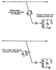
FIG. 3—USE OF WAVE-TRAP TO ELIMINATE HARMONICS
