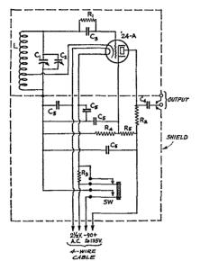
4 - SCHEMATIC DIAGRAM OF W1FL'S VER-SION OF THE E.C. FREQUENCY METER
