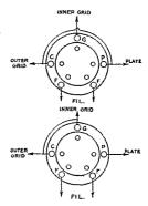
FIG. 3 — SOCKET CONNECTIONS FOR THE 46
