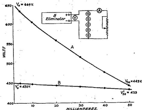
FIG. 2 — SHOWING THE STABILIZING EFFECT OF NEON LAMPS
