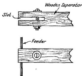
and a hole drilled through at right-angles to the slot about a half-inch in from the end. A machine screw is run through the hole and fastened down with a nut. The wire slips in the slot outside the bolt near the end of the spacer, and when the latter is in the right position the bolt is tightened to hold the wire securely in place. The gripping pressure is greatest near the ends of the spacer. The spacers should be made of hard wood boiled in paraffin.
