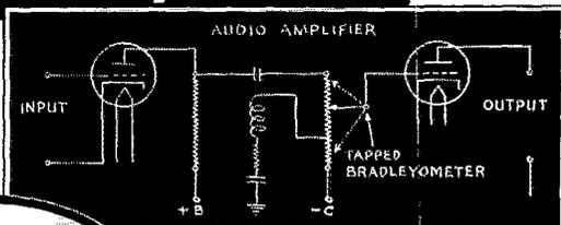
The new Tapped Bradleyometer provides automatic tone correction with volume control. It achieves this result in any one of several audio frequency networks. (See above diagrams.)
