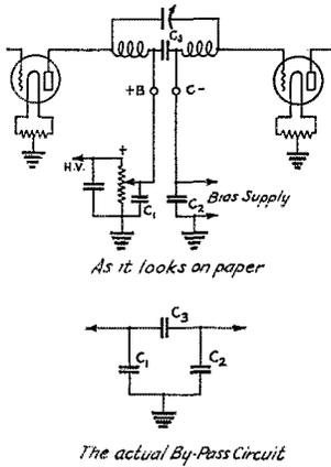
FIG. 4—HOW THE POWER-SUPPLY CONDENSERS CAN AFFECT TUNING WHEN A SERIES-FED CIRCUIT WITH SPLIT INDUCTANCE IS USED
