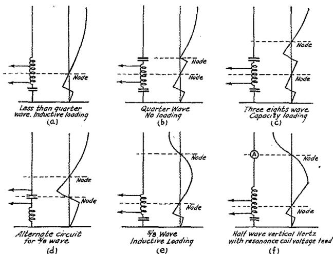
FIG. 5 — THE CIRCUIT OF FIG. 4b APPLIED TO ANTENNAS OF DIFFERENT LENGTHS
