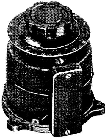
● VARIAC autotransformers are used extensively as voltage controls in amateur stations. Connected in the input side of high-voltage rectifiers, the VARIAC supplies *continuously adjustable* d-c output with a 320 degree rotation of the control knob. VARIACS are ideal for compensating, manually, for low line voltages. The Type 200-CU, illustrated, supplies output voltages in stepless increments to 135 volts when used on a 115-volt line.
