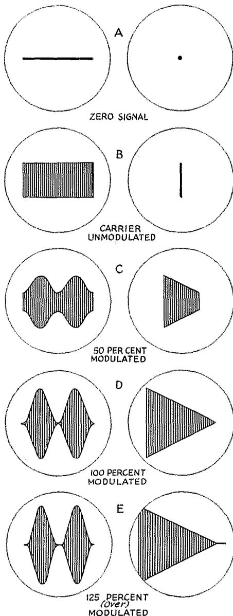
Fig. 1—Wave-envelope (left) and trapezoidal (right) oscilloscope patterns.
