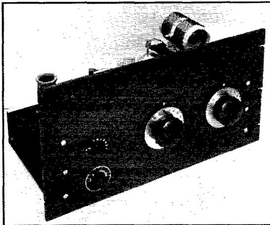
Front panel view showing position of controls. The oscillator plate tuning control is at the left below the crystal-selector switch. The panel is 10½ inches high.
