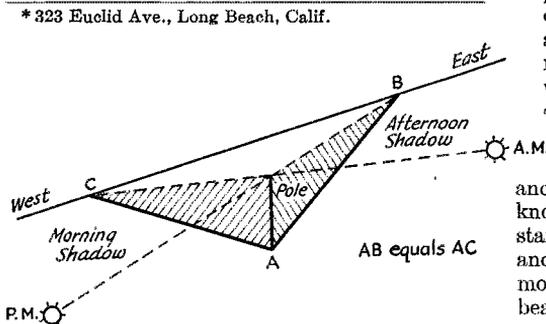
Fig. 1 — The simple method for determining an east-west line from the sun uses a vertical stick or pole on a level surface. A line drawn between the extremities of equal morning and evening shadows gives the desired direction.
