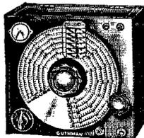
Temperature stabilized. Fundamental range 840-1030 kc, strong harmonics covering 5 thru 160 meters. 7 1/2" dial may be set with extreme accuracy on WWV or 19 broadcast stations. Voltage regulated. Added frequency standard thru built-in 100 kc. oscillator. Detector tube provides audio monitoring and zero beeping; cathode ray tube connected to monitoring detector gives visual deviation. For 105-125 volts, 25-60 cycle. A.C.-D.C. Uses one each 43, 25A7, 6J5, 6E5, VR-105, 55-A.
