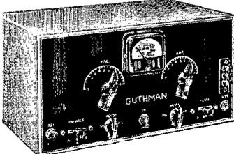
tube transmitter. Switch choice of three frequencies. Selects between standby or power of two ant. matching coils. Modulator 1 power supply, 105-125 volt, 50-60 cy. A.C. output up to 10 watts. Controls: Key-jack, 3 xtal switch, 6-110 volt selector, oscillator tuning, on-off, meter-selector, amp. tuning, out-coupling, standby, mike jack. Panel cut for meter. 6 volt socket on chassis rear. Uses 4 7C7, 83V, two 7C5s. Ship. weight, 16 lbs. Size 12 1/2"x7"x7 1/2".
