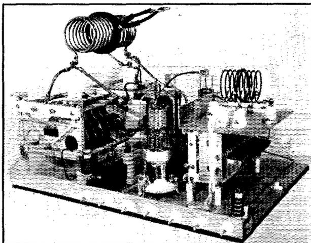
Each unit is built on a 16-gauge cadmium-plated body steel chassis which is supported by a piece of  $\frac{5}{8}$ " three-ply. All parts and wiring are readily accessible for modifications or trouble-shooting.
