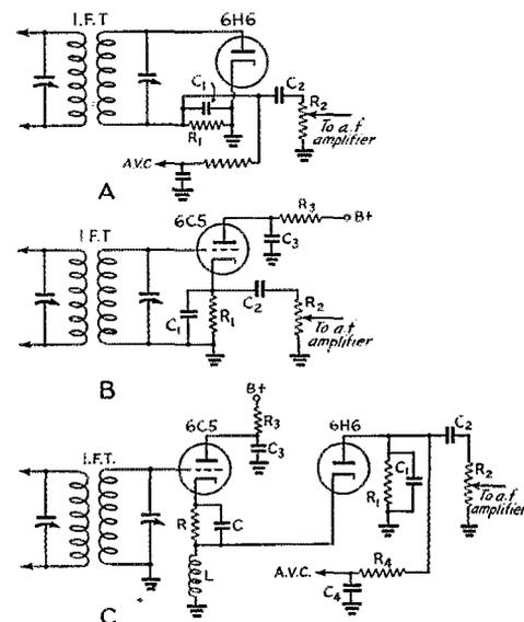
Fig. 1 — The second detector circuits under discussion. The conventional diode rectifier is shown at A, while B shows the "infinite impedance" type of detector. C is the diagram of a cathode-coupled i.f. amplifier.
