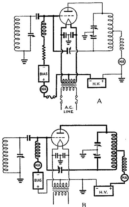
Fig. 3—Grounding the positive high-voltage terminal instead of the negative terminal places most of the exposed portions of the circuit at ground potential, while less exposed portions are at high d.c. potential above ground. Heavy lines indicate high potential points of the usual arrangement at B and the grounded-positive arrangement at A. See text for precautions in using.
