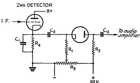
Fig. 1—The series limiter circuit, with infinite-impedance detector.
