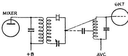
Fig. 4—Broadening crystal filter for 'phone work. The coupling connection is shifted from the center tap to the grid.
