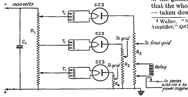
Fig. 2 — The bias supply uses separate rectifier tubes to keep the bias from "backing up."
