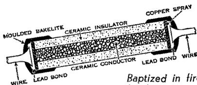
*Baptized in fire at 2500 degrees — hard as stone — center ceramic core and ceramic jacket fired together to form a single shock-proof unit. Pure copper applied by Schoop metal spray process forms intimate end contact to conducting area.*
