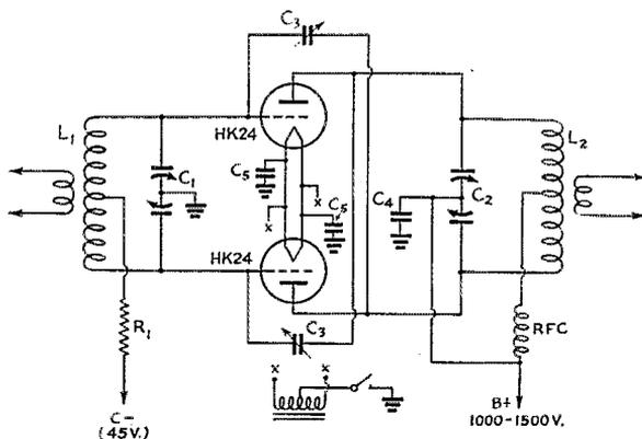
Fig. 1 — Circuit diagram of the HK24 amplifier.
