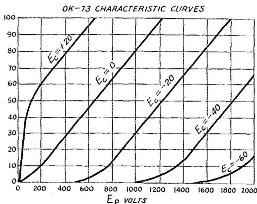
Fig. 2 — The characteristic curves of the OK-73.
