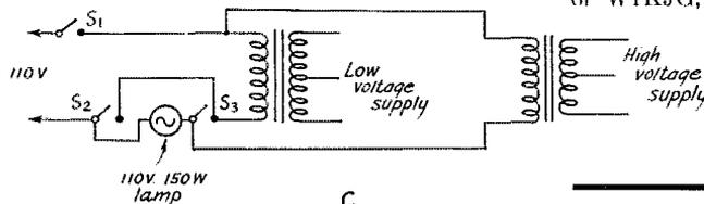
Fig. 5 Power-supply kinks. A — Operating 866 Jr's from 5v., 3a. transformer. B — Changing voltage by changing rectifier-tube sockets with dual-voltage secondary transformer. C — Plate-voltage control system.
