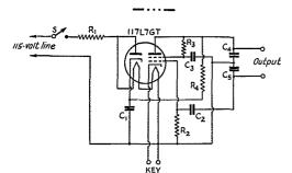
Fig. 2 — Circuit diagram of simple code-practice oscillator.
