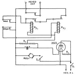
Fig. 2 — Circuit diagram of the code reproducer. - 40-µfd. electrolytic, 150 volts. (Smaller capacities will do.)
