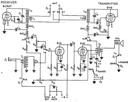
Fig. 1 — Circuit diagram of the 21/2-meter transmitter-receiver.
