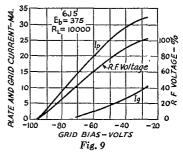
value of grid current for a given bias voltage, on the input, linearity and grid bias. In each of these cases the values at minimum grid bias (approximately —25 volts) can be taken as representing conditions existing at the modulation peak. For carrier conditions the bias would be set midway
