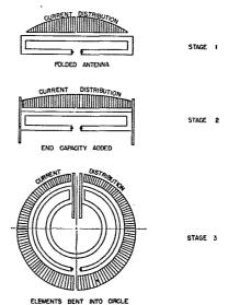
Fig. 5 — Evolution of the circular antenna from a folded dipole.
