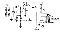
Fig. 4 — Automatic air-raid alarm device operating from any b.c. receiver.
