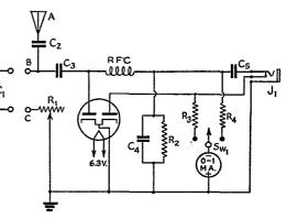
Fig. 3 — Circuit diagram of the modulation indicator.
