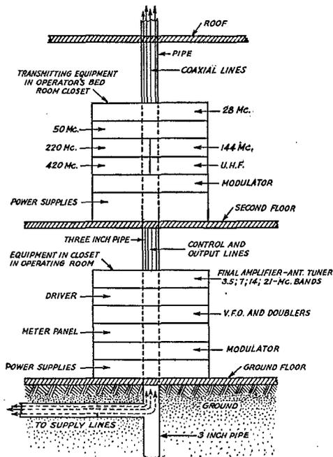
Fig. 2—Coordinated installation of transmitting equipment in closets on two levels. Supply lines are brought in underground. The 3-inch pipe extends down into a well or other suitable grounding arrangement. This pipe also extends upward through the roof. Equipment control and feed lines are run through the pipe.
