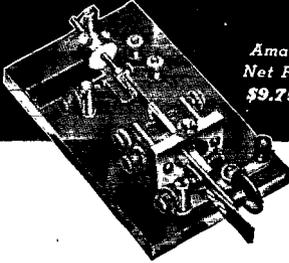
One of the finest commercial or amateur bugs available. Chrome finished base and superstructure. Springs made of selected blue spring steel for uniform performance in all keys. Nine points of adjustment to suit the most critical touch. Fully adjustable. Silver contacts 3/16" diameter.
