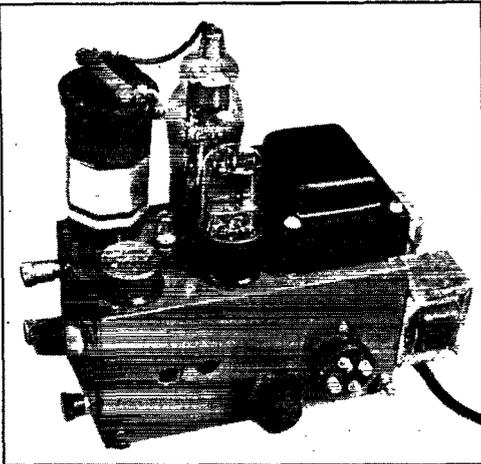
Top view of the "Tom Thumb" transmitter-receiver. The 79 tube is in the rear and the 6X5GT in front. Along the front edge are the screwdriver-tuning openings, the regeneration control knob, and the audio-output socket for making connections to an external audio amplifier.
