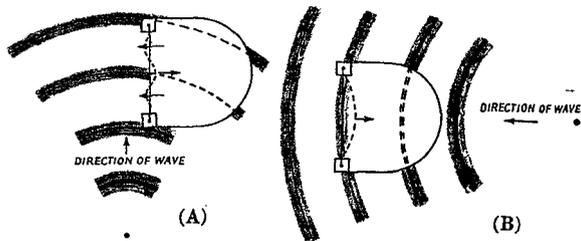
Fig. 4—A—Diaphragm movement under wave approaching at right angles to plane of diaphragm. B—Wave approaching from the rear of the microphone.
