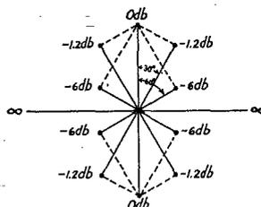
Fig. 8 — Directional characteristics of a velocity microphone.
