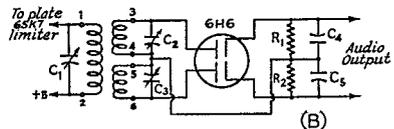
trimmer condensers of suitable capacity to operate on the frequency desired. In my receiver, I used 360- $\mu$ fd. trimmers to cover the range from 69 to 130 kc. The transformer should be mounted adjacent to the trimmers. I cut holes through the chassis to permit adjustment of the variable trimmers. — *G. A. Lyerly, 403 65th St., N. E., Washington 19, D. C.*
