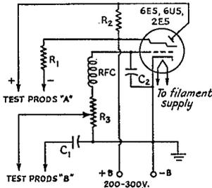
Fig. 1 — Condenser checker and output meter using a "magic eye" tube.  $R_1$  is adjusted until shorted prods *A* will close shadow.  $R_1$  is 3300 ohms in W7FGB's tester.  $R_3$  is a 100,000-ohm potentiometer.  $C_1$  and  $C_2$  are 0.01- $\mu$ fd. 600-volt paper. The r.f. choke was salvaged from an old h.c. receiver.
