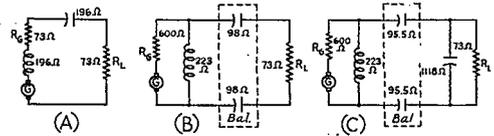
Fig. 3—Development of 7-Mc. network. (A)—Electrical equivalent series circuit. (B)—600-ohm source matched to 73-ohm load. (C)—Same as (B) but corrected after 14 Mc. has been added.
