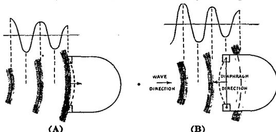
Fig. 3—A—Microphone diaphragm under pressure of sound wave. B—Diaphragm position under a "rarity" or absence of pressure. The shaded dashed line represents the part of the wave which is passing the microphone indicating that the wave direction and direction of diaphragm movement are opposite.
