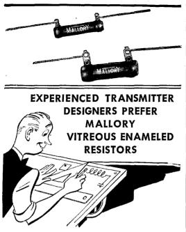
Engineering advancements born of wartime experience make Mallory vitreous enameled resistors better than ever. An improved enamel provides greater protection, keeps out moisture, minimizes warping, stretching and shifting of the wire during manufacture. New processing technique banishes "hidden corrosion," the thief that robs life, whether the resistor be in service or out.
