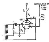
Fig. 1 -- Circuit modifications required for the addition of a noise limiter to the Sky Buddy receiver. C1 - 100-µµfd. mica.
