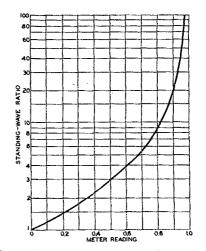
Fig. 2 — Standing-wave ratio plotted against meter reading of the Micromatch. The meter has a full-scale reading of 1.0.
