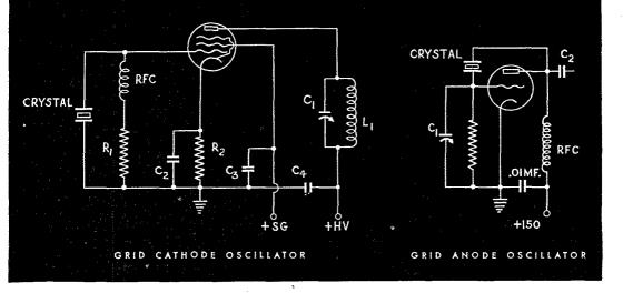
Way back in the prewar era Bliley pioneered "harmonic" crystals for amateur frequencies in the 10 and 20-meter bands. Nowadays we know that such crystals should be correctly termed "overtone" oscillators because the crystal does not oscillate at the exact mathematical harmonic of its fundamental frequency. The present Bliley AX2 unit for 20-meter operation contains an overtone crystal designed to oscillate at approximately three times the fundamental mode.
