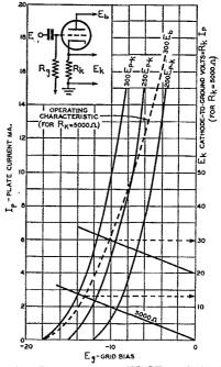
Fig. 3 — Curves used in 6SN7GT analysis. Gridcathode voltage is shown across bottom. When upper 5000-ohm line is extended, it crosses the  $E_g$  axis at +20 volts.
