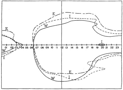
Fig. 2 — The 30-megacycle F2-4000 m.u.f. contour lines traced from the CRPL prediction charts for April, 1947. The contours for the three zones are superimposed on the same chart so that 10-meter predictions the world over can be observed at a glance.
