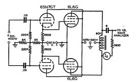
Fig. 1 — Circuit used for measuring power output and distortion in the cathode-coupled Class AB<sub>2</sub> modulator.
