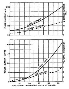
Fig. 2 — Curves showing power output and distortion from a 6L6 Class AB<sub>2</sub> amplifier with cathode-coupled driver.
