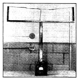
Twin-Lead folded-dipole receiving antenna The mounted on a wooden frame above the indicating meter.
