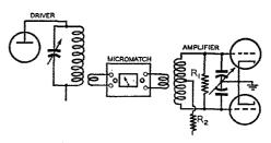
Fig. 8 — Interstage link coupling can be properly adjusted by means of the Micromatch. Since the gridcircuit loading depends upon the grid current of the tubes and the value of grid leak,  $R_2$ , adjustment should be made under actual operating conditions. In some cases it is necessary to load the circuit with an additional resistor,  $R_1$ , to obtain the proper match for the link line.
