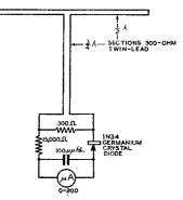
Fig. 1 - Circuit diagram of field-strength indicating receiver using crystal-diode rectifier.
