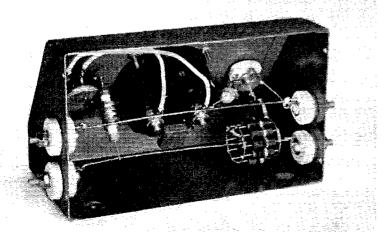
A rear view of the Micromatch with its Masonite back cover removed. Notice the construction of the composite 1-ohm resistor and how the other components are arranged to have as little coupling as possible to the No. 14 wire main lines.
