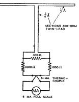
Fig. 3 - Circuit diagram of receiver using vacuum thermocouple.
