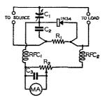
Fig. 5 - Circuit diagram of the Micromatch standing-wave indicator.
