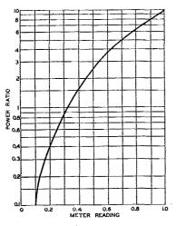
Fig. 3 -- Calibration curve of the Micromatch ind cator used as a wattmeter. One actual point must be found by comparison with a lamp or other known r.f. load, after which the above scale can be fitted to the meter.
