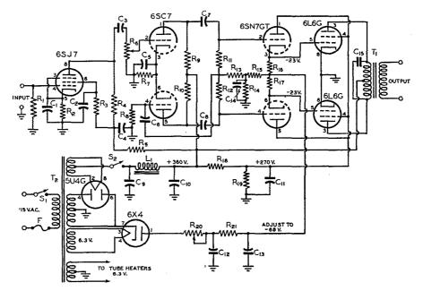
Fig. 4 — Circuit diagram of the 40-watt modulator using a cathode-coupled driver.
