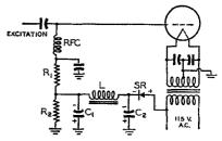
Fig. 3 — Bias system for an 813 amplifier using one of the new midget selenium rectifiers.
