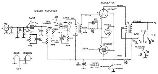
Fig. 1 — Circuit diagram of the modulator unit. All capacitors are in  $\mu$ f. except  $C_1$ . Capacitors marked with polarity are electrolytic; others may be mica, ceramic or paper. All resistors are  $\frac{1}{2}$  watt unless specified.
