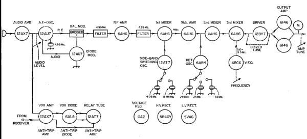
Fig. 1 — Block diagram of the HT-32 transmitter/exciter. The s.s.b. signal is generated through two crystal filters at 4.95 Me.; then heterodyned several times for side-band selection and to permit use of a 5.0-5.5-Me. v.f.o.
