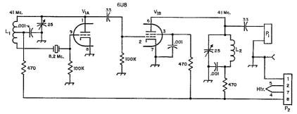
Fig. 4 — Circuit of the 41-Mc. injection unit used with the 10B exciter to obtain 50-Mc. output.  $L_1$ —10 turns No. 24, 32 t.p.i.,  $\frac{1}{2}$ -inch diameter, tapped at 3 turns from crystal end.  $P_1$ —300-ohm line plug (Millen 37412).  $P_2$ —8-pin plug. (Fits octal socket on back of 10B.)  $P_2$ —8-pin plug. (Fits octal socket on back of 10B.)
