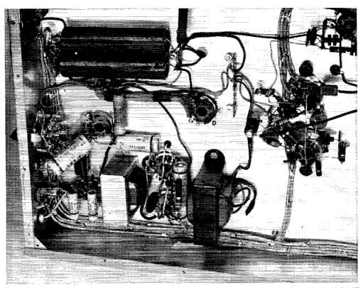
Bottom view showing audio components under the chassis. T1 is to the left; T2 to the right. The two 6BQ6GT sockets are between the transformers. The two large tubular capacitors above are in the original power-supply filter.
