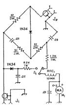
Fig. 2 — Circuit of the s.w.r. bridge. All resistors are composition. Capacitors are ceramic and values are in  $\mu$ f. J<sub>1</sub>, J<sub>2</sub> — Coaxial receptacle, SO-239. M<sub>1</sub> — 0-2 d.c. milliammeter.
