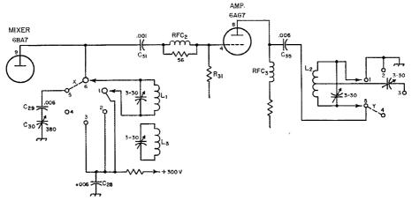
Fig. 3 — Plug-in coil circuits of the 10B as they appear after the conversion process. Jumpers X and Y, shown in dashed lines, are installed in the 10B coils for lower frequencies, and are omitted from the 50-Mc. coils. Parts numbered, but not appearing below, are original components in the exciter.
