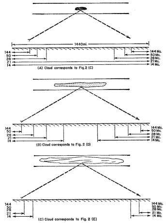
Fig. 5 — How the area coverage varies with time, for different frequencies.
