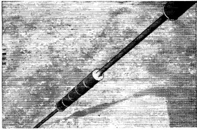
by melting the poly slightly with an iron so that it makes a tight fit.
