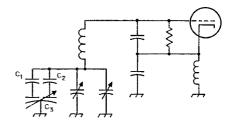
differential capacitor, as shown in Fig. 3. The oscillator is tested by recording the frequency change with temperature. The direction of the drift then indicates which way the differential capacitor must be moved to minimize the deviation.
