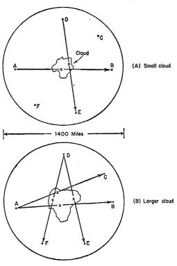
Fig. 3 — Effect of cloud size on radio area coverage. The ion density is assumed constant in both cases shown.
