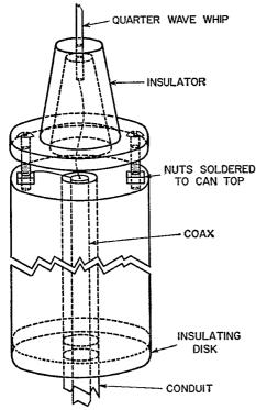
Fig. 1 — Details of the top section of the juice-can coaxial vertical antenna.
