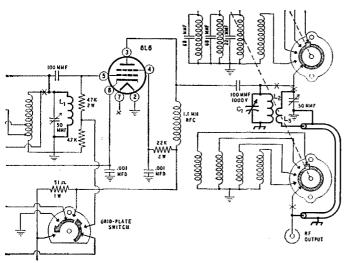
Fig. 1—Changes in the AT-1 required to operate it on 50 Mc. Points where the circuits are broken are indicated by "X." Band switch is left in the 80-meter position
