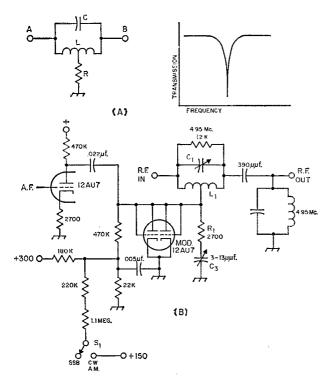
Fig. 2 — The bridged- $\Gamma$  circuit is shown at  $\Lambda$ , together with the transmission properties between points  $\Lambda$  and B. When the value of R is equal to  $\frac{1}{4}$  the resonant impedance of LC, the notch is a maximum, at the frequency determined by LC. Increasing or decreasing the resistance of R reduces the depth of the rejection notch. When used as a balanced modulator, LC is tuned to the (suppressed) carrier frequency and R is varied at the modulation frequency.
