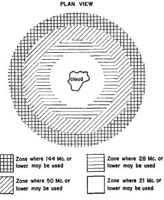
Fig. 4—Typical area coverage of different radio frequencies reflected from a given ion cloud.
