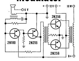
Now radio amateurs and experimenters can build a mobile transistorized modulator. Simple circuit features: pre-driver, driver, and final amplifier with low-cost CBS 2N255 and 2N256 power transistors ... 10 watts output (modulates 2E26) ... instantheating . . . low drain . . . for use with transmitter or sound system.
