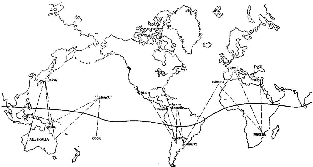
Fig. 1—Dashed lines illustrate some of the 50-Mc. transequatorial scatter paths worked by PRP observers during the IGY. The solid, wavy line represents the magnetic equator where the earth's magnetic field is parallel to its surface. Note how the *TE* is roughly symmetrical to this equator.
