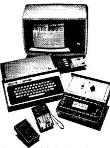
Your training includes the TRS-80 color computer, the NRI Discovery Lab, interfacing breadboard, digital multimeter, frequency counter, computer-assisted training programs, audio instruction tape, and 46 profusely illustrated lessons.
