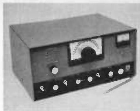
The receiver is built in a homemade aluminum cabinet. A two-tone gray and flat-black paint job has been applied. Black Dymo tape labels are used for identifying the controls in the black area, and gray labels are affixed to the gray portion of the front panel. A cut-down Jackson Brothers vernier dial mechanism (two-speed) is used for frequency readout.
