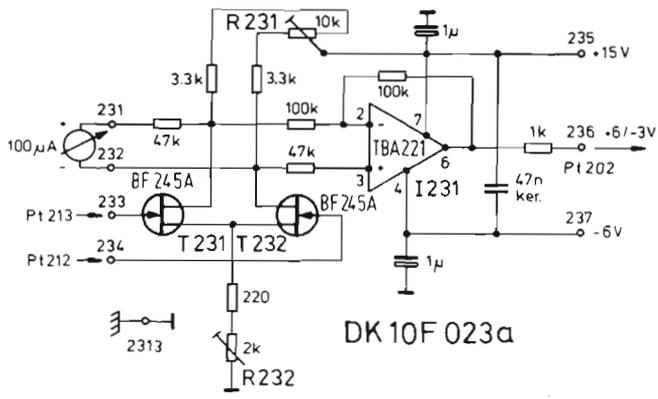
Fig.20: Circuit diagram of the AGC and S meter amplifier
