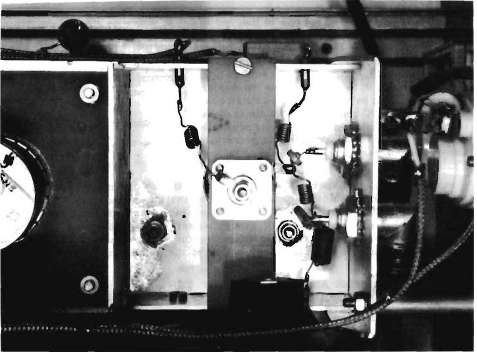
Fig.15: Close-up view of the cathode side of the mixer stage
