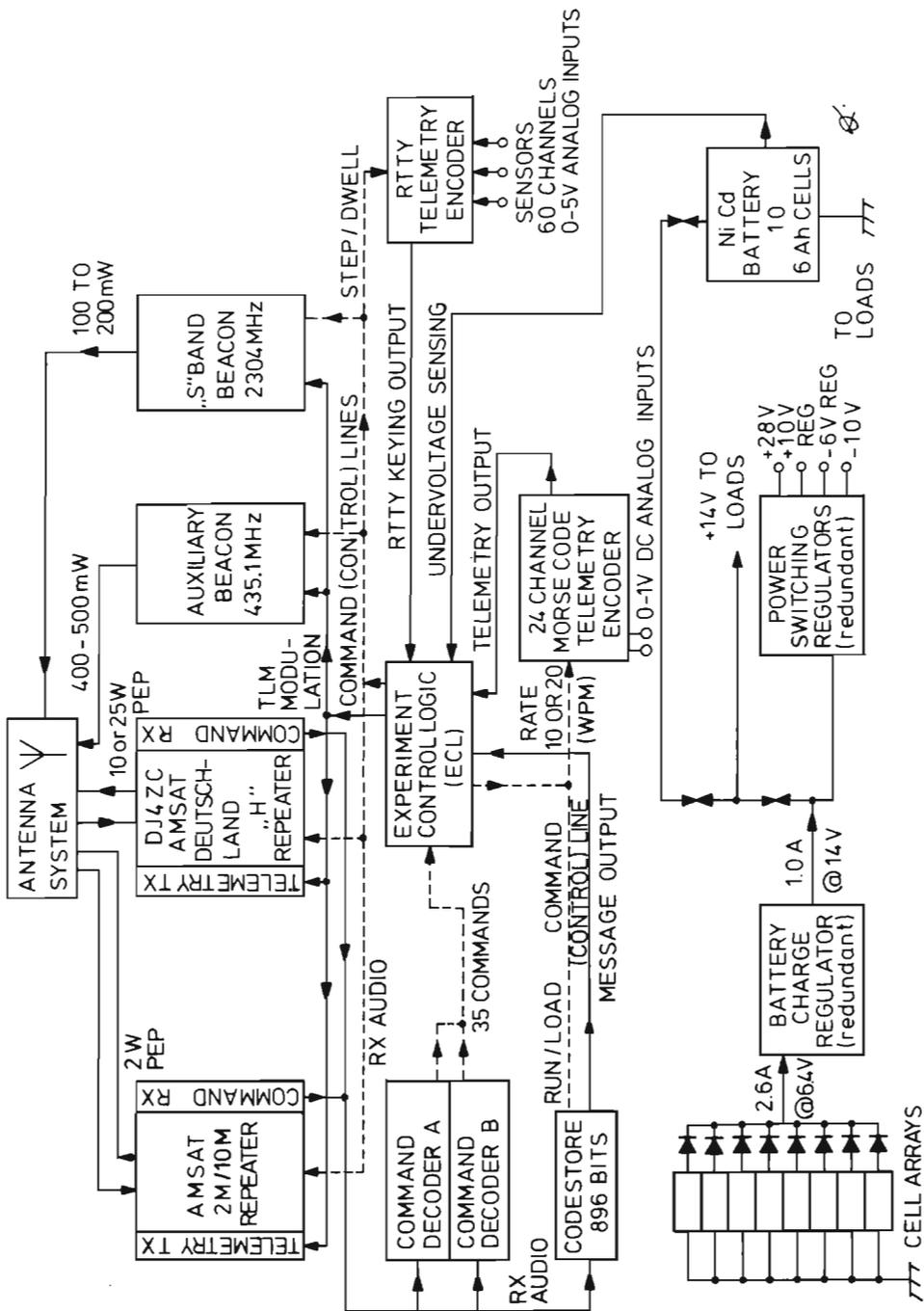
Fig.1: Block diagram of the electronic circuits in OSCAR 7
