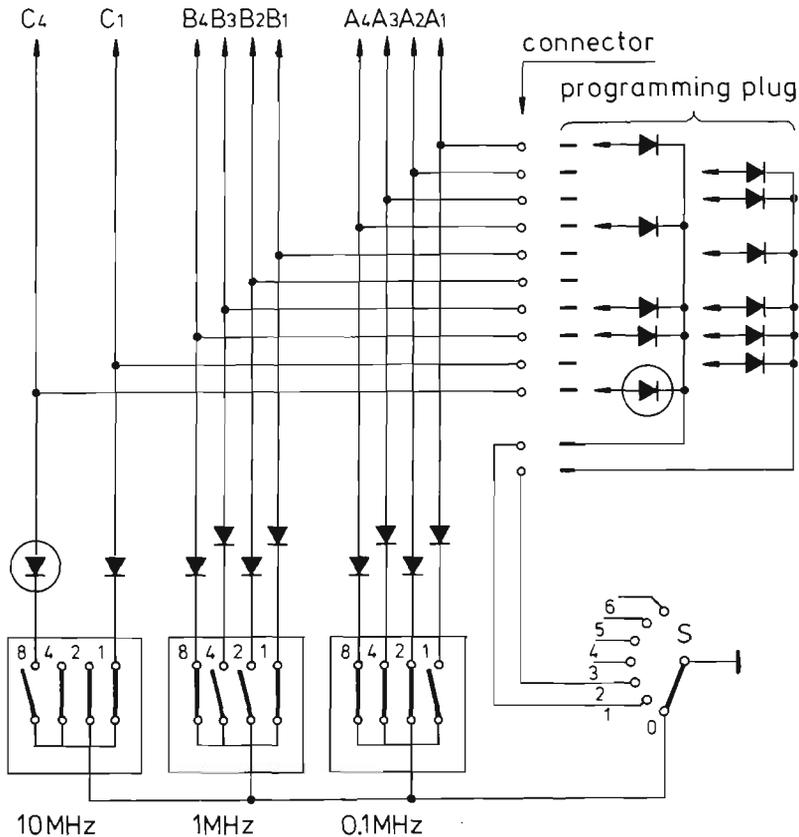
Fig.17: Channel selection and programming using inverted BCD-coded switches
