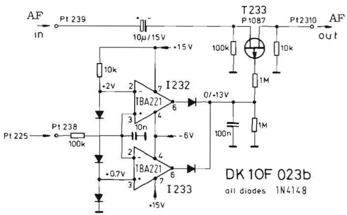
Fig.21: Circuit diagram of the squelch circuit
