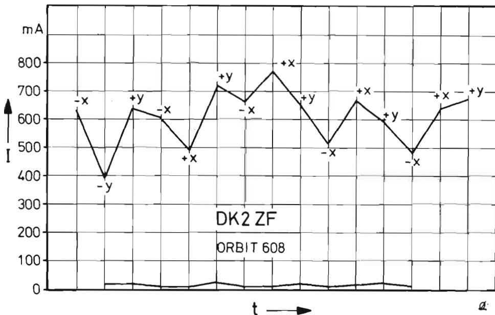
Fig.7: Maximum of the solar cell currents indicating a regular rotation of the satellite
