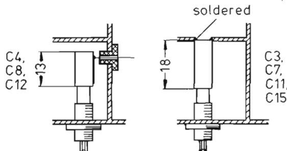
Fig.14: Installation of the tubular trimmers
