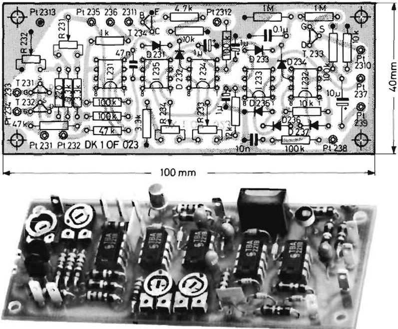
Fig.23: Component locations and prototype of the AGC-amplifier, squelch, and tuning indicator
