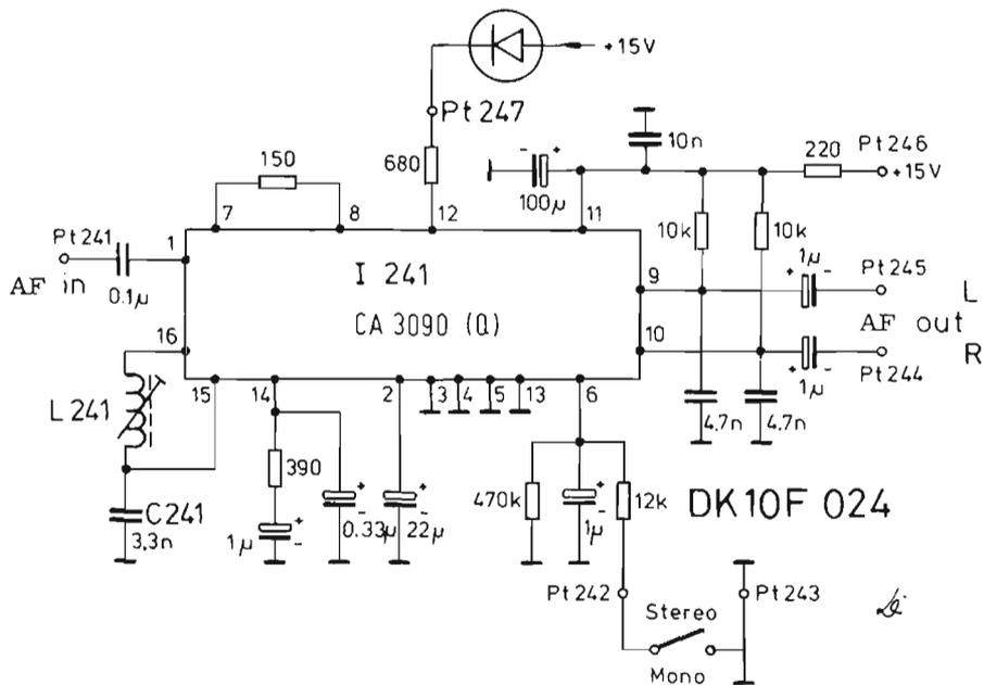
Fig.24: Circuit diagram of the stereo decoder
