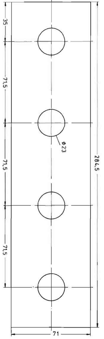
Fig.4 : Dimensions of the grid plate
