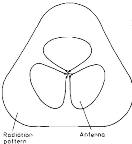
Fig.8: Horizontal radiation pattern of a Big Wheel antenna
