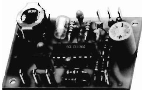
Fig.26: Prototype of the stereo decoder
