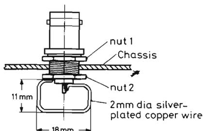
It has been found that there is some danger of the solder melting later. It is not possible to hard solder the coupling link to the connector, since this would damage the teflon dielectric. It is therefore necessary for both ends of the coupling link to be provided with enough solder so that they are completely covered. It should then be possible to solder the anode chamber of the output stage without unsoldering the coupling link at the same time.
