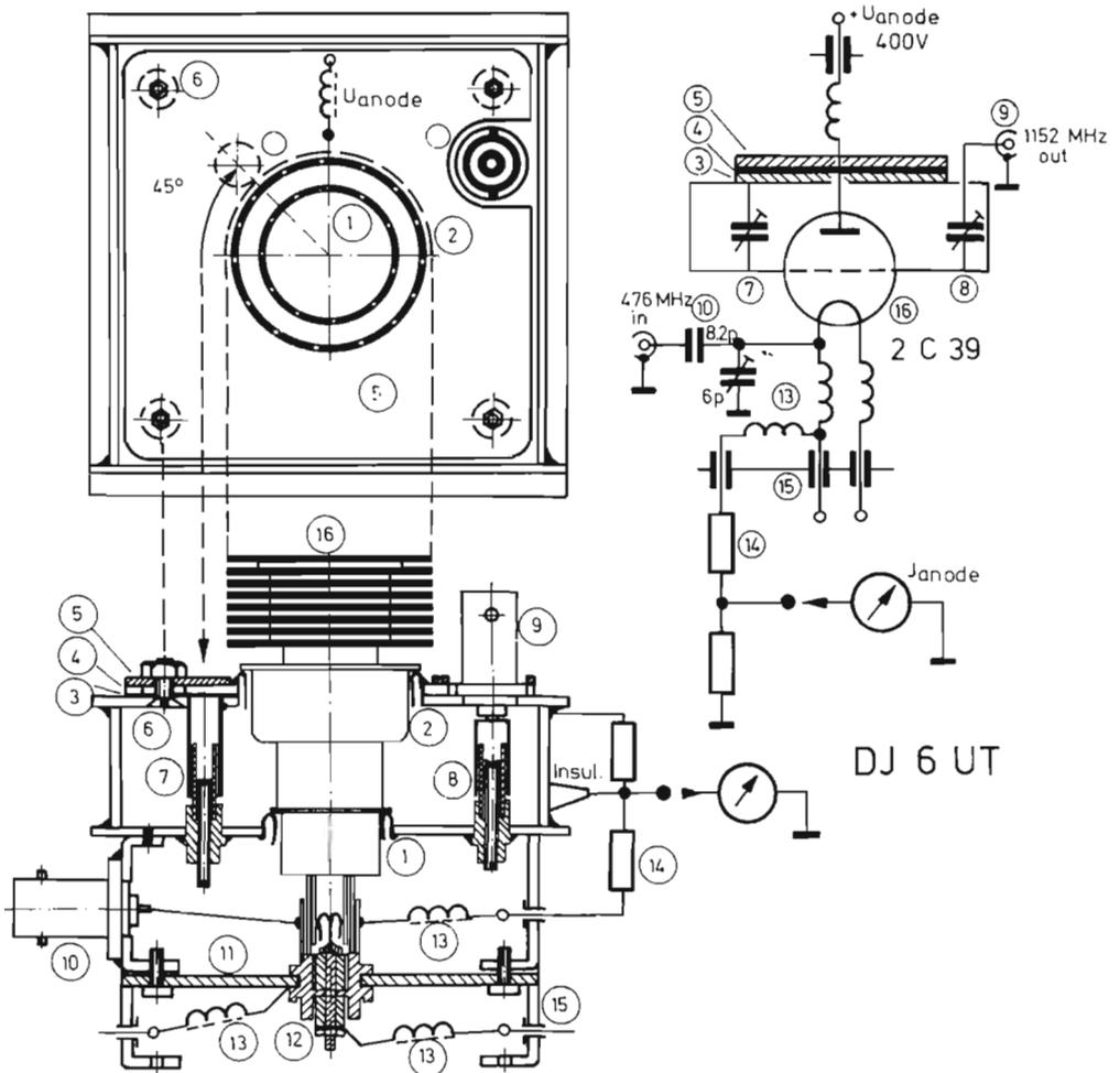
Fig.18: Last frequency doubler 476/1152 MHz of the local oscillator
