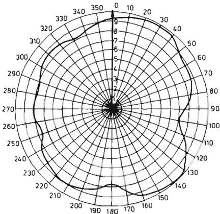
Fig.5: Horizontal radiation pattern of a Halo antenna
