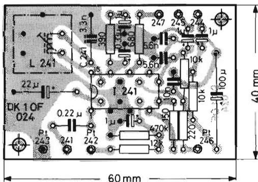
Fig.25: Component locations on PC-board DK 1 OF 024
