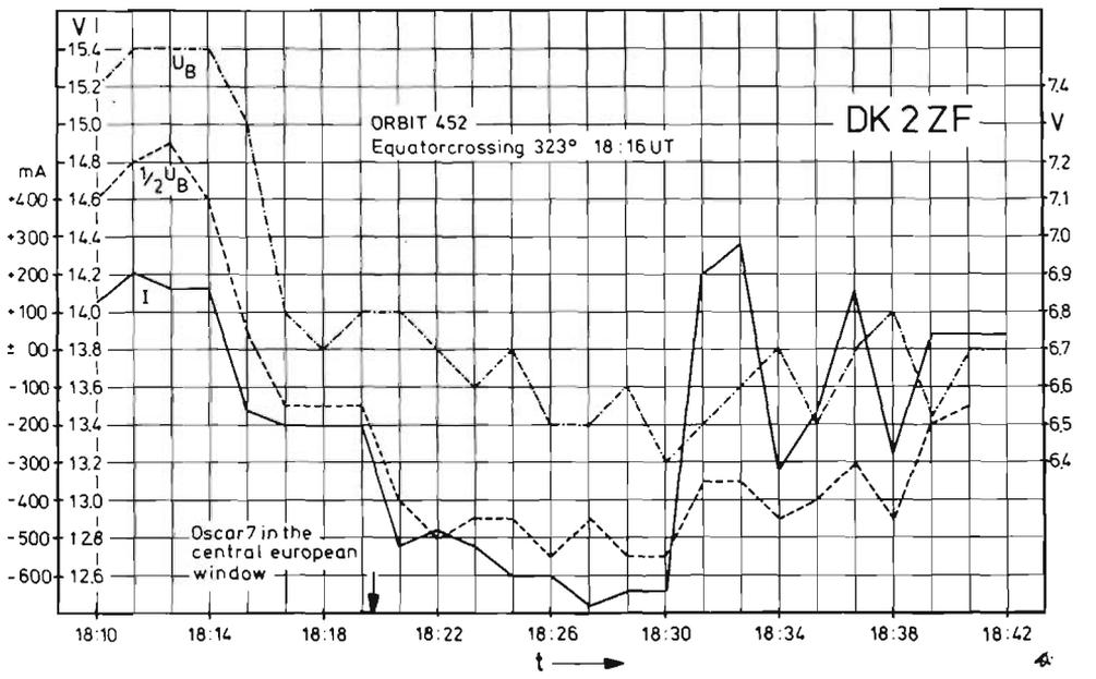
Fig.5: Three further telemetry values during orbit 452
