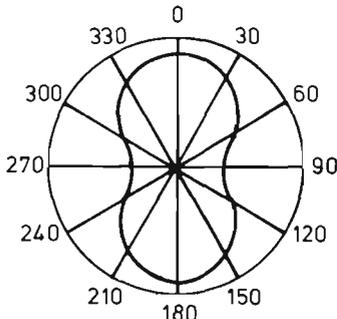
Fig.7: Horizontal radiation pattern of a canted dipole
