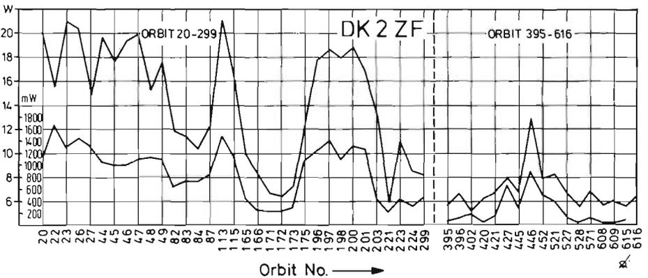
Fig.3: Solar cell power and RF-output power of the 10 m transmitter
