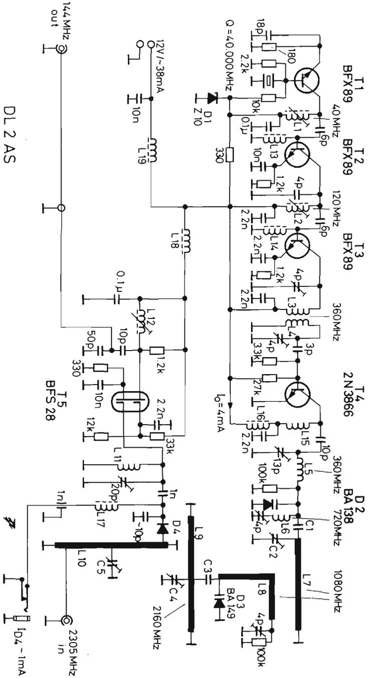
Fig.1: Circuit diagram of the 13 cm receive converter
