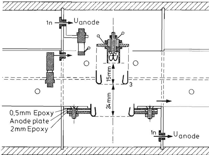
Fig.13: Tube contacts, installation of the trimmers and feedthroughs
