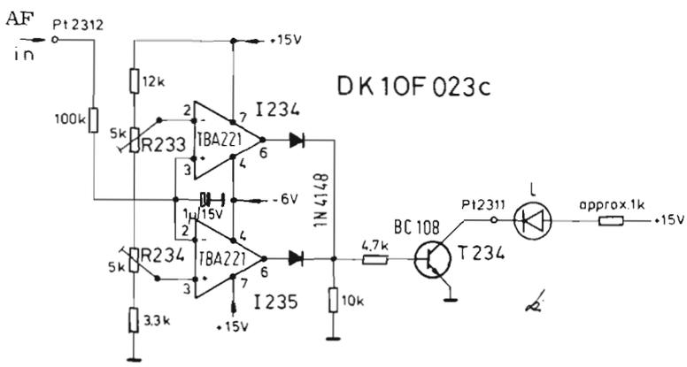
Fig.22: Circuit diagram of the tuning indicator
