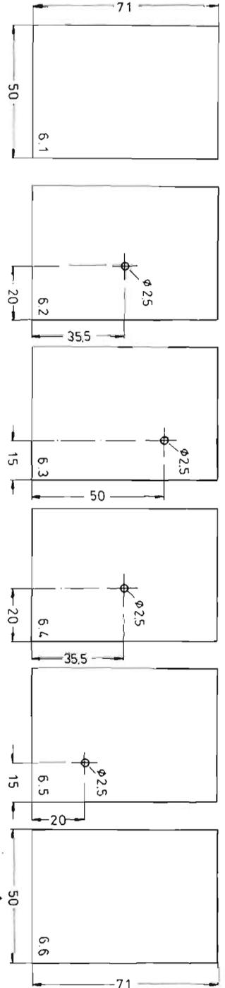
Fig. 6 : The six intermediate panels
