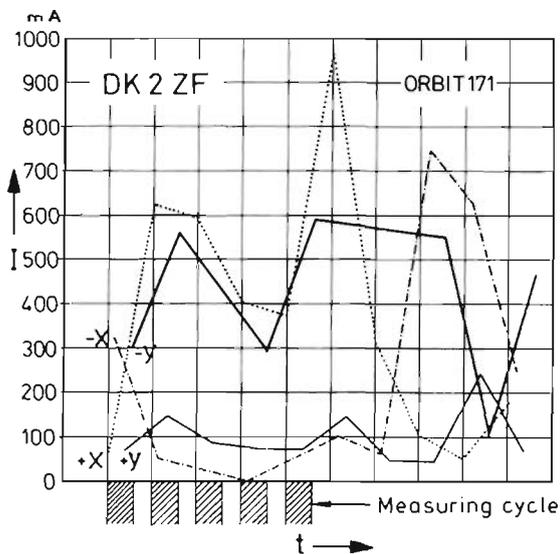
Fig.8: Solar cell current during orbit 171
