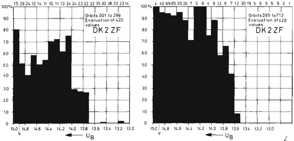
Fig.2: Dependence of the indication in channel 1 A from the battery voltage
