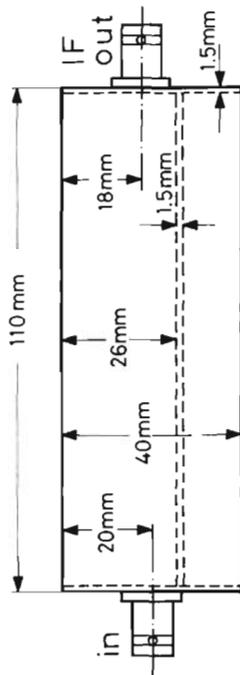
Fig. 4: Dimensions of the case
