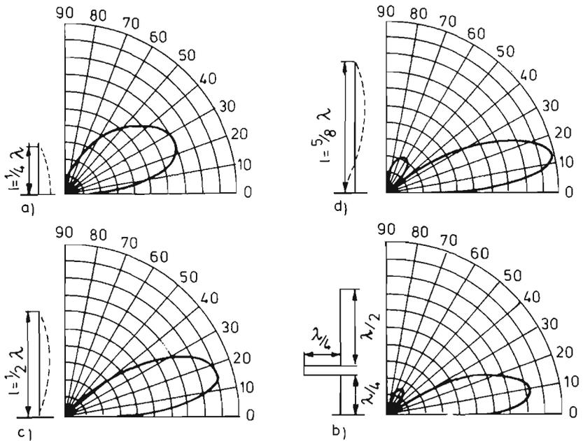
Fig.1-4: Vertical radiation patterns of vertically polarized mobile antennas
