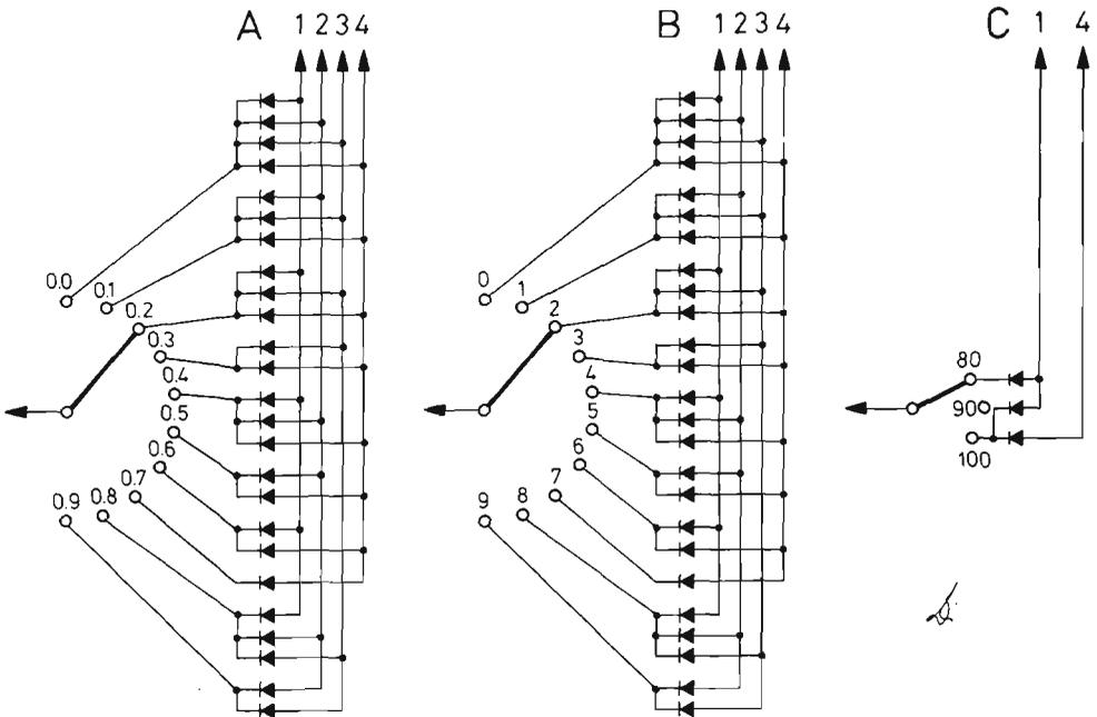
Fig.18: Using a multi-position switch for channel selection
