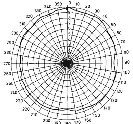
Fig.6: Horizontal radiation pattern of a crossed dipole
