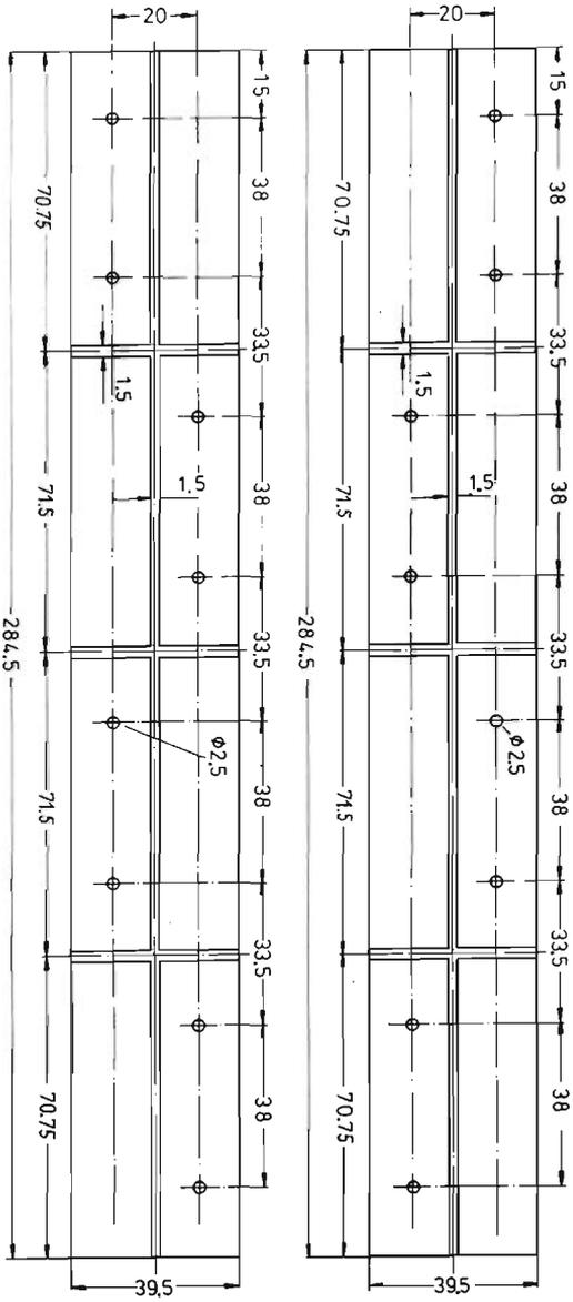
Fig.5 : Dimensions of the two side panels
