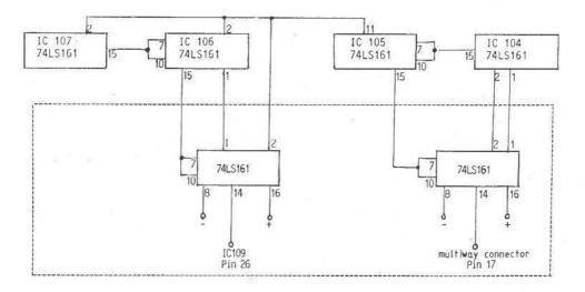
The part of the circuit within the dotted rectangle is added to the original circuit Fig. 1: Colour test-image extension DD 1 PE
