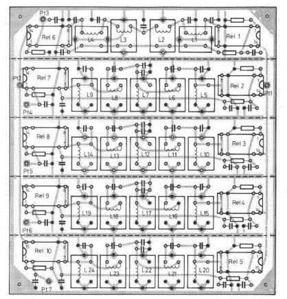
Fig. 11: Filter card component layout
