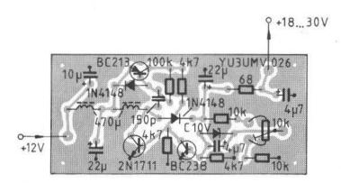
Fig. 27: Component plan of PCB YU 3 UMV 026 (regulated DC-voltage converter)
