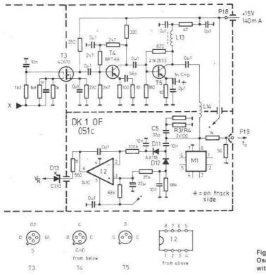
Fig. 6: Oscillator-amplifier with level control
