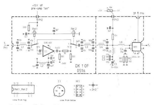
Fig. 2: RF pre-amplifier, IF trap and mixer
