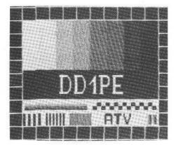
Fig. 2: Original test-image with 256 x 128 pixels following the generator extension
