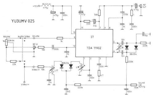
Fig. 19: Circuit diagram of the sound demodulator YU 3 UMV 025
