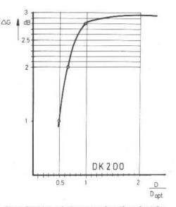
Fig. 3: Stacking gain departures from the gain at the optimum distance. Use this curve to arrive at the shortfall in gain when the optimum spacings cannot be achieved in practice.
