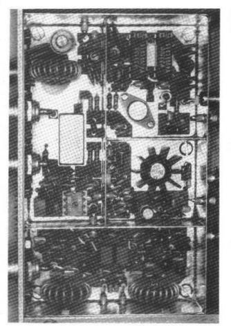
Fig. 8: Mixer module prototype
