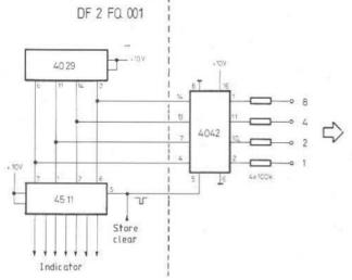
the pull-down resistors at the comparator inputs, a voltage divider which delivers the correct H level of 15 V. The module of DF 2 FQ has a four digit readout which, in general, is sufficient for amateur radio equipments having a resolution of 100 Hz at high frequency and 1 kHz at VHF / UHF. The inputs of both the high value digits remain unswitched.
