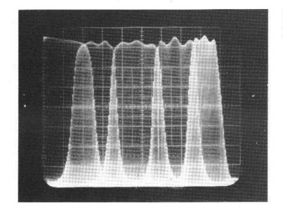
Fig. 10: Band-pass characteristics of the five input filters
