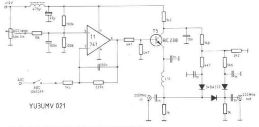
Fig. 15: Circuit diagram of the AGC attenuator YU 3 UMV 021
