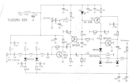
Fig. 14: Circuit diagram of the second tunable down-converter 800 to 1700 MHz/200 MHz (YU 3 UMV 020)
