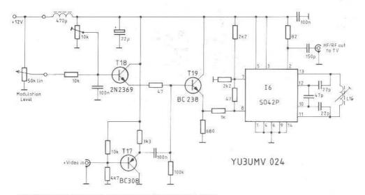
Fig. 18: Circuit diagram of the AM video modulator YU 3 UMV 024
