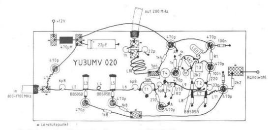
Fig. 21: Construction of the second tunable down-converter YU 3 UMV 020
