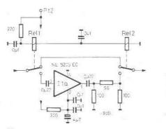
Fig. 3: Low-cost version of RF pre-amplifier
