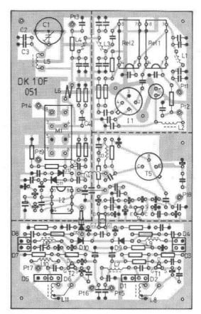
Fig. 7: Mixer card component layout
