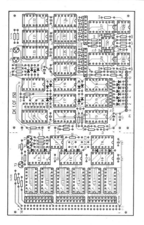
Fig. 40: Component layout plan of PCB DK 1 OF 050
