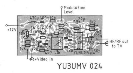
Fig. 25: Component plan of PCB YU 3 UMV 024 (AM video modulator)
