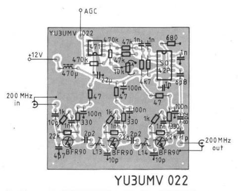
Fig. 23: Component plan of PCB YU 3 UMV 022 (second IF amplifier and AGC detector)
