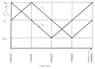
Fig.35: Control voltages V<sub>1</sub> and V<sub>2</sub> dependent upon input data
