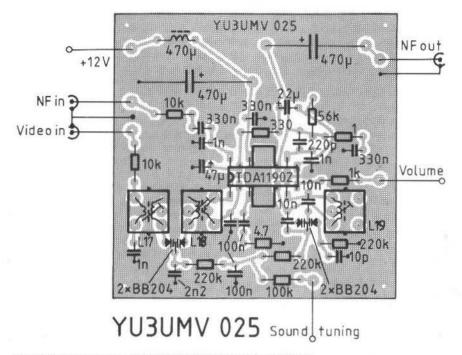
Fig. 26: Component plan of PCB YU 3 UMV 025 (sound demodulator)
