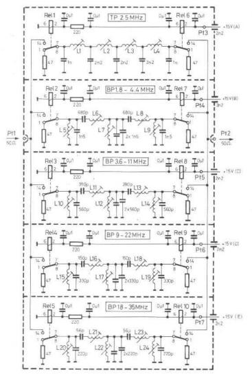
Fig. 9: RF input filter unit circuit diagram
