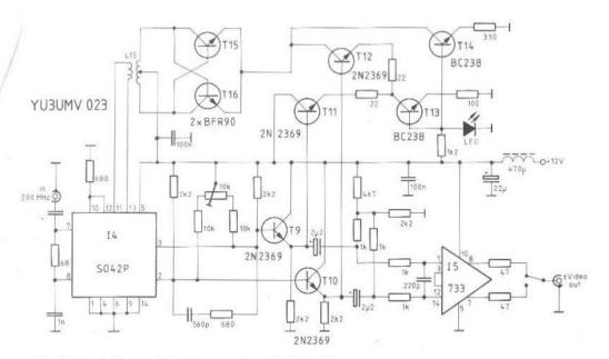
Fig. 17: Circuit diagram of the PLL demodulator YU 3 UMV 023
