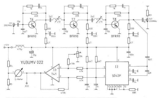
Fig. 16: Circuit diagram of the second IF amplifier and AGC detector YU 3 UMV 022
