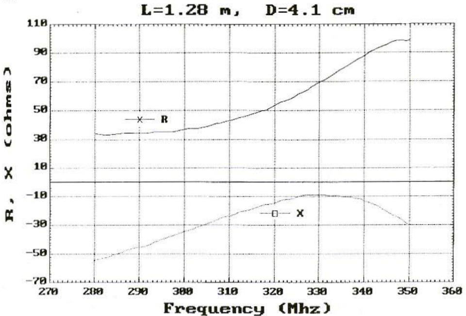
Fig.6: Measured XDZ Input Impedance
