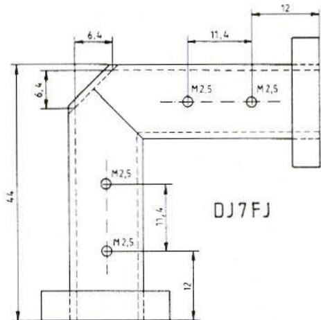
**Fig.4: Construction Dimensions for a "Compensated Bend" made from Waveguide Material**
