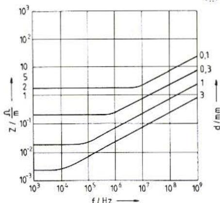
Fig.2: Skin Effect for Round Copper Conductors
