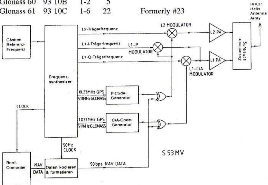
Fig.6: Block Diagram of GPS and GLONASS Satellites
