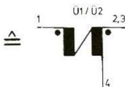
Wire the two-part windings together, observing the correct polarity
