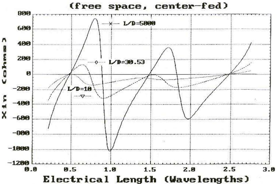
Fig.5: Dipole Input Reactance
