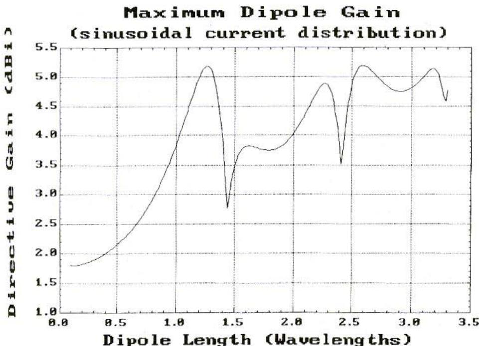
Fig.2: Directivity of a Free-Space Centre-Fed Dipole vs Electrical Length
