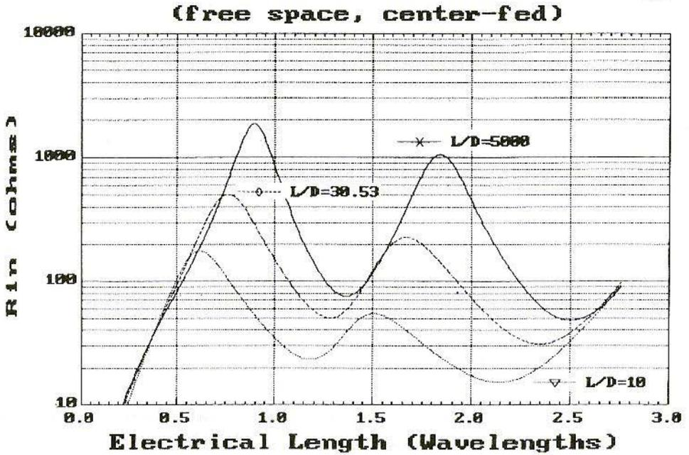
Fig.4: Dipole Input Resistance
