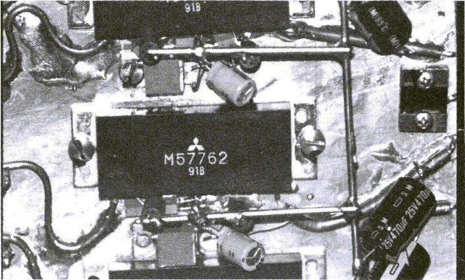
The coax stubs are soldered directly to the copper plate, which makes a very stable assembly. This is essential in this kind of circuit.
