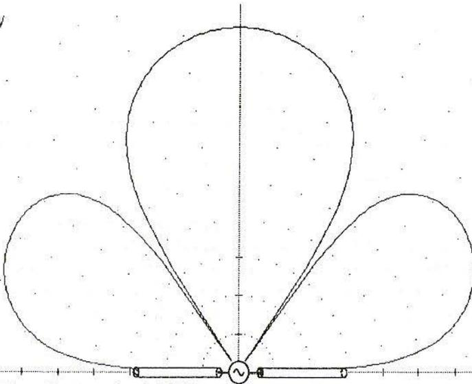
Fig.3: Pattern Factor of a 1.27 Wave Dipole
