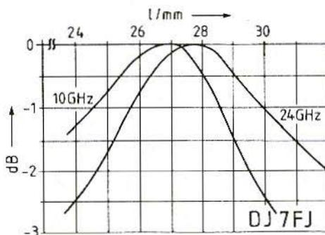
Fig.3: Optimising Gain by changing Radiator Position
