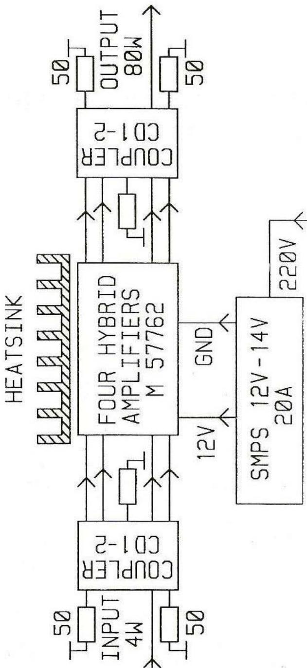
Fig.1: Circuit Connections
