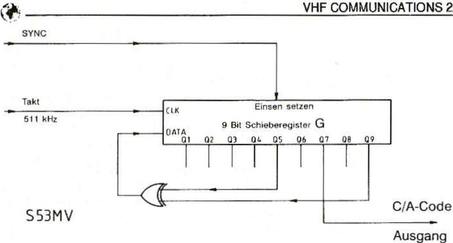
Fig.10: The GLONASS C/A Code Generator
