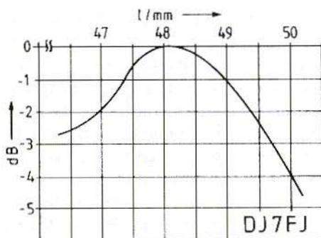
Fig.2: Radiator Length plotted against Gain at 24 GHz
