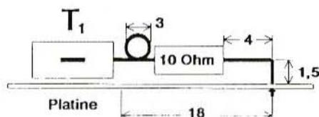
Fig.8: Dimensions of the Coupler
