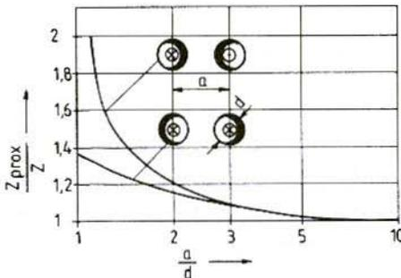
Fig.3: Proximity Effect for Round Conductors
