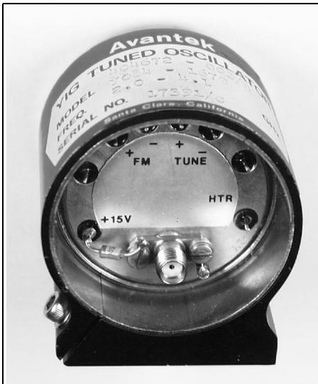
**Fig 27: YIG oscillator used in the prototype.**
