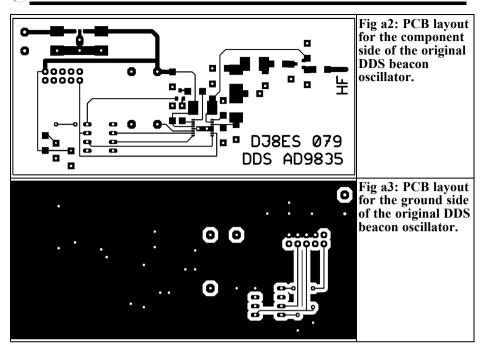
ATTiny45 (IC1) microcontroller from Atmel. This also produces of telegraph signals. The output level of DDS is adjustable on pin 1 (FSAdj) using the current through R2. A switching FET T1 (2N7002) is used for the CW keying. The modulation depth is approximately 40dB. This is sufficient in the low power shortwave use.
