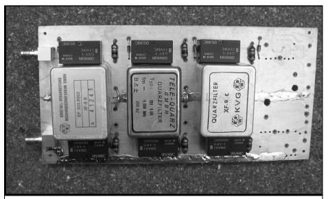
Fig 6: Photograph of the completed prototype showing the XF9B SSB filter, TQF9-06 CW filter and the XF9E FM filter. The vias along the edge and in the middle under the filters can be seen.
