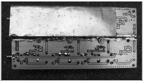
Fig 7: The bottom of the filter bank has an L shaped shielding plate covering the upper half. It is soldered to a metal bar that runs along the middle of the circuit board length.
