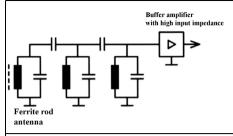
Fig 13: Now for something different: developed from the simple circuit, a circuit with three bandpass filters and a buffer amplifier.
