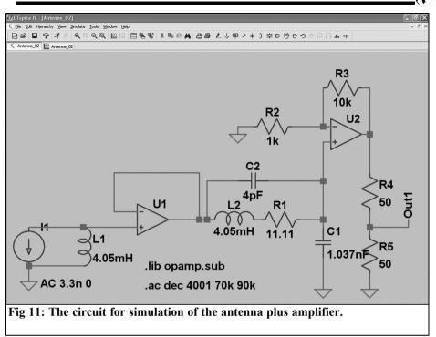
receive the real DCF77 signal in the basement workshop. Result: a display of 31dBm 6.3mV measured at the output "OUT1" with a minimum gain (G = 5.5) using the spectrum analyser. A Spice circuit diagram as shown in Fig 11 was
