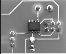
Fig 4: The ICS501 PLL frequency multiplier IC on the test PCB.
