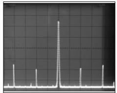
Fig 5: The harmonics of the input frequency are more than 40db down in the output spectrum of ICS501 PLL ICS510 multiplier.
