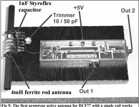
Fig 9: The first prototype active antenna for DCF77 with a single coil works well.
