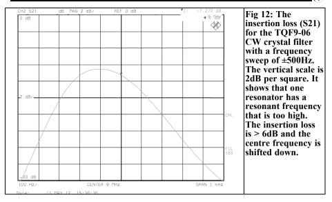
that is not possible with a crystal filter. The filter case would have to be opened and the defective crystal found and replaced by a matching crystal. The "bent" filter curve can be seen even better in Fig 12. Fig 13 shows the out of band attenuation achieved of 90dB.
