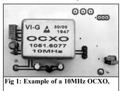
lised oscillator, such as an OCXO (Oven Controlled Xtal Oscillator).
