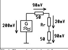
Fig 4: The equivalent circuit for determining the coil losses and the Q. (see text.
