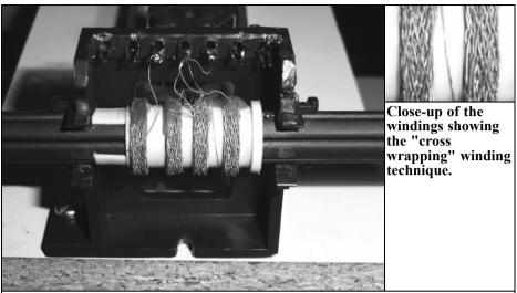
Fig 2: A photograph of the ferrite rod antenna showing the individual windings of Litz wire. These windings reduce the self capacitance and hence increase the self resonant frequency.
