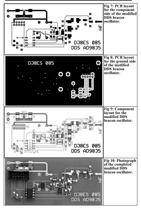
photograph of the completed PCB is shown in Fig 10. The target files and the software in Bascom are available for those who are interested in copying this design. Please send a requests to VHF Communication Magazine [4].
