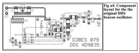
A professionally made PCB is recommended due to the very fine tracks in the area of the DDS module and the many vias that are required. The TARGET files are available on request.
