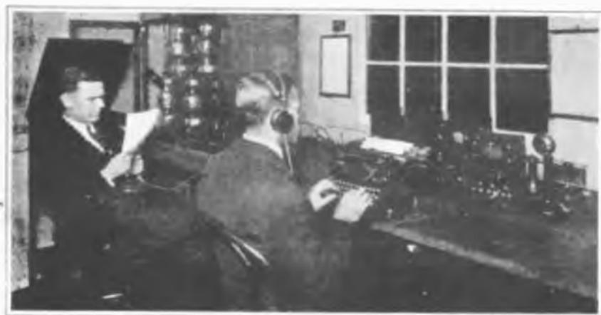
The "announcer" of a radio-phonograph broadcasting station, and the recording operator. The announcer speaks into the radio-phonograph transmitter which he holds in his hand. Alongside of him is the radio-phonograph transmitting apparatus, with the circuit tubes for generating and modulating the radio waves. This is WJL, the Newark radiophone.
