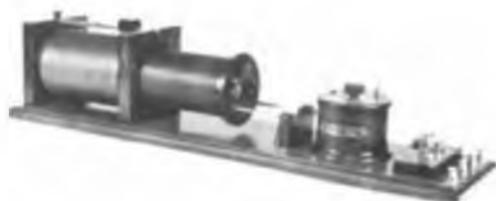
THREE CIRCUIT LOOSE COUPLER RECEIVER
