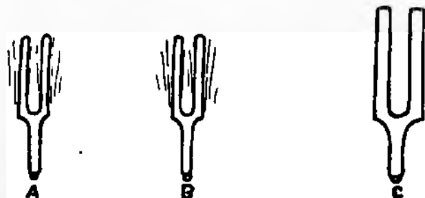
FIG. 11. TRANSFER OF MECHANICAL VIBRATIONS BETWEEN UNITS HAVING SAME FREQUENCY OF VIBRATION.
