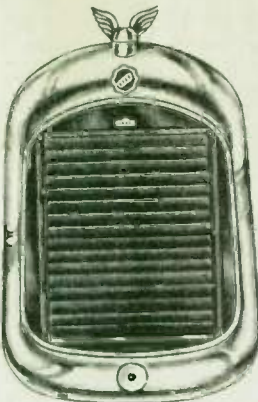
Shows Vernay Shutter on Chrysler Radiator, with vanes closed. The nearest, sturdiest shutter made. A real ornament to the car front.
