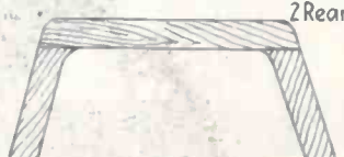
FIG. B-B A RECENTLY DEVELOPED FORM OF CABANE STRUT Section shown at Fig. T
