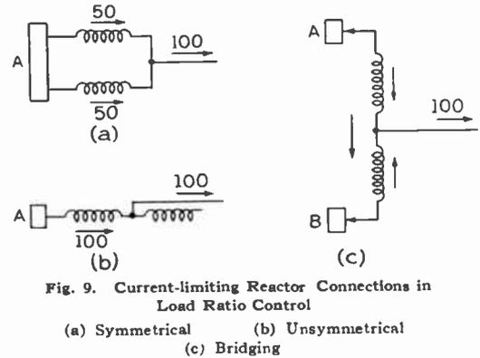
Fig. 9. Current-limiting Reactor Connections in Load Ratio Control
