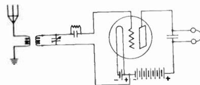
Fig. 14. Diagram of Connections of Three-element Tube as Detector Used with Grid Leak and Condenser
