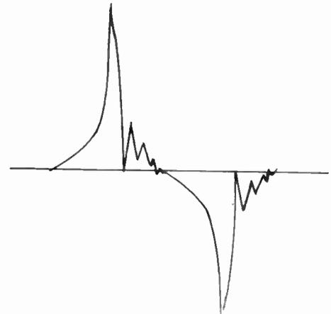
Fig. 10. The Wave Shape for which the Neon Lamps Are Designed to Operate in the New Stroboscope
