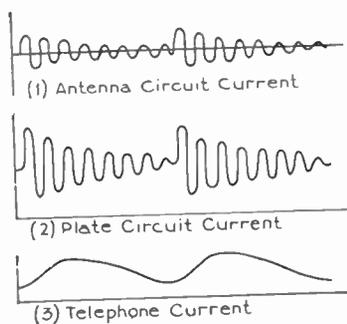
Fig. 13. Oscillograph Curves—Three-element Tube Used as Detector without Grid Leak and Condenser
