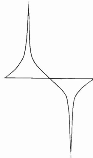
Fig. 7. Secondary Voltage Generated by the Special Transformer Used with the Neon-electric Stroboscope
