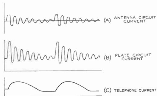
Fig. 6. Oscillographs of Current
