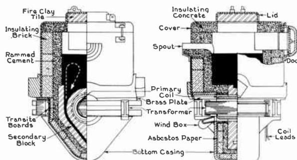
Fig. 70. Sectional Views of a Vertical Ring Induction Furnace
