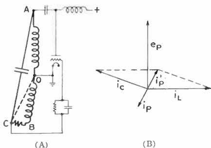
Fig. 24. Effect of Load Resistance in a Hartley Circuit
