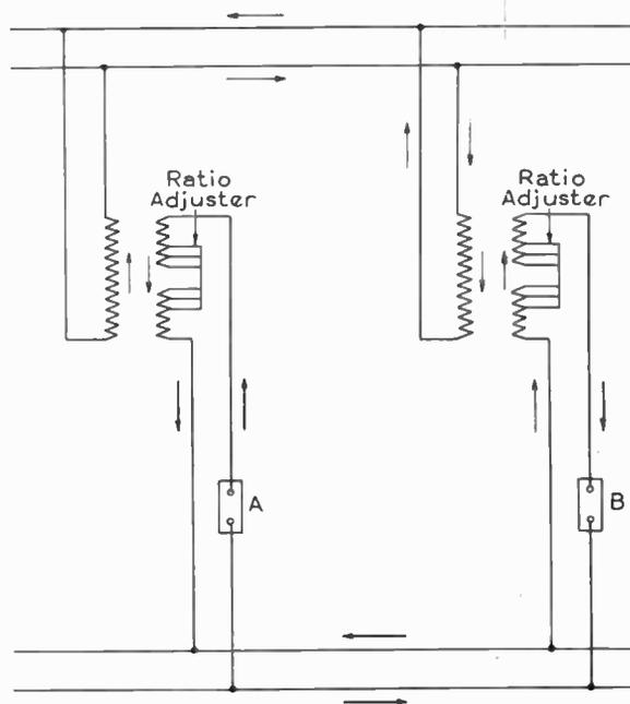
Fig. 3. Elementary Scheme of Connections for Voltage Adjustment by the Use of Two Parallel Transformers Having Suitable Means for Changing Taps
