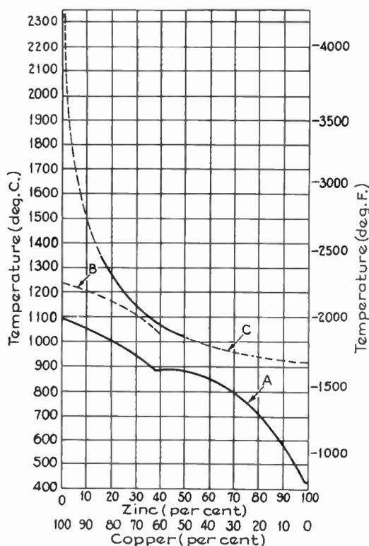
Fig. 58. Temperature Chart for Molten Copper-zinc Alloys (Gillett)
