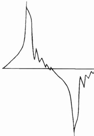
Fig. 9. Tuned Secondary Voltage with Load
