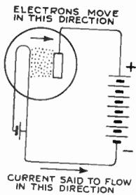
Fig. 2. Diagram Showing Flow of Electrons in Vacuum
