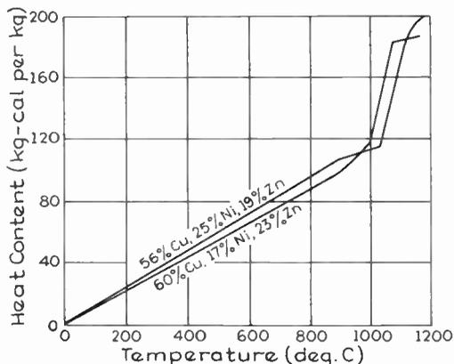
Fig. 60. Heat Content Curves of Two Nickel Silver Alloys (Tama)
