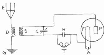
Fig. 5. Diagram of Connections of Fleming Valve as Detector of Radio Signals
