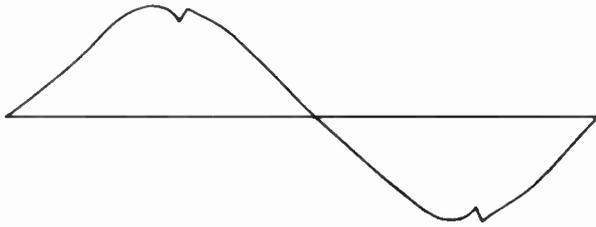
Fig. 11. Voltage Induced in Exploring Coil Used in Making Oscillographic Investigations of Stroboscope Performance
