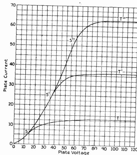
Fig. 8. Plate Voltage—Plate Current Relation at Different Filament Temperatures
