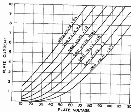
Fig. 10. Plate Voltage—Plate Current Curves for Different Grid Voltages
