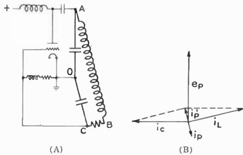
Fig. 25. Effect of Load Resistance in a Colpitts Circuit
