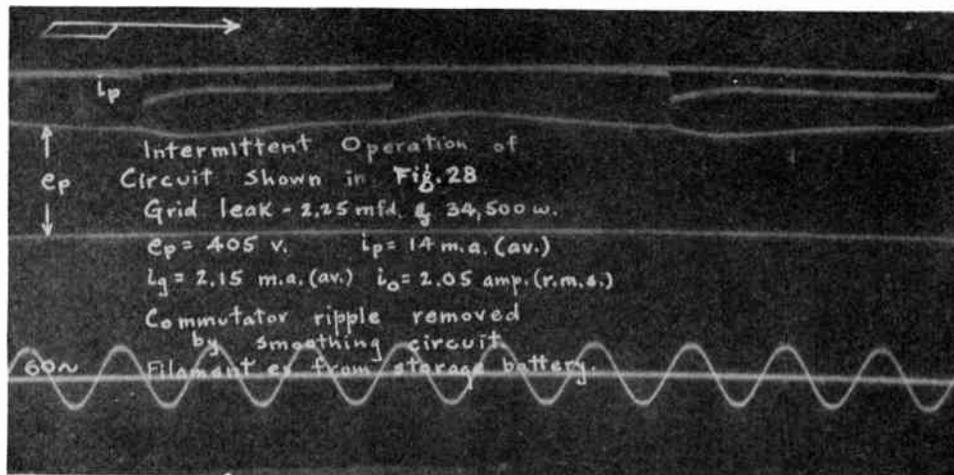
Fig. 30. Intermittent Operation with a Very Large Grid Condenser
