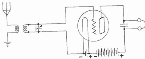
Fig. 12. Diagram of Connections of Three-element Tube as Detector of Radio Signals Without Grid Leak and Condenser
