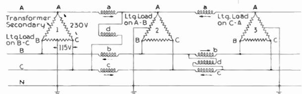
Fig. 14. The Translator Network, Consisting of a Combination of Mid-point Transformer Taps in Separate Phases and Special Devices for Supplying Lighting Loads
