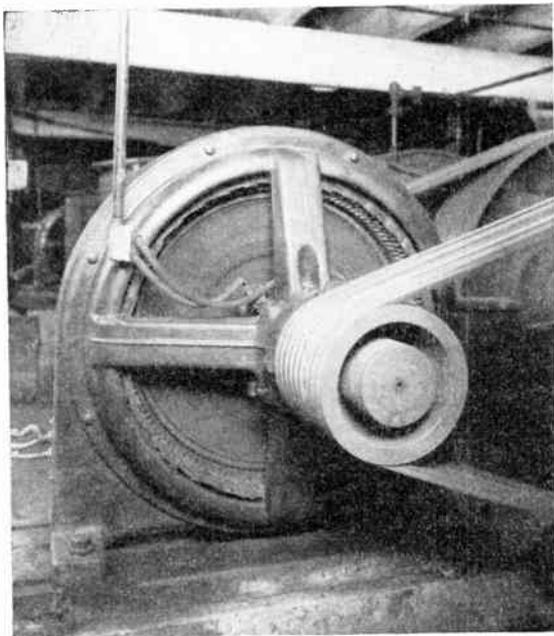
One of the Synchronous Motors Installed
