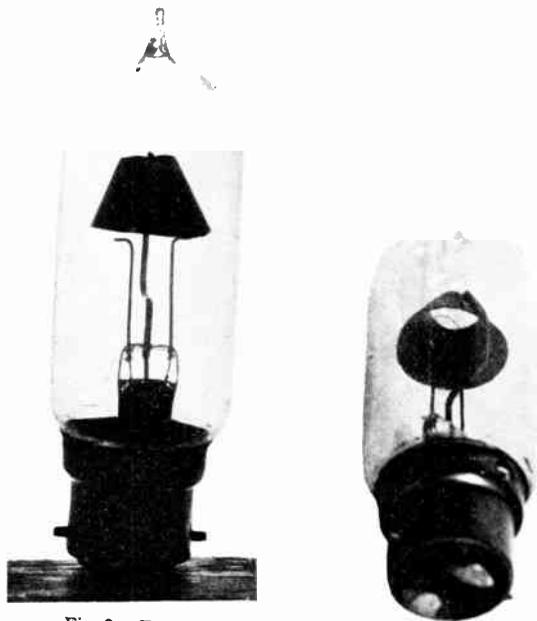
Fig. 3. Two Views of a Two-element Tube or Fleming Valve
