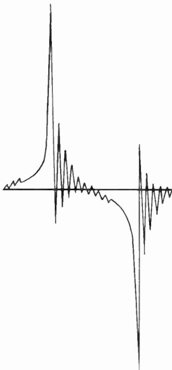
Fig. 8. Tuned Secondary Voltage Obtained Through the Use of a Condenser
