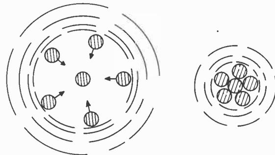
Fig. 61. The Constricting Effect of Electromagnetic Forces Between Parallel Conductors Carrying Currents in the Same Direction
