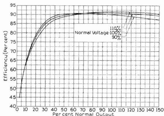
Fig. 8. Approximate Efficiency Curves for a Standard Induction Motor
