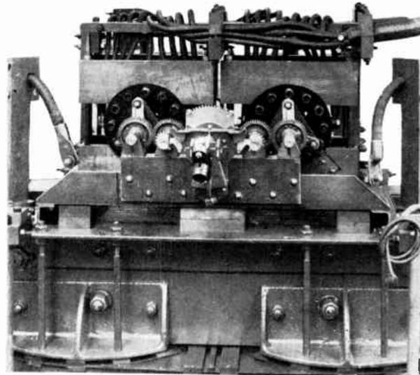
Fig. 5. Close-up View of Intermittent Gear Used to Drive Load Ratio Control Equipment. Single-phase application
