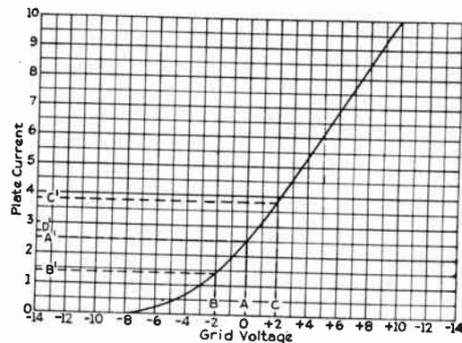
Fig. 11. Grid Voltage—Plate Current Characteristic to Illustrate Action of Three-element Tube Detector without Grid Leak and Condenser
