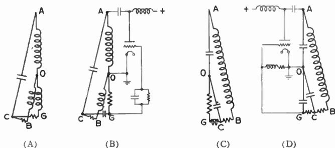
Fig. 27. Special Circuits to Compensate for Errors in Phase of Grid Voltage
