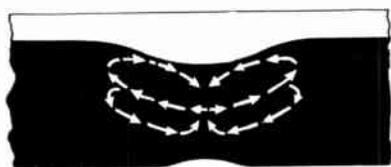
Fig. 62. A Diagram of a Portion of a Molten Metal Conductor, Showing the Constriction of Its Sectional Dimension Occasioned by Electromagnetic Forces
