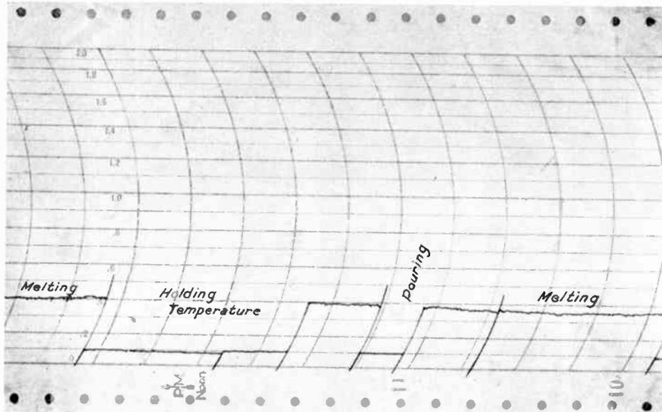
Fig. 71. A Typical Load Chart of a Single-phase 60-kw., 220-volt Vertical Ring Induction Furnace
