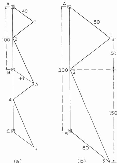
Fig. 11. Diagram Showing the Voltages Derived in Tap-changing with a Circulating Current of 60 Per Cent Full Load at 80 Per Cent Power-factor
