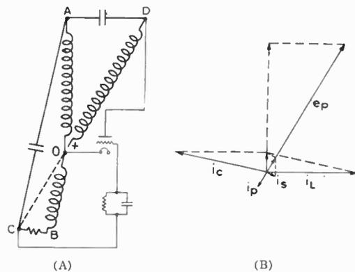
Fig. 26. Effect of Plate Choke and Blocking Condenser
