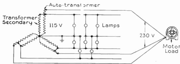
Fig. 12. Auto-transformers Used in Conjunction with a Lighting Supply Circuit to Provide for a Motor Load
