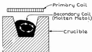
Fig. 68. A Sectional Diagram Showing the Forces Acting Upon the Secondary Circuit of a Horizontal Ring Induction Furnace
