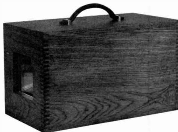
Fig. 3. The Neon-electric Stroboscope
