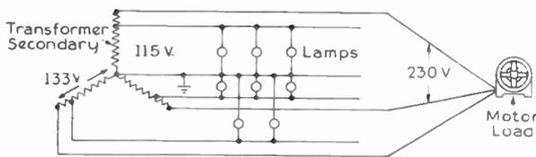
Fig. 13. A System Providing Proper Voltages for Lamps and Motors Through the Employment of Transformer Taps
