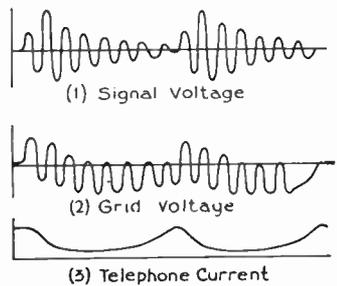
Fig. 15. Oscillographs of Signal Voltage, Grid Voltage and Telephone Current of Three-element Tube Detector with Grid Leak and Condenser
