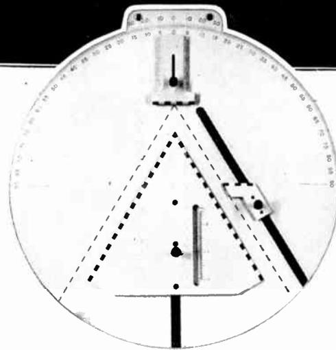
The Bausch & Lomb Contour Measuring Projector is a remarkable time saver in inspecting screw threads. The image can be projected on to a screen, magnified many times, and errors detected at once.
