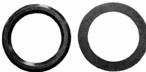
Fig. 69. Starting Rings for a Horizontal Ring Induction Furnace
