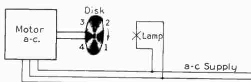
Fig. 1. Diagram of a Simple Form of Stroboscope
