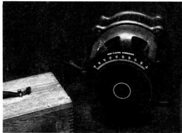
Fig. 5. A Laboratory Set-up with the Neon-electric Stroboscope in Position but Without the Neon Lamp in Operation, for which Reason the Arrows on the Rotating Disk Are Invisible (See cover illustration)
