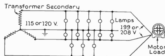
Fig. 7. The Y-secondary System of Distribution for Supplying Combined Lighting and Motor Loads
