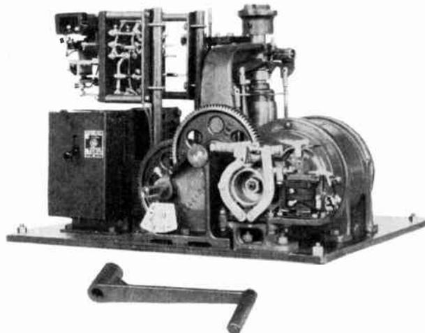
Fig. 6. Driving Mechanism for a Transformer Load Ratio Control. Direct-current Drive
