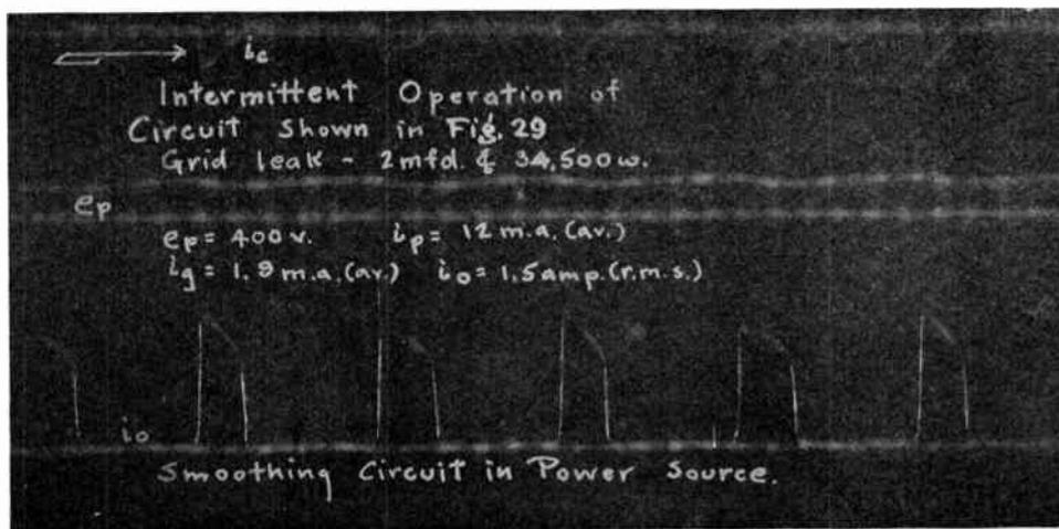
Fig. 33. Intermittent Nature of Oscillating Current
