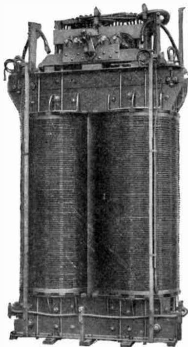
Fig. 2. Load Ratio Control Transformer Removed from Tank
