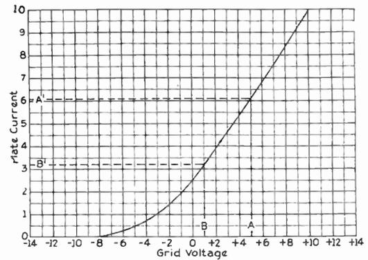
Fig. 16. Grid Voltage—Plate Current Characteristic to Illustrate Action of Three-element Tube Detector with Grid Leak and Condenser
