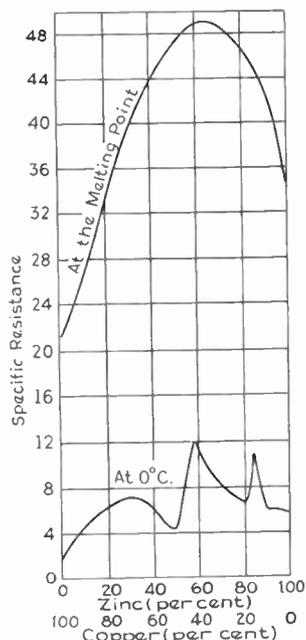
Fig. 64. Relative Values of Specific Resistances for Copper-zinc Alloys in Solid and Molten States (Tama)
