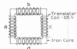
Fig. 16. Elementary Construction of an A-c. Network Translator
