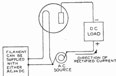
Fig. 4. Diagram of Connections Illustrating Rectifying Action of Two-element Tube
