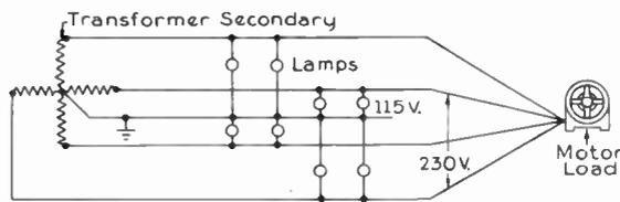
Fig. 11. A Two-phase Five-wire System for Supplying Lighting and Motor Loads
