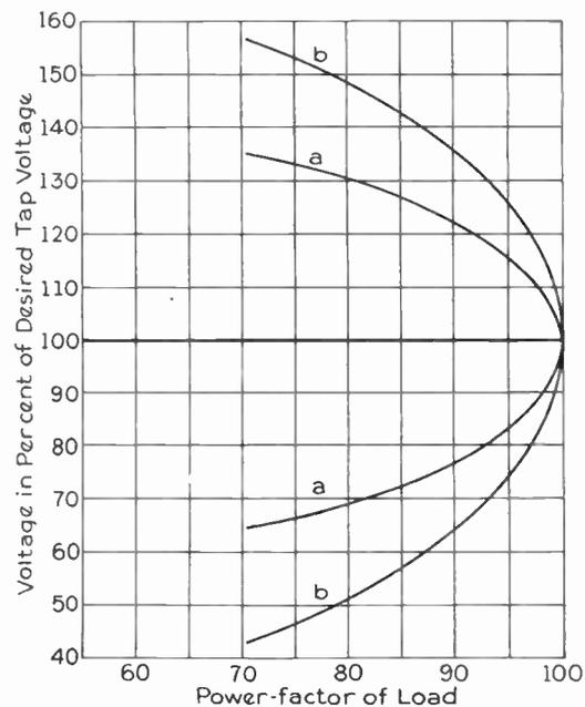
Fig. 12. Unequal Voltage Steps, Caused by Operating Alternately with One and Two Taps Closed, Plotted as Functions of Power-factor
