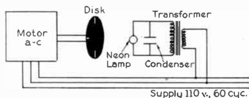
Fig. 2. Diagram of the Neon-electric Stroboscope
