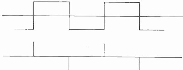
Fig. 6. Rectangular Flux Wave and Induced Voltage
