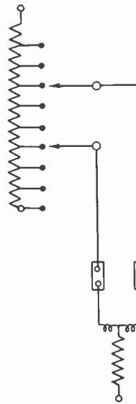
Fig. 8. A Connection Diagram for Load Ratio Control in which Nine Taps Are Provided for Deriving Nine Operating Voltages
