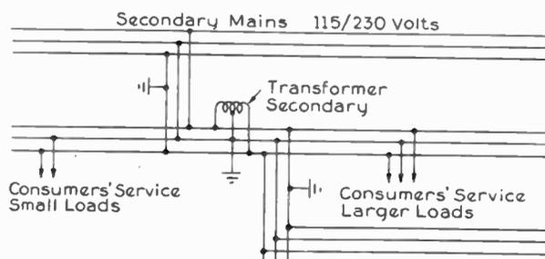
Fig. 5. A Three-wire Secondary Distribution System for Supplying Power for Lighting and Household Appliances
