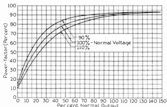
Fig. 9. Typical Power-factor Curves for a Standard Induction Motor
