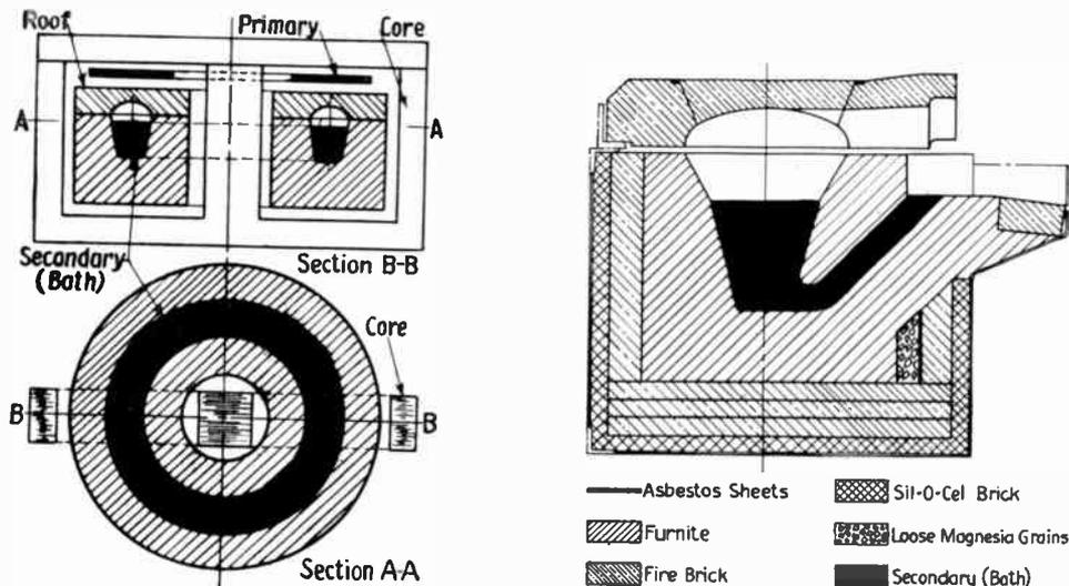
Fig. 66. A Diagram of the Horizontal Ring Induction Furnace, Showing a Section Along the Transverse Horizontal Axis and Another Through the Pouring Spout
