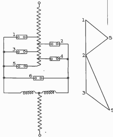
Fig. 14. The Switching Equipment of Fig. 13, Supplemented by the Use of an Additional Unit, 6, Permits Tap-changing in Uniform Voltage Steps. In the voltage diagram, on the right, 1, 2, 3 are operating positions; 4, 5 are transition positions
