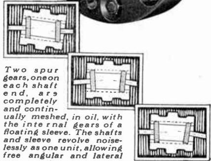
Two spur gears, one on each shaft end, are completely and continually meshed, in oil, with the internal gears of a floating sleeve. The shafts and sleeve revolve noiselessly as one unit, allowing free angular and lateral movement.
