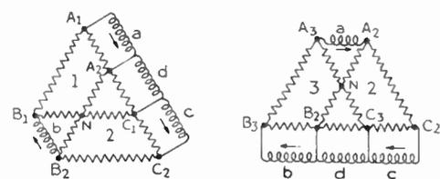
Fig. 15. Diagrams Showing the Relationship of Voltages in the Translator System
