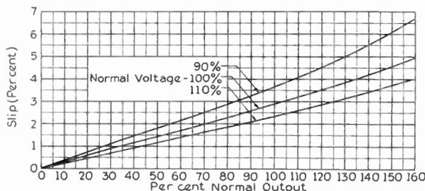
Fig. 10. Approximate Slip Characteristics of a Standard Induction Motor
