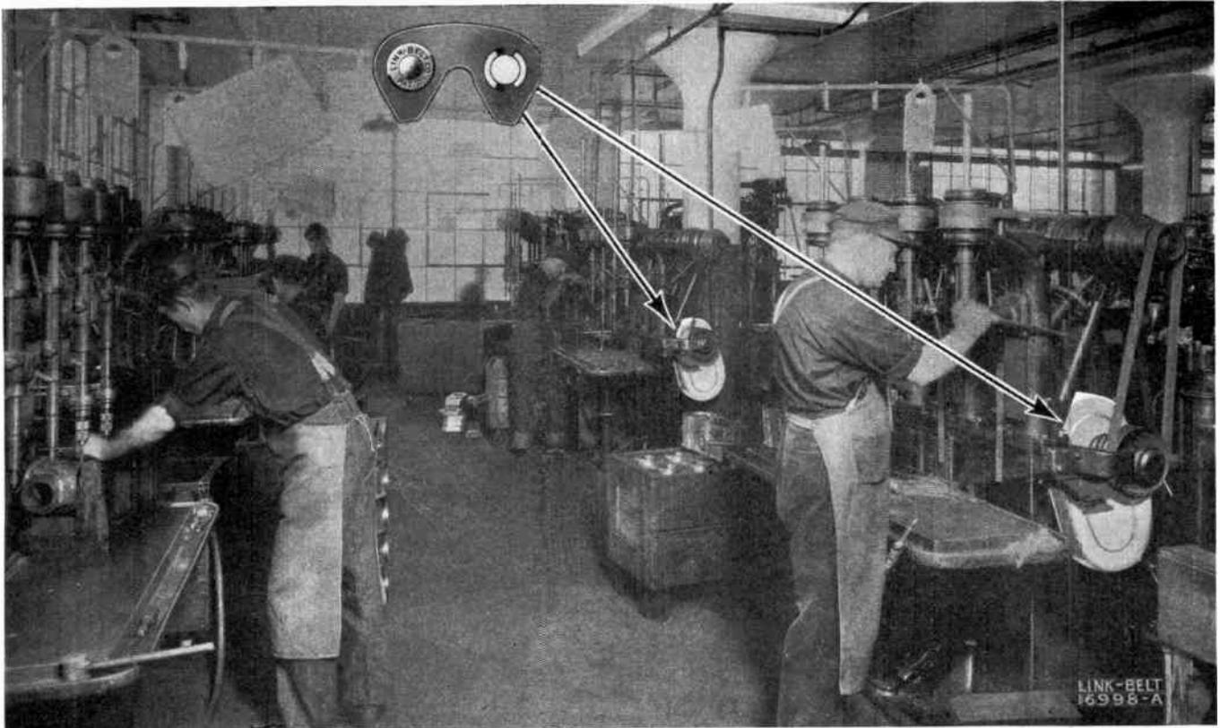
7 Avey drills and 2 Cincinnati Bickford drills using Link-Belt Silent Chain Drives at the Hobart Manufacturing Company, Troy, Ohio.
