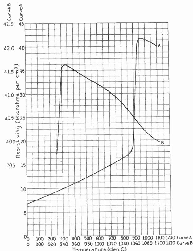
Fig. 65. Resistivity of a Copper-zinc-lead Alloy (Northrup)
