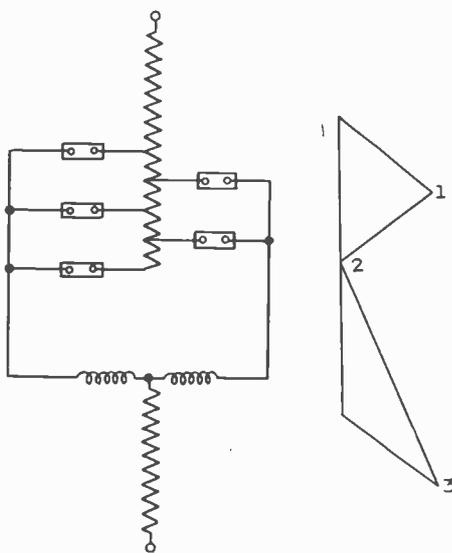
Fig. 13. Connection Diagram Showing How Load Ratio Control May be Accomplished by the Use of Circuit Interrupting Equipment Alone. The voltage diagram appears on the right
