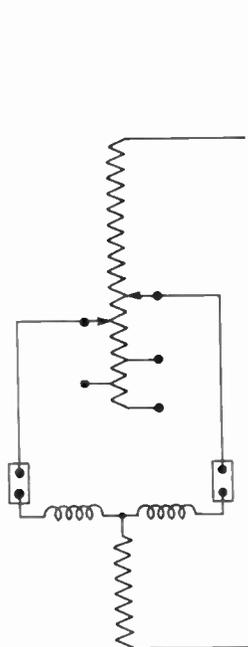
Fig. 10. A Connection Diagram for Load Ratio Control in which All Positions Are Made Operating Positions, Thus Making it Possible to Obtain Nine Voltages by Using Only Five Taps
