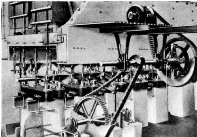
*7½-hp. Morse Silent Chain Drive from motor to countershaft. Driver, 870 r.p.m.; Driven, 100 r.p.m., 55-inch centers. 2½-hp. Morse Silent Chain Drives from countershaft to electrolyzing tanks. Driver, 100 r.p.m.; Driven, 15 r.p.m., 59½-inch centers.*
