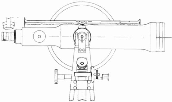
Clear Fused Quartz Pointing Device Shown Mounted on the Telescope of a Precision Theodolite
