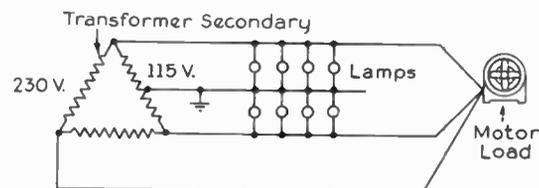
Fig. 6. A Method of Supplying a Lighting Load from One Phase of a Power Transformer that Furnishes Motor Service
