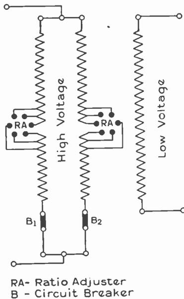
Fig. 7. Diagram of a Transformer Designed with a Multiple Circuit, by Means of which Many Difficulties which Accompany Tap-changing Under Load Are Overcome
