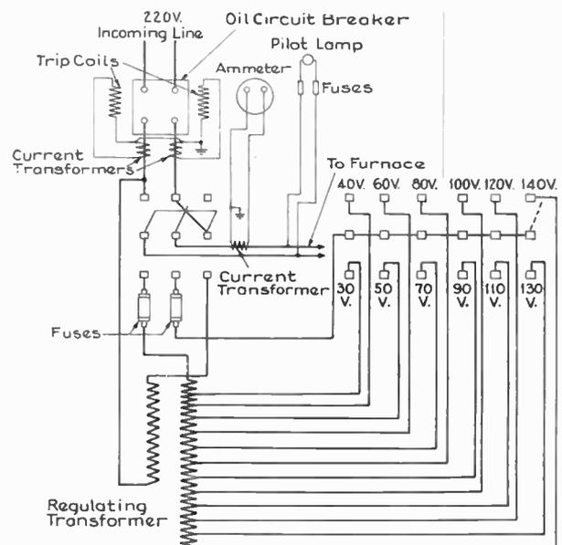
Fig. 72. The Connection Diagram of a Single-phase 60-kw. 220-volt Vertical Ring Induction Furnace
