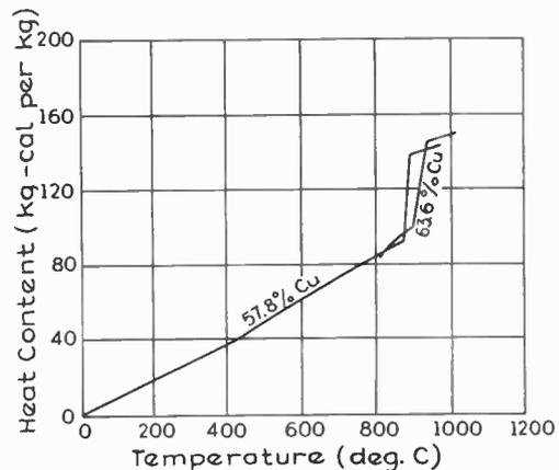
Fig. 59. Heat Content Curves of Two Copper-zinc Alloys (Tama)
