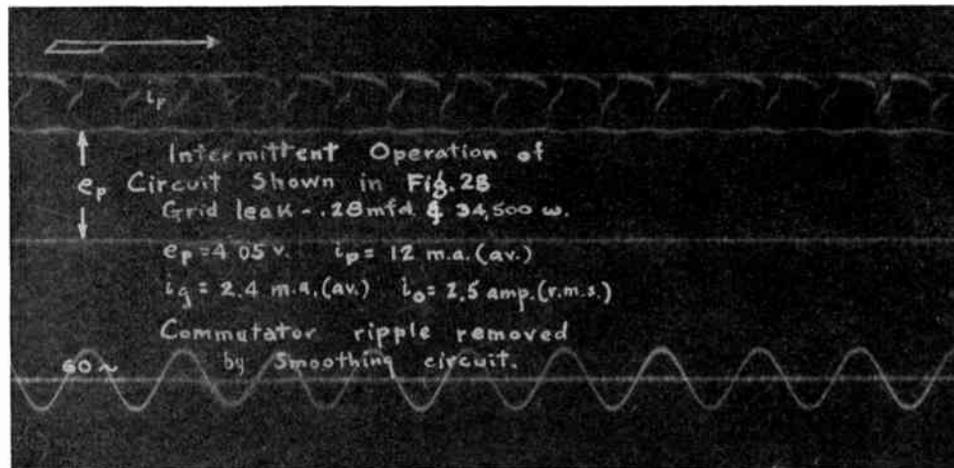
Fig. 31. Intermittent Operation with a Grid Condenser of Smaller Capacity Than is Used for Fig. 30
