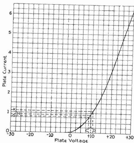
Fig. 7. Plate Voltage—Plate Current Characteristics
