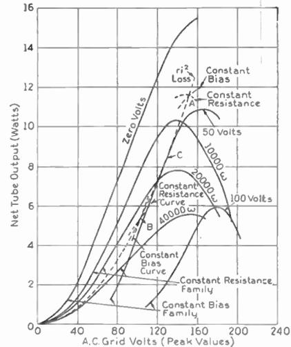
Fig. 34. Curves Showing Grid Circuit Stability of a Small Pilotron Assuming the Alternating Plate Volts as 1.7 Times the Alternating Grid Volts and a Direct Plate Potential of 350 Volts
