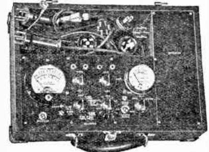
The Modern Set Analyzer. Contains ohmmeter, 0-6,000,000 ohms, and capacity meter, .008 to 10 mfd., both direct reading. A unique and exclusive circuit is employed, providing a new method of set analysis. No serviceman will fail to recognize its superiority and outstanding advantages. Every serviceman needs this instrument to properly test modern receiving sets.
