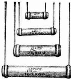
They are wound on a porcelain tube with a special high-grade resistance wire of low temperature coefficient and provided with pig-tail terminal leads 2 in. long. The entire unit is completely coated with a newly developed refractory compound which resists wear and will not chip or crack. The 5-watt resistors. Type 931, are of the same dimensions as our standard 1-watt carbon resistors. Type 1094.
