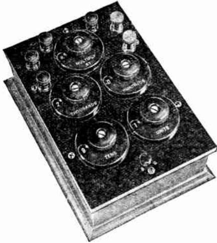
These bridges are similar in construction to Rubicon Type B resistance boxes. Bifilar coils wound on Isolantite spools with double silk covered manganin wire are used throughout. The rheostat dials contain nine coils each. The ratio dial affords a selection of seven multiplying factors—.001, .01, .1, 1, 10, 100 and 1000. The rheostat coils are guaranteed accurate to .1%, while the ratio coils have a guaranteed accuracy of .05%. No variable contacts of any kind are present in the ratio arms.
