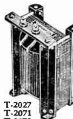
1.5 Henry Choke, 200 mils, 1600 V. insulation. Filter choke in key circuits.
