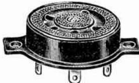
The Type 8 Socket is similar to the Type 12 in the construction of the upper part and the contact springs, but the base consists of a separate, laminated bakelite plate instead of being molded as part of the top. This type of socket is designed for sub-panel mounting. A large hole, approximately 1 1/8", to receive the body of the socket, is drilled or punched through the sub-panel.
