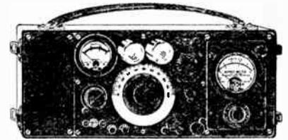
Batteries are self-contained. One 22½-volt "B" and four 1½-volt dry cells are used. The complete instrument is shielded in an aluminum case. An output meter is a necessary accessory for this instrument and a compartment has been provided in the case for the Weston Model 571, which can be purchased with the oscillator. Dimensions: 16¼ x 7 x 5¼". Weight: 15 lbs.
