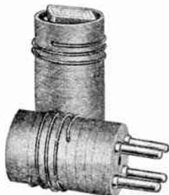
In order to insure stability, maintain calibration, and give maximum efficiency and flexibility to ultra-high-frequency circuits, a low-loss, rigid coil form is essential. These forms are designed to give best form factor and lowest R.F. resistance. Diameter, 1"; length, 1 1/2"; 3/8" wall. Made in standard 4-prong type only. Unwound and ungrooved.
