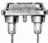
A pair of Tip Jacks moulded in Bakelite providing a completely insulated assembly with embossed designations for single screw mounting. Widely used wherever two Tip Jacks are required. Mounting hole centers  $1\frac{1}{4}$ ".
