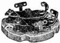
These condensers, except for having two sections, are identically the same as the single described below. Their principal use is for tuning the intermediate frequency transformer stages in superheterodynes. Sensitivity and selectivity depend upon these condensers maintaining constant capacity and constant power
