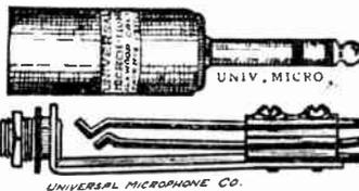
A special design of 3-conductor plug and pack for microphone use. Standard size. High insulation factor. Connection made by solder joint insuring positive connection. Plug size—length overall, 2 7/8 in. diameter, 3/4 in. tip—length, 1 1/2 in. diameter 1/4 in. Jack fits 1/2 in. mounting hole and any panel up to 3/8 in. thick. Overall length, 3 1/2 in.
