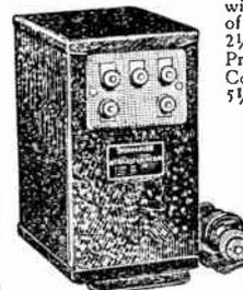
T-2098—A conservatively rated transformer with high voltage winding of 550 volts each side of center tap, and two 7 1/2 volts, 2 1/2 amp. filament windings. Primary: 110 volts, 60 cycles. Cool in operation. Size: 4 1/2" x 5 1/4" x 5 3/4". 13 3/4 lbs.
