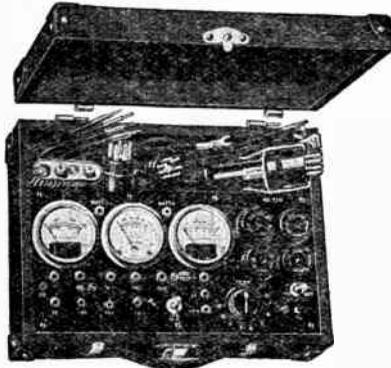
Capacity and resistance charts are furnished showing use of instruments for testing condensers, also measuring resistances up to 100,000 ohms. The nine scale readings of the meters may be used separately with the jack terminals provided. The scale readings are 0-20-60-300-600 D.C. volts, 0-10-140-700 A.C. volts and 0-20-100 milliamperes. Contains new wiring with added 6-hole socket.
