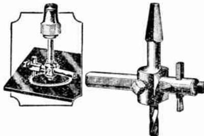
A well-made, substantial tool for cutting holes in panels. Quickly adjusted from  $1\frac{1}{2}$ " to 6". Tapered shank fits carpenter's brace or machine. Center drill penetrates panel while cutter is operating. T-564.
