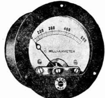
Dimensions—Identical with Model 46. Flange diameter, flush type, 3 1/4"; mounting hole radius, No. 4 screw, 1 1/2"; body diameter, flush and surface, 2 3/4"; depth, 1 3/4"; weight, 7 oz.; scale length, 2 3/8". Bakelite cases.
