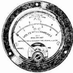
Designed for the serviceman who desires to build a multi-range instrument to fill his particular testing requirements. These instruments are for use with external shunts and external resistances for measuring D.C. voltages and currents and A.C. voltages.
