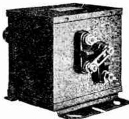
The same general construction has been employed in building the filament supply transformers. They are completely encased and sealed. The primary is arranged for 110 and 220 volts operation with the same method for changing as applied to the plate transformers. The secondary is adequately insulated for operation in connection with its associated apparatus even to the extent of using high voltage porcelain insulator at the terminals. No humid salt atmosphere will affect this transformer.
