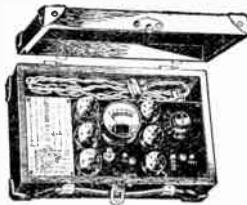
For checking all new and old tubes used in receiving sets. Test card attached to panel gives simple instructions. Anyone can operate. A push button provides two plate current readings for determining the conductance and worth of a tube. A new and outstanding feature applies the same test to rectifier as all other types of tubes. A separate push button provides for testing both plates of '80 type tubes.
