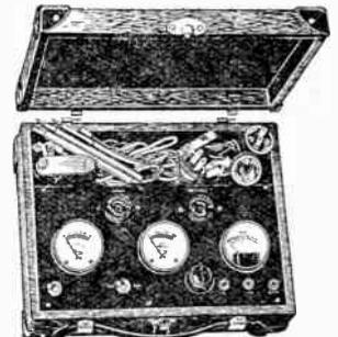
Contains input and output outlets for measuring volts and amperes, A.C. Ammeter reading up to 20 a m p s., A.C. Voltmeter reading up to 300 volts, and a complete direct reading Ohmmeter 0-40, 0-10,000 ohms for continuity testing.
