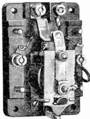
This midget keying relay is suitable for speeds up to 40 words per minute. Contacts are large fine silver buttons assuring long life and may be easily replaced. Coil consumes only 50 milliamperes at 110 volts, 60 cycles, while contacts will interrupt currents of 6 amperes at 110 volts. The unit is designed for mounting on vertical panel, and is recommended for loads up to 660 watts. The contacts close when the coil is energized.
