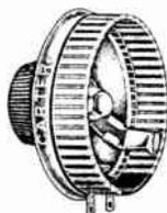
A perfected heavy-duty rheostat of many distinctive features and advantages. Resistance wire is wound on an asbestos covered steel strip. It may be run at high temperatures without danger of destruction and carries safely a load of 25 watts, and is widely used for motor control, radio and experimental work. Mounts in single hole on panels up to 1/8 inch.
