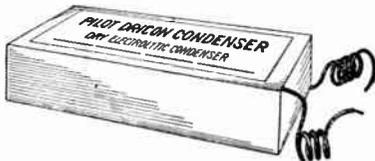
The 4 mfd. unit measures 1 7/8 by 1 by 3/4 ins. long, and the 8 mfd. unit, 1 7/8 by 1 1/4 by 3/4 ins. long. These can be assembled into a very small can to contain the total capacities needed for power supply circuits, and are practically self-healing.
