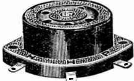
The Type 12 Socket is the Eby "Universal" with the entire shell and base molded in one piece. The arrangement of the contact spring terminals is such that it can be mounted on metal or insulating panels, with terminals projecting above the panel for experimental or above-board wiring, or projecting below the sub-panel for sub-panel wiring. The socket can be mounted on sub-panels with the base above the sub-panel or with simply the top projecting through a large hole in the sub-panel.
