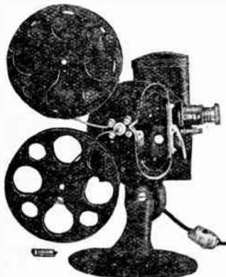
Model A-74 is equipped with a 200-watt special concentrated filament pre-focused projection lamp. A ventilating fan is connected to motor which forces cool air through lamphouse, thereby cooling lamphouse and mechanism. Universal motor drive, 2-inch double achromatic lens, two-claw intermittent movement and perfection oiling system complete this remarkable low-priced projector.
