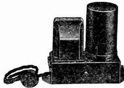
MIK 80 is designed for use solely with PAM 80. Taking advantage of the high amplification of PAM 80, it requires no tubes. It comes equipped with a cord and plug for attachment to PAM 80, through which it gets its power supply. It operates entirely from A.C., including button current supply. A 1,000-ohm variable volume control is provided, but not built into the unit for the sake of portability and convenience. Terminals for the microphone are tip jacks, color coded.
