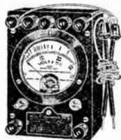
A small compact instrument for voltage and resistance measurements and continuity tests.
