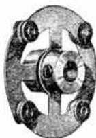
Made of Bakelized canvas, with brass bushings and for 1/4" shafts. Four rustproofed and hardened steel set screws provide against shafts slipping. Overall diameter is 1 1/2".
