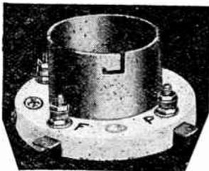
The REL Cat. No. 131-A power tube sockets fit all standard 50-watt base tubes. Maximum insulation is obtained by the use of heavy glazed Isolantite forms. All metal parts are nickel-plated. Connections may either be made to the No. 10 terminal screws or else soldered directly on to the extended portion of the contact springs. All connections are plainly marked.
