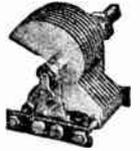
The NATIONAL Type SE Variable Condenser has been designed especially for short-wave work and is not of the "cut down" broadcast variety. Among the outstanding features is the use of the 270° rotation equicycle plates, insulated front bearing, constant impedance pigtail, single hole panel mounting, as well as provision for baseboard mounting. Has 1/4 inch shaft and Isolantite insulation. (Also available with equitune plates, 180° rotation.)
