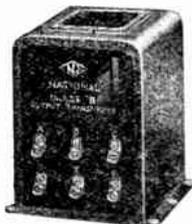
Type B0 Output Transformer for coupling a Class B Amplifier employing 2 210's (operating at a plate voltage of 500 V. and a bias of 57 V.) to a loud speaker or Class C RF Amplifier. Six terminals are available for various loads. The secondary is not designed to carry the RF Amplifier plate current. Insulated for 5,000 volts. Tested at 10,000 volts. Primary inductance 20 henrys; primary resistance (total) 115 ohms.
