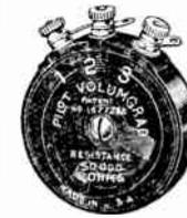
The Volumgrad is a smooth action variable resistor designed especially for volume and oscillation control purposes. The arm is insulated from the shaft, so the Volumgrad can be mounted directly on a metal panel. The maximum power dissipation is 1/2 watt. The maximum voltage across the terminals is 140, 280, and 450 for the four types listed below.
