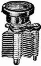
This Midget variable condenser, designed for easy mounting, has a Bakelite frame and rigid brass plates. There are types for neutralizing R.F. amplifiers, antenna coupling, tuning verniers, regeneration control, and short-wave tuning circuits. The depth behind the panel ranges from 1 in. to 1 1/4 ins., depending upon the capacity, with a 1/4-in. shaft.
