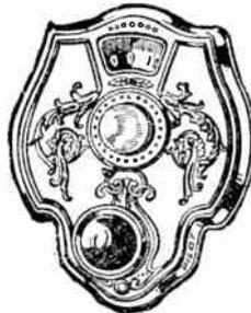
This ornamental vernier dial is made of solid bakelite, and lends an air of distinction to any set. It is available in either black or walnut color. A positive friction drive prevents slipping or backlash, even with heavy triple condensers. Mounts with a single machine screw. The scale is calibrated for both clockwise and counter-clockwise condensers. The dial is 4 inches high and 3 5/16 inches wide.
