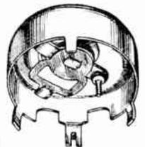
The contact arm and shoe is of new and improved construction. The pressure is automatically held uniform—the action smooth and silent
