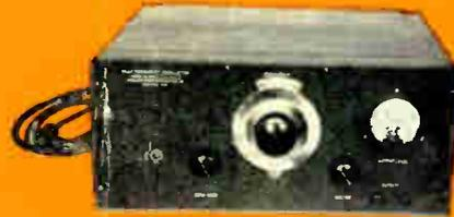
The cabinet has a compartment to hold the batteries, making the instrument completely self-contained. The unit uses three 227 tubes and one 224. The frequency range is from 10 to 10,000 C.P.S., continuously variable.
