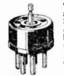
For use with No. 906WL 6-prong analyzer plug above. Six holes top, with center stud 5-prong bottom. All connections through. Suppressor grid contact dead.
