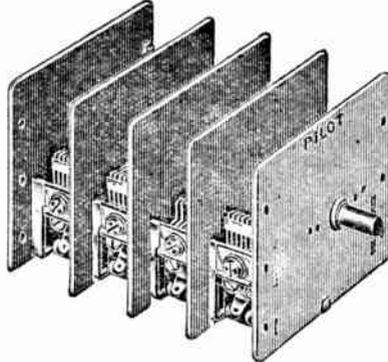
PILOT has developed the Precision Type variable condensers to meet the most exacting requirements of balanced super-heterodyne circuits. Each section has an adjustable compensator to allow for balancing in accordance with the distributed capacities of the circuit to which the sections are connected.
