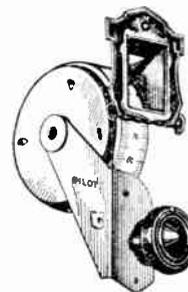
Extreme simplicity and ruggedness have been combined to produce the No. 1273 drum dial at a very low price, although in operation and appearance it is equal to the most expensive types. The drum is intended to be carried on a 1/4-in. condenser shaft. The mounting bracket goes directly on the rear of the front panel. At the top of the escutcheon there is an opening through which a Pilot light can shine to illuminate the celluloid dial on the drum.
