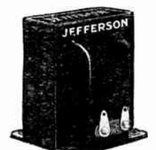
This choke is for use with filament and plate supply transformers Nos. 465-151 and 464-191. It is especially adaptable as choke input for Class "B" amplifier as it aids materially in maintaining the close regulation desirable for this type amplifier. Resistance 190 Ohms; nominal inductance 18 Henries, 50 M.A. Capacity of winding 150 M.A.
