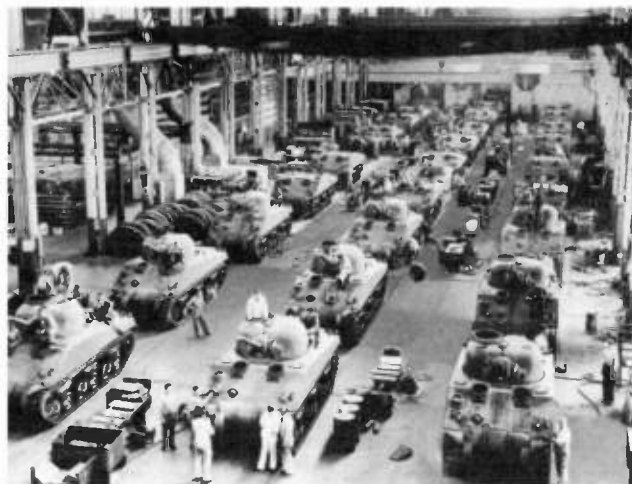
Quantity production of medium tanks on parallel assembly lines.
