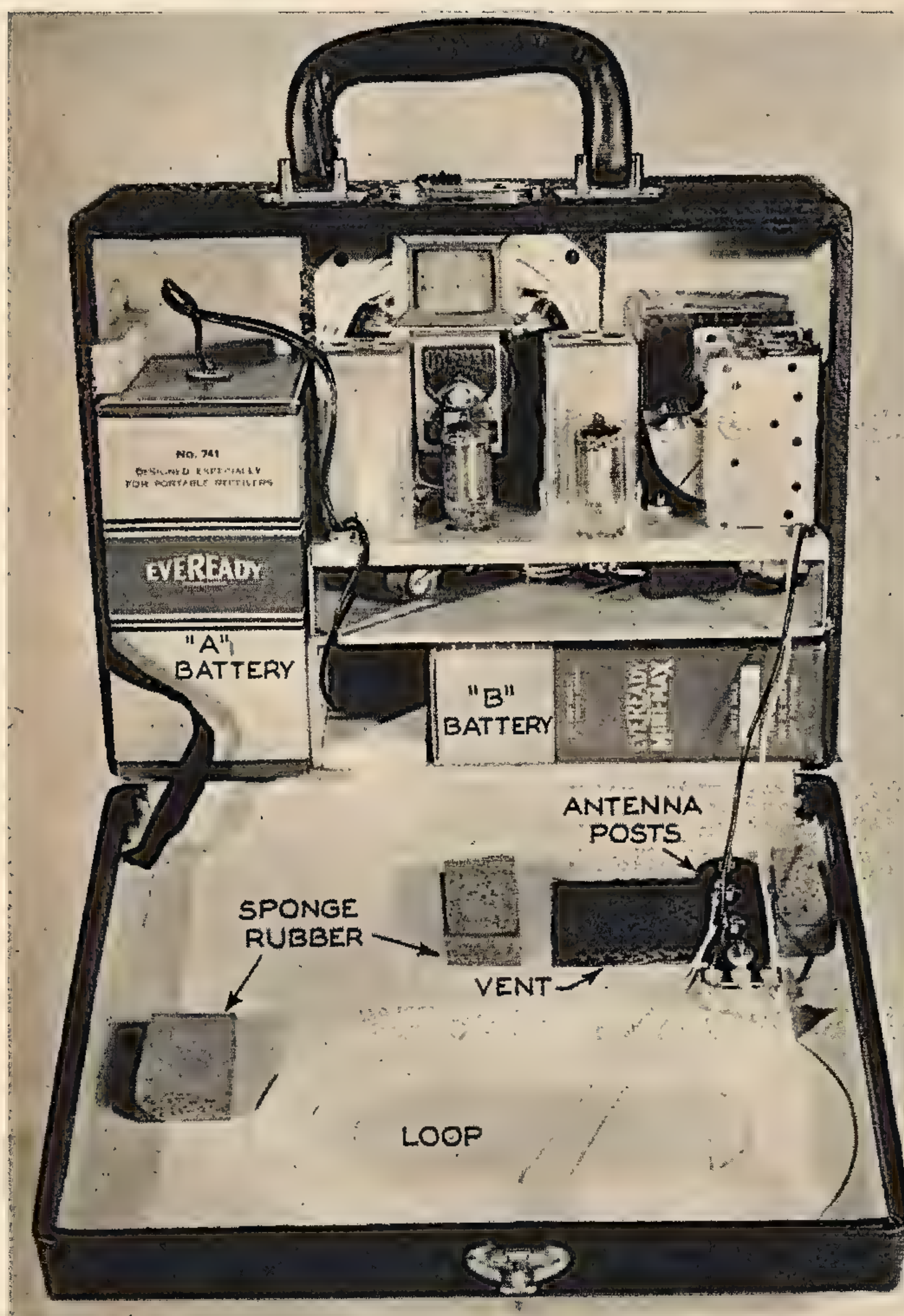
There isn't much empty space inside the "pee-wee" portable! When the cover is closed, the sponge rubber pads press against the "A" and "B" batteries and keep them securely in place.
