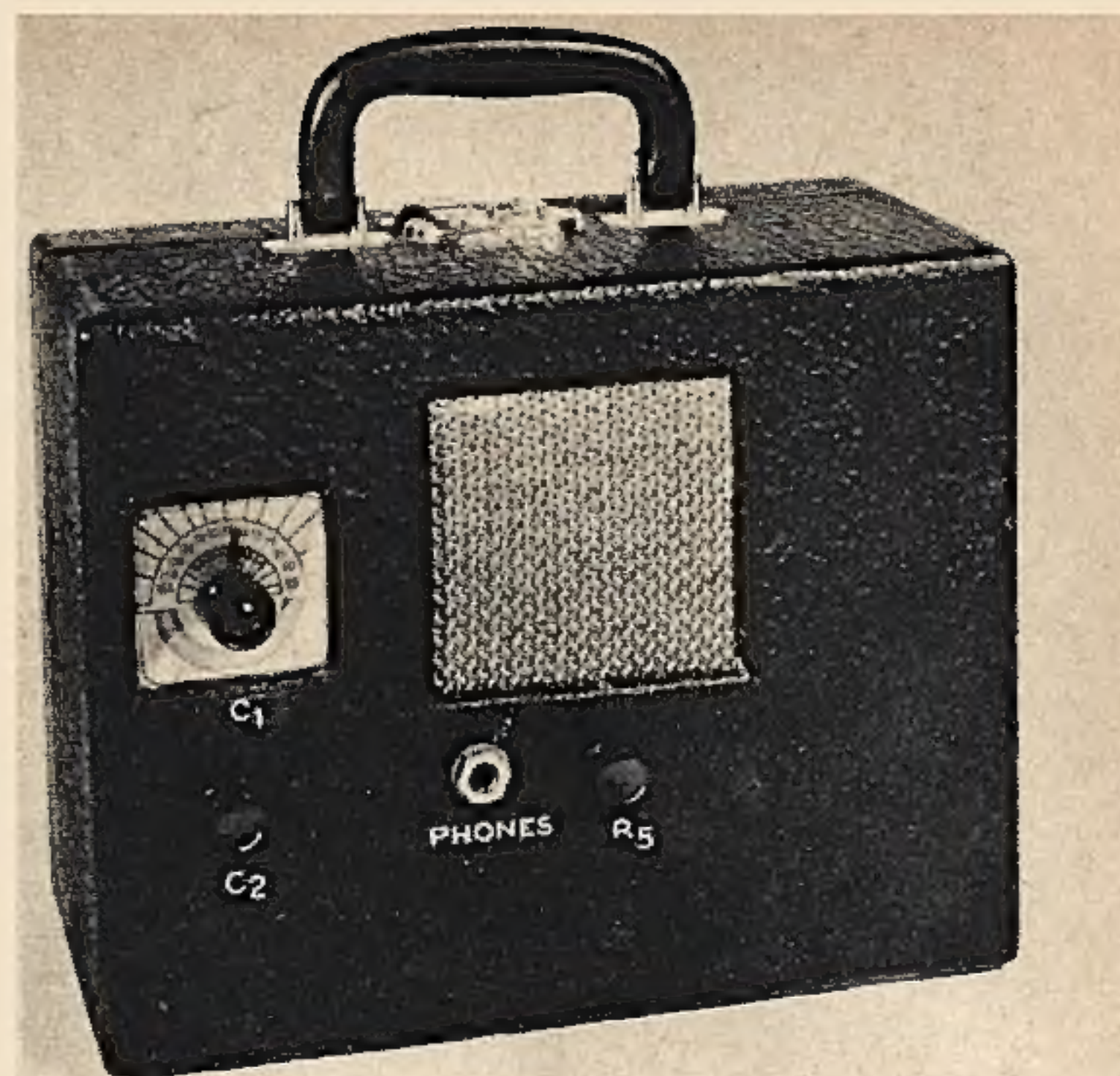
Above: The openings in the front of the case for the loud speaker and the tuning dial are readily cut with a sharp knife.
