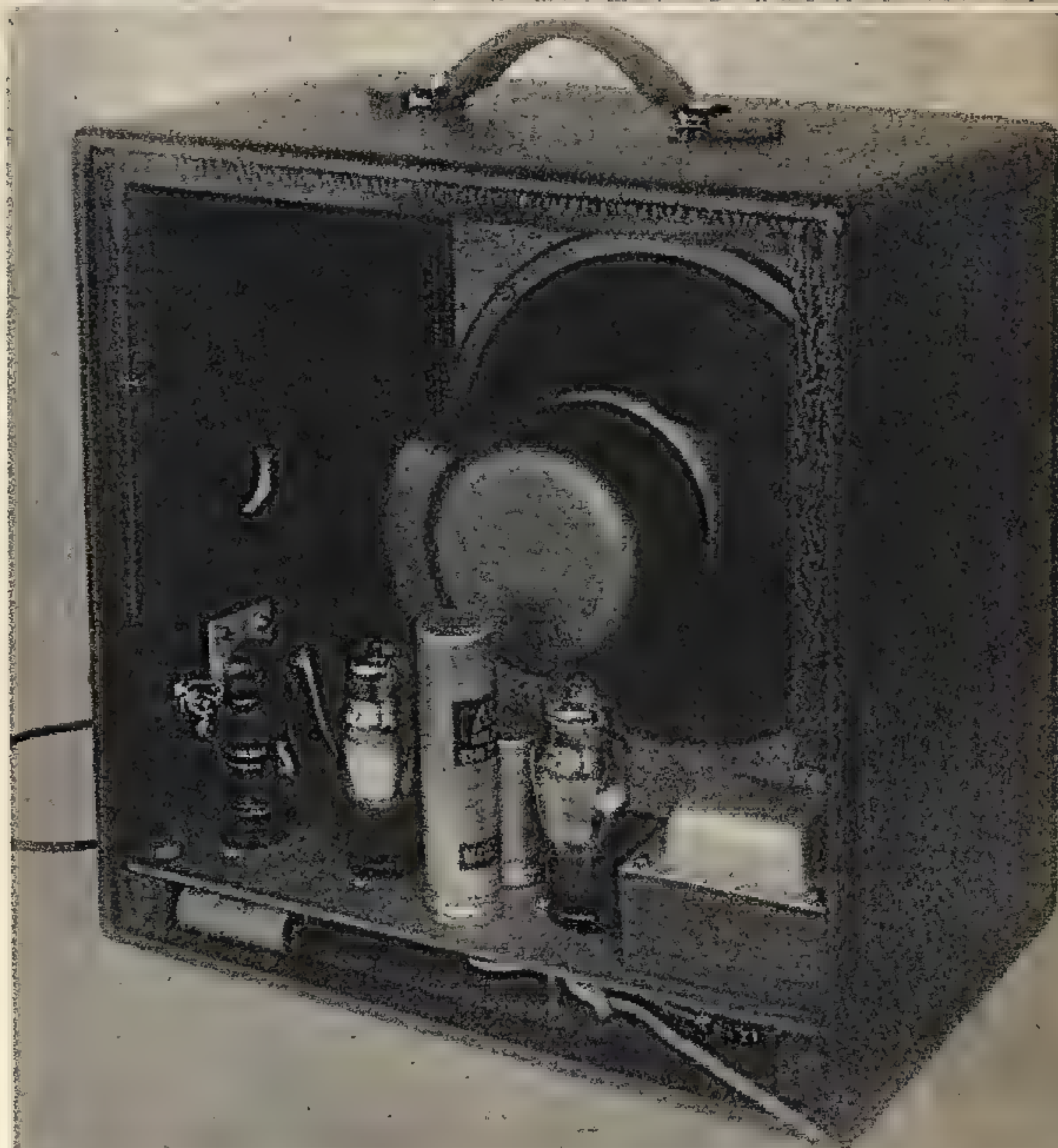
Above—A rear view of the amplifier showing the location of the parts. The power transformer is at the extreme right with the rectifier tube and filter capacitors next. Below is the wiring diagram.
