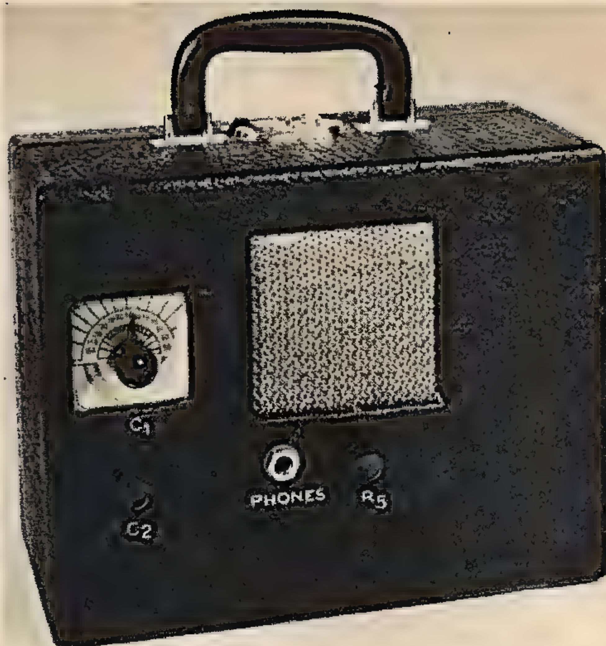
Above: The openings in the front of the case for the loud speaker and the tuning dial are readily cut with a sharp knife.
