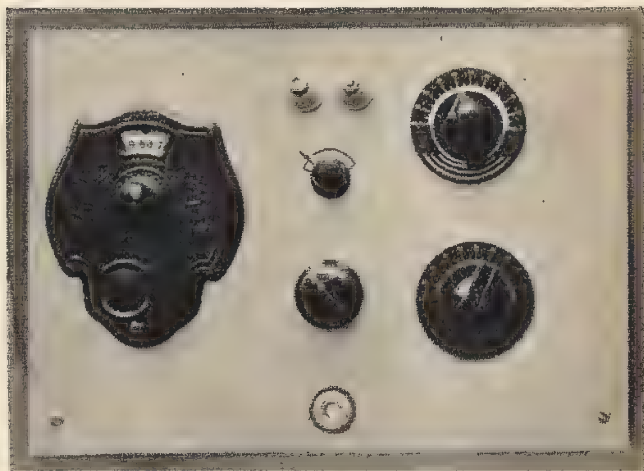
When the set is not in operation, be sure the changeover switch is either in the off position, or on "transmitter." When the switch is in "receiver" position, the potentiometer and dropping resistor are connected across the "B" battery.
