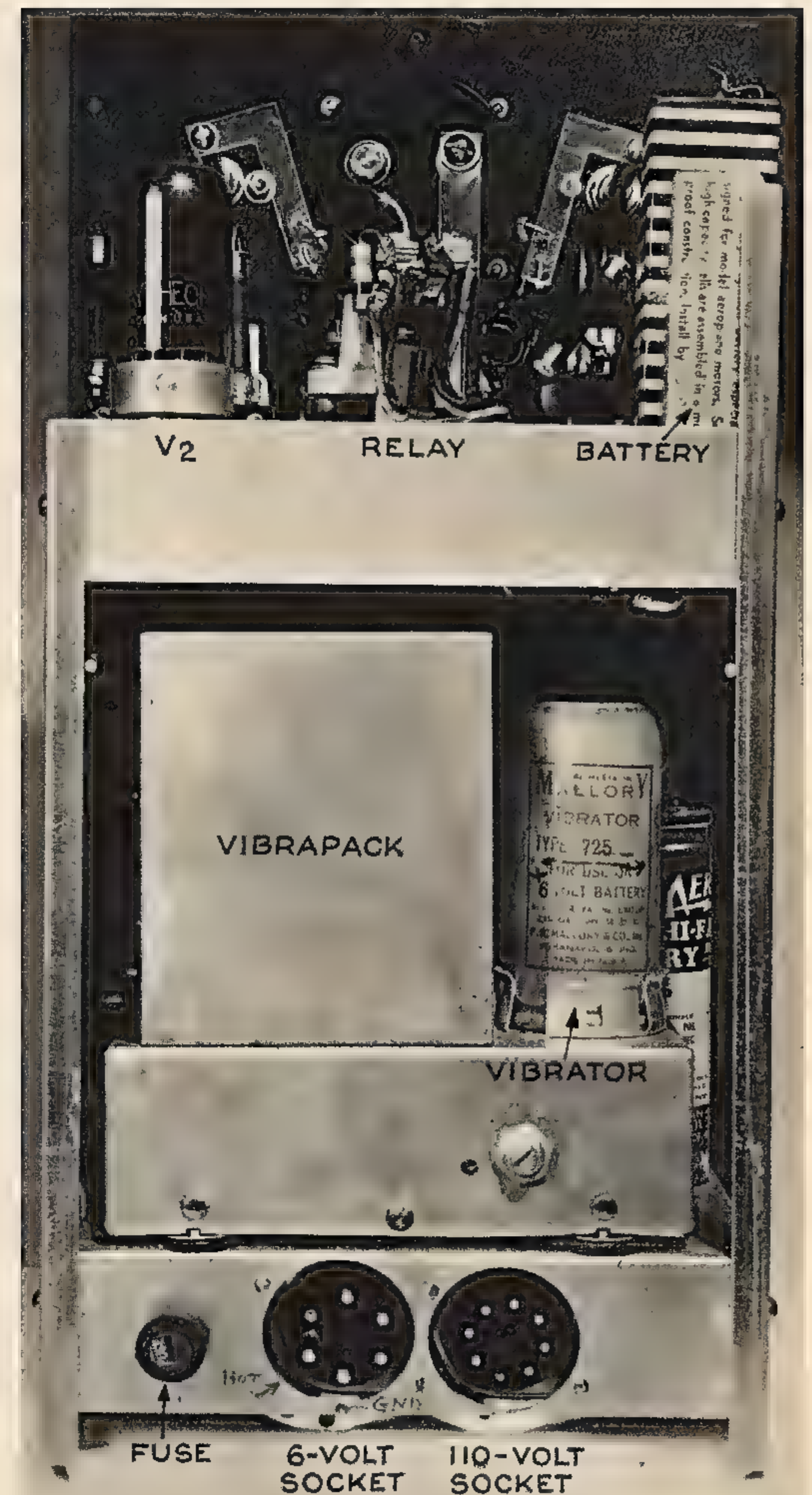
Back view of the completed set. Note that the 6-volt and 110-volt sockets are sunk behind the edge of the bottom chassis.
