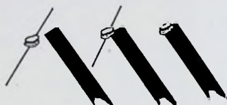
How to mount the small mirror S on the vibrator-strip V. At the left we see the stretched thread carrying the glue and mirror, S. In the second sketch S is being stuck on V. At the right—finished.
