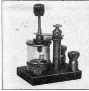
Fig. 62.—An Inclosed Type of Crystal Detector.
