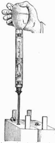
Fig. 77.—Battery Hydrometer Inside the Barrel of a Syringe.
