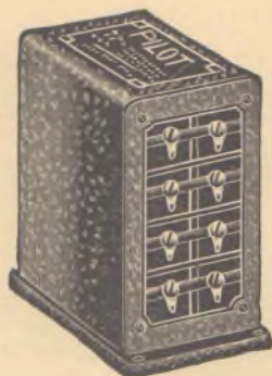
Appearance of Nos. 421 and 396 Condenser Blocks
