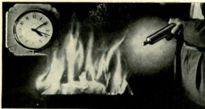
Fire of gasoline-soaked rags is put out (right) in less than three seconds as vaporized methyl bromide from the tiny extinguisher smothers the flames with a blanket of heavy, noncombustible gas.
