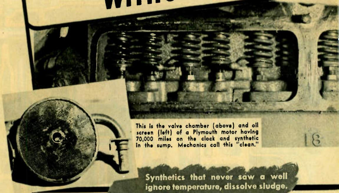
This is the valve chamber (above) and oil screen (left) of a Plymouth motor having 70,000 miles on the clock and synthetic in the sump. Mechanics call this "clean."
