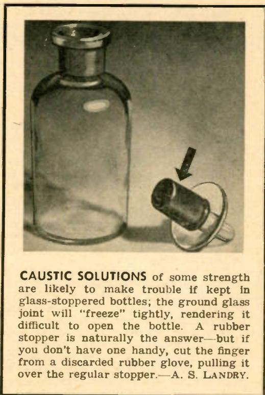
**CAUSTIC SOLUTIONS** of some strength are likely to make trouble if kept in glass-stoppered bottles; the ground glass joint will "freeze" tightly, rendering it difficult to open the bottle. A rubber stopper is naturally the answer—but if you don't have one handy, cut the finger from a discarded rubber glove, pulling it over the regular stopper.—A. S. LANDRY.
