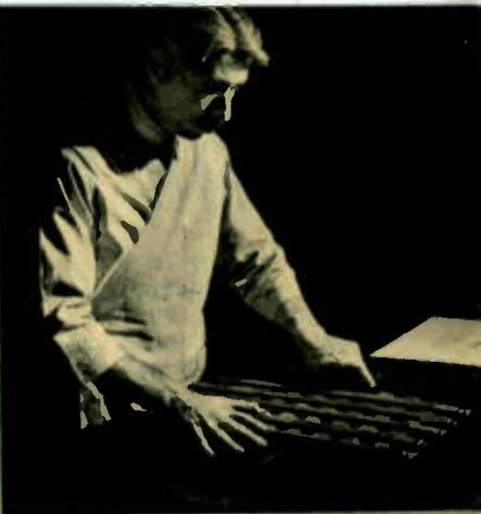
Painting and film are whirled on turntable as X ray is taken. A clearer radiograph is obtained by using this medical technique.
