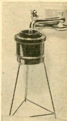
**SINK WASHING** of prints is a pleasure with the drain plug below. A 6" length of 3/4" brass tube has eight or ten 1/8" holes drilled around its top and about twice as many near the bottom. A hole is cut through the center of the rubber plug to take the tube snugly. The lower holes let out the heavier, hypo-laden water at a rate determined by how far in the plug the tube is.—W. T.
