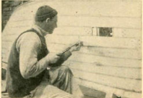
**8** Take care with the planking to get an exact fit, and then bevel the edge for calking. Holes are bored and countersunk deeply, and the screws are put into the butt blacks and frames.
