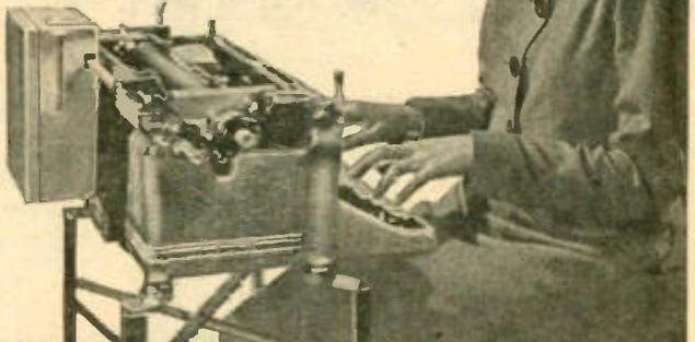
This coin-operated typewriter will be available in hotel lobbies, railroad stations, and even drug-stores. When a dime is inserted, the machine unlocks, setting a meter that measures 325 lineal inches—enough to fill a standard letterhead single-spaced and address an envelope or two. Marlyn C. Ford of Jacksonville, Fla., devised the automatic machine.
