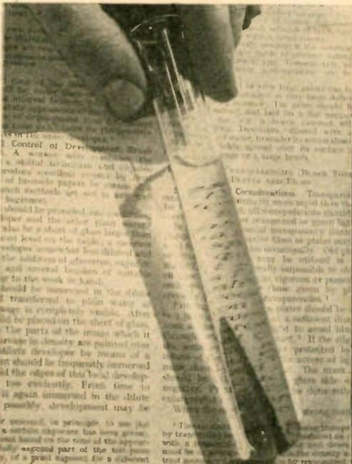
Fully developed black emulsion in the tube (left) becomes a clear solution when a reducer is added. That's how reducers act on overexposed negatives.
