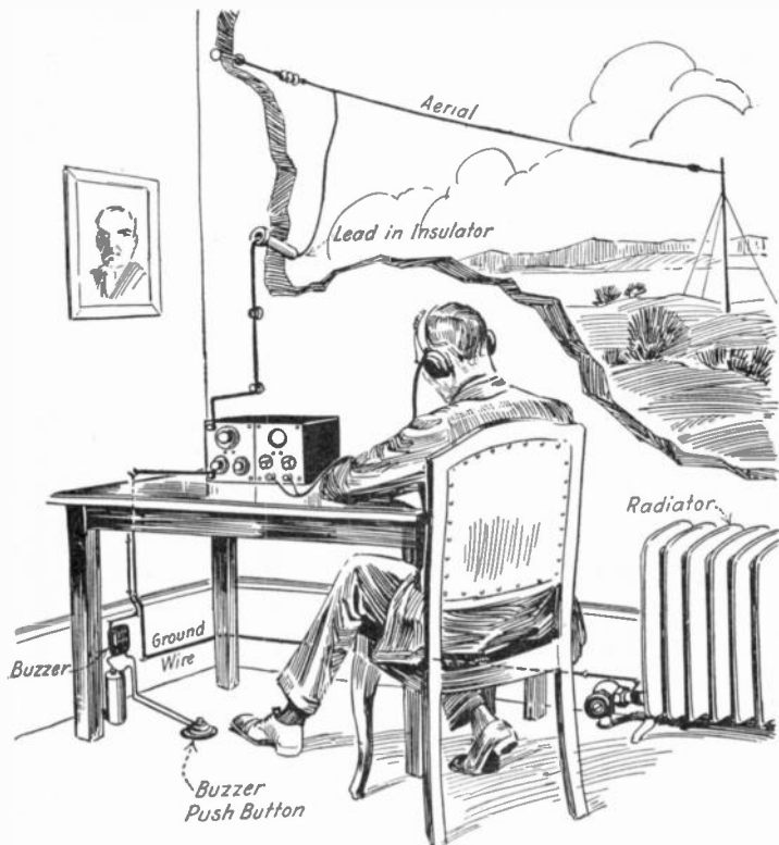
A complete receiving layout, as fully described in the text
