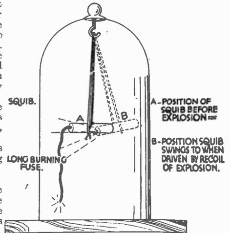
Fig. 6.—To prove that the recoil of a rocket would be effective in the "vacuum" of space.
