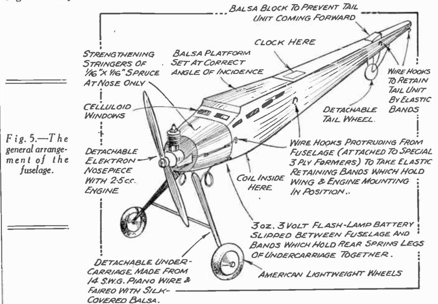
Fig. 5.—The general arrangement of the fuselage.
