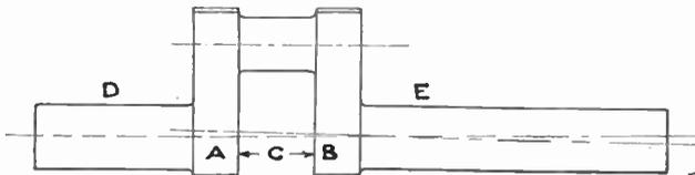
Fig. 1.—The crank shown out of line.
