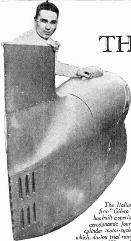
The Italian firm "Glera" has built a special aerodynamic four-cylinder motor-cycle, which, during trial runs, has reached a speed of nearly 190 m.p.h.
