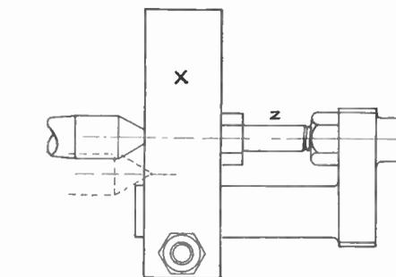
Fig. 3.—The crank ready for chucking.
