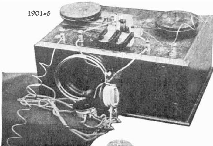
(Above) An early Marconi magnetic detector, period 1901, the predecessor of the crystal detector.
