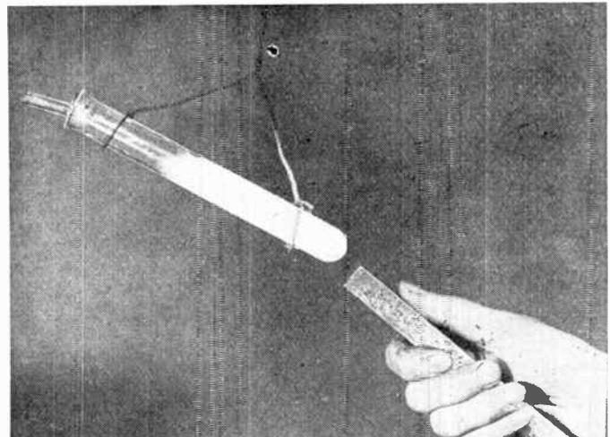
Showing the magnetic nature of liquid oxygen. A suspended tube of oxygen-rich liquid air being attracted to the pole of a bar magnet.
