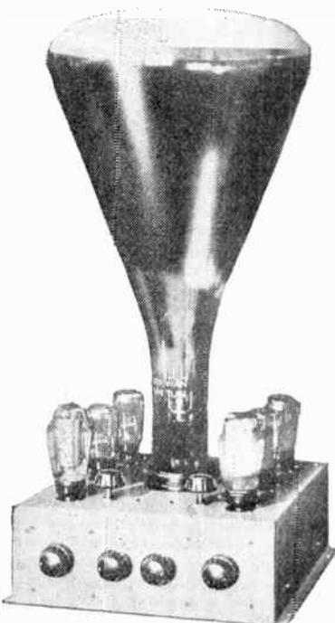
A time-base unit with cathode-ray tube in position, which shows the size of the tube compared with ordinary valves.
