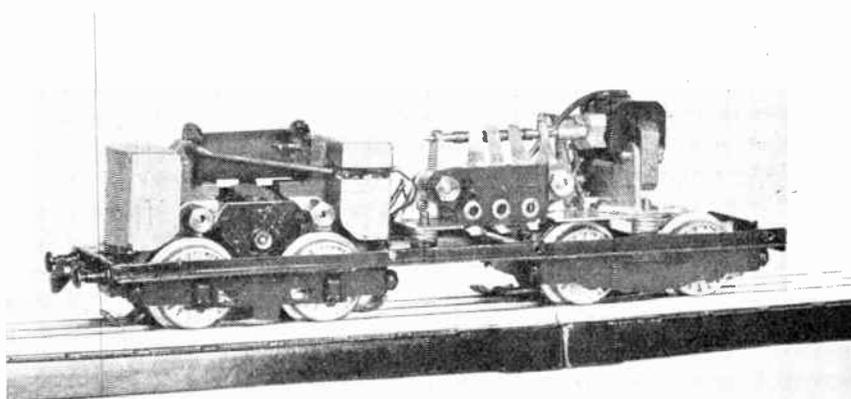
*The motor-coach chassis showing the motor and reversing mechanism.*
