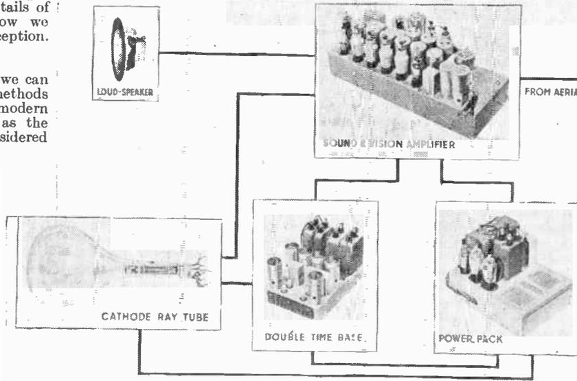
On the left is shown a diagrammatic arrangement of the component assemblies of a G.E.C. television receiver.
