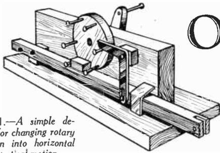
Fig. 1.—A simple device for changing rotary motion into horizontal or vertical motion.
