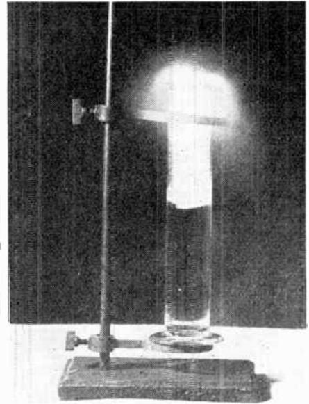
A cylinder containing liquid air. Notice the "fumes" of the liquid caused by the freezing of the moisture in the surrounding air.
