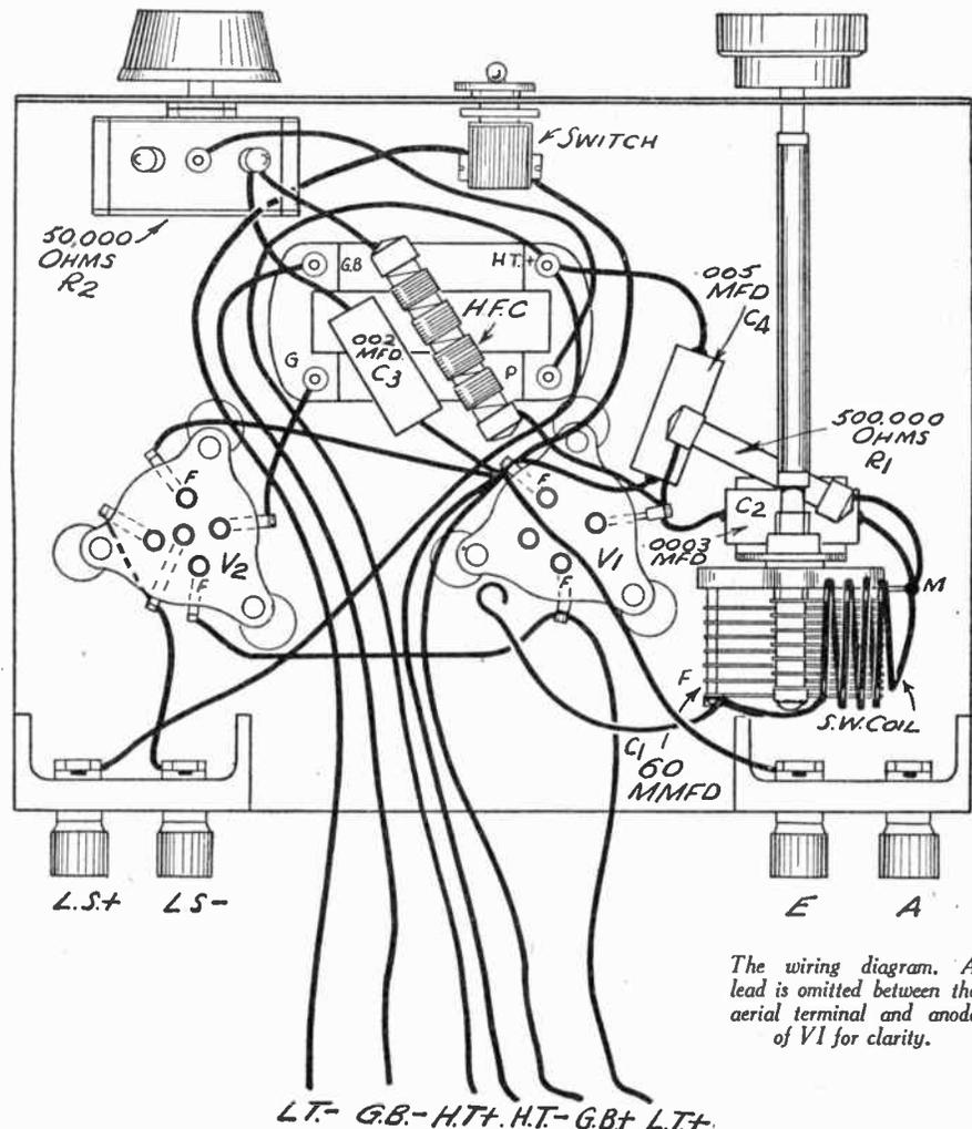
The wiring diagram. A lead is omitted between the aerial terminal and anode of V1 for clarity.
