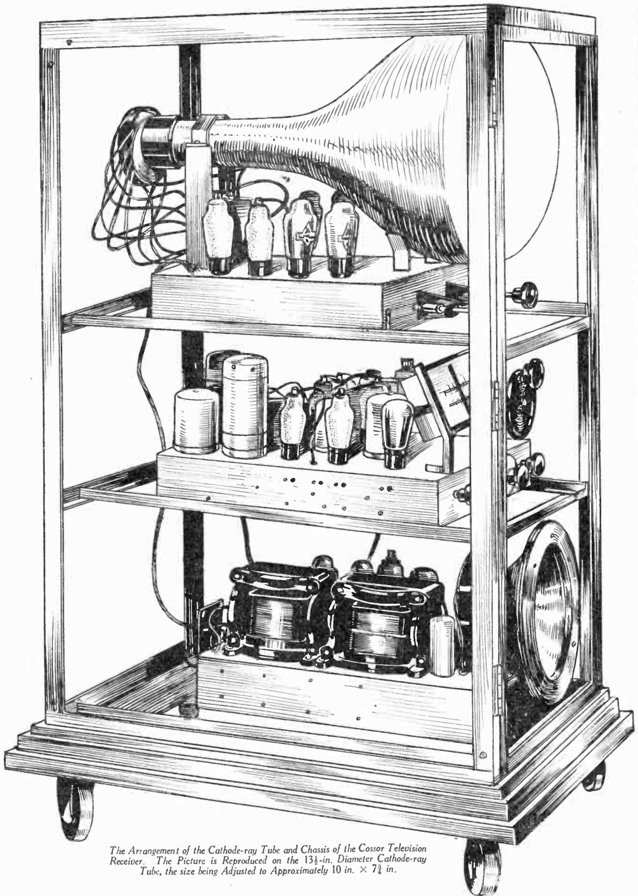
*The Arrangement of the Cathode-ray Tube and Chassis of the Cosor Television Receiver. The Picture is Reproduced on the 13½-in. Diameter Cathode-ray Tube, the size being Adjusted to Approximately 10 in. × 7½ in.*
