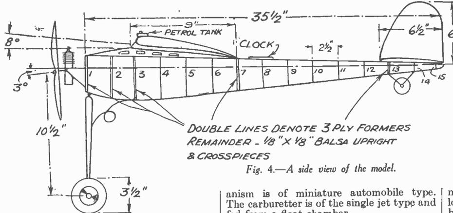
Fig. 4.—A side view of the model.
