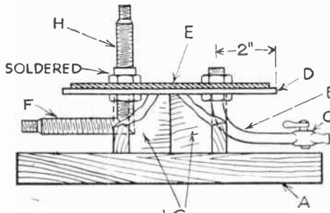
Fig. 1.—A simple yet efficient air-pump. The exhausting platform. A. Baseboard 10 in. × 10 in. × 1 in.; B. Bent gas-pipe; C. Gas-tap fitted to B; D. Metal plate 7 in. diameter, about  $\frac{1}{8}$  in. thick; E. Rubber gasket ring,  $6\frac{1}{2}$  in. overall diameter; F. Right-angled Schrader tyre valve without "inside"; G. Platform support, 2 pieces of  $\frac{1}{2}$ -in. wood, each 7 in. × 2 in.; H. Ordinary short tyre valve with "inside."
