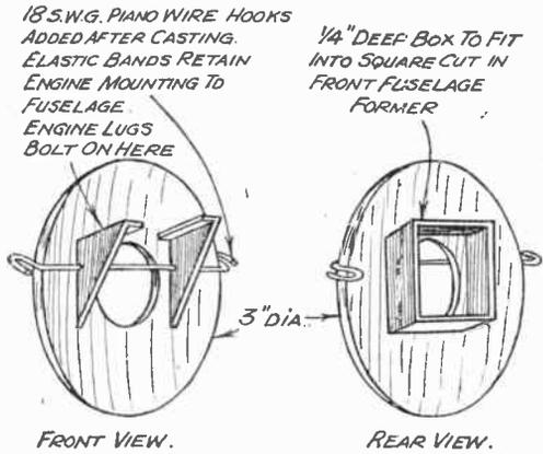
Fig. 6.—A front and rear view of the wooden pattern for a cast elektron mounting for the "Elf" or other 3-c.c. engine.
