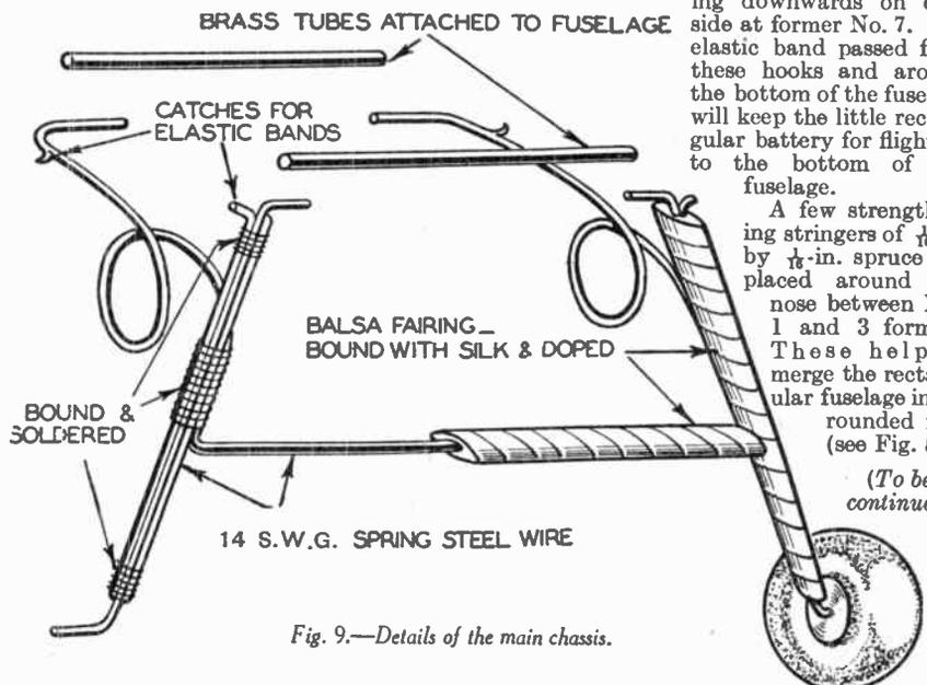
Fig. 9.—Details of the main chassis.
