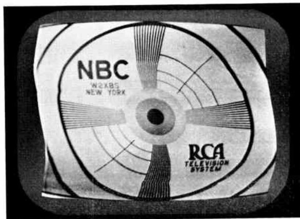
Figure 47—Excessive Ripple in Horizontal Deflection
