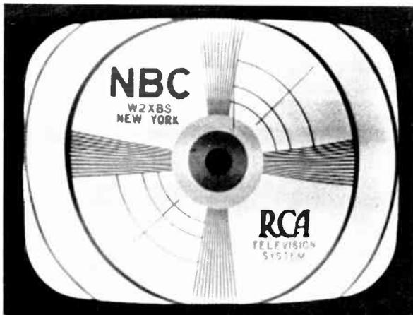
**Figure 53—Loss of Interlacing**
