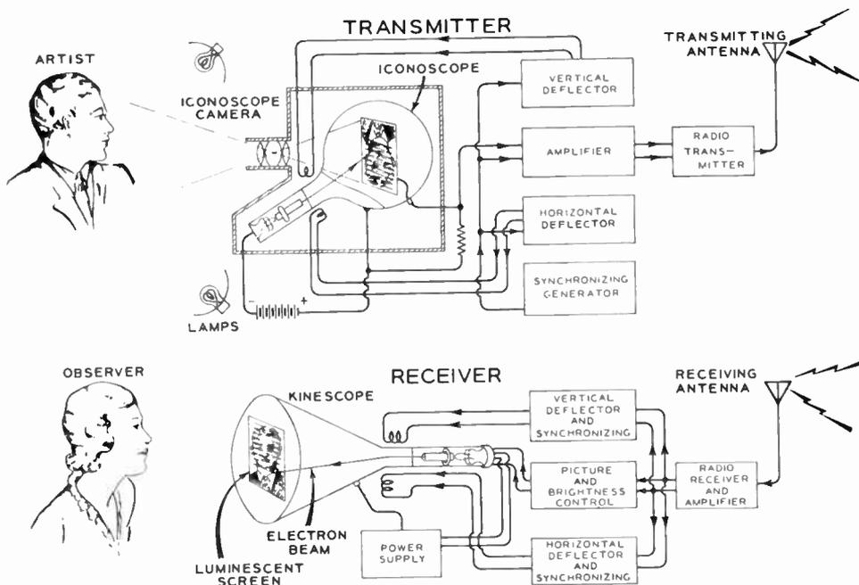
**Figure 1—Schematic of RCA Television System
