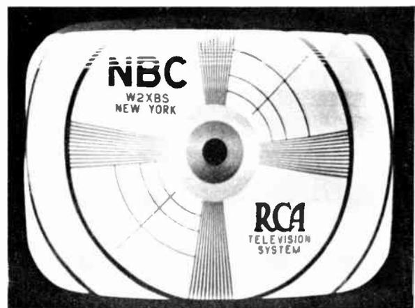
**Figure 55—Vertical Distortion Caused By Defective Peaking**
