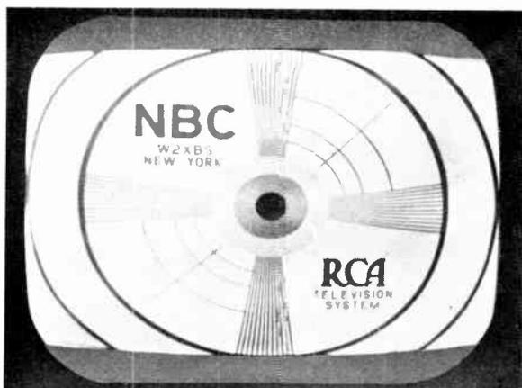
**Figure 37—Vertical Height Control Incorrectly Set**
