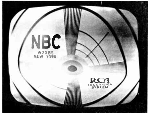
**Figure 54—Excessive Ripple in Vertical Deflection**
