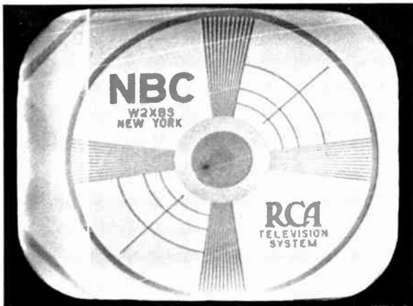
Figure 60—Effect of Damping Tube Failure
