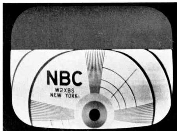
**Figure 38—Vertical Centering Control Incorrectly Set**
