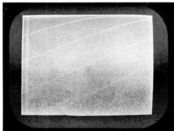
**Figure 39—Scanning Raster Correctly Oriented**
