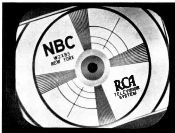
**Figure 34—Picture Incorrectly Oriented**
