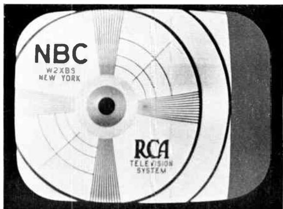
**Figure 36—Horizontal Centering Control Incorrectly Set**
