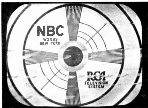
Figure 44—Excessive Auto Ignition Interference
