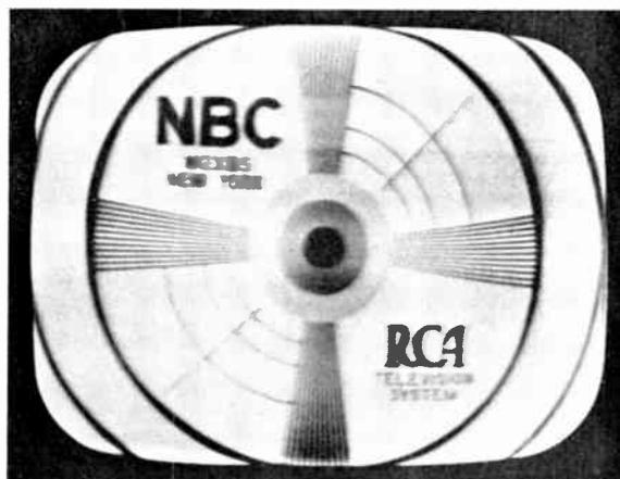
Figure 58—Loss of High Video Frequencies
