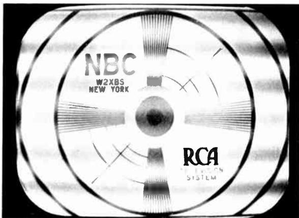
**Figure 33—Sound Modulation in Picture**
