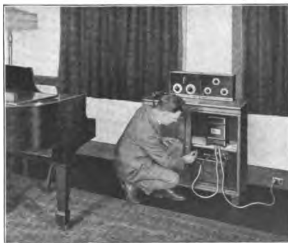
Illustrating the simplicity of battery charging when A. C. is available.
