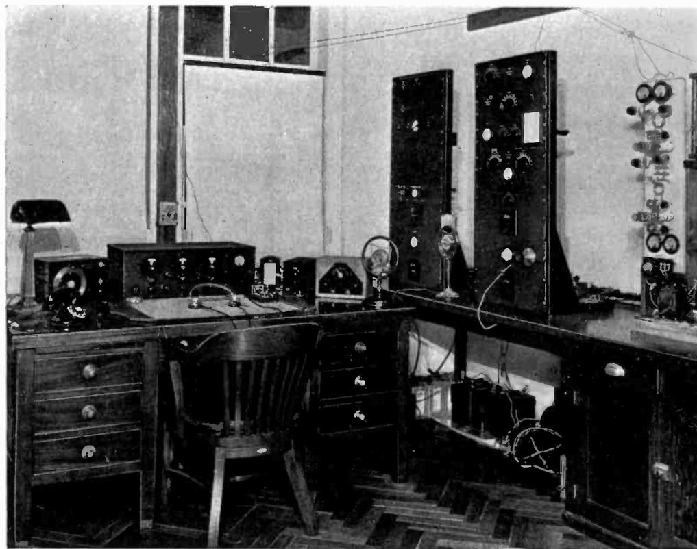
Station "W2GEC". G. E. Burghard, 520 East 86th St., N. Y. C., 1934. Left to right: Frequency meter, single signal superbet, 5 meter super-regenerative receivers, Modulator panel, C. W. transmitting panel, 20 to 180 meters, and 5 meter M.O.P.A. transmitter.
