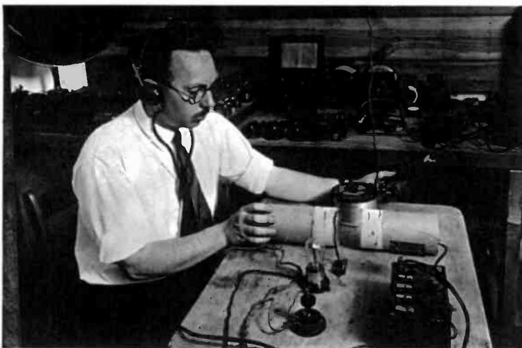
*Typical amateur transmitter of the rotary synchronous spark gap era in 1919. The rig was built and operated by Lester Spangenberg in New Jersey.*
