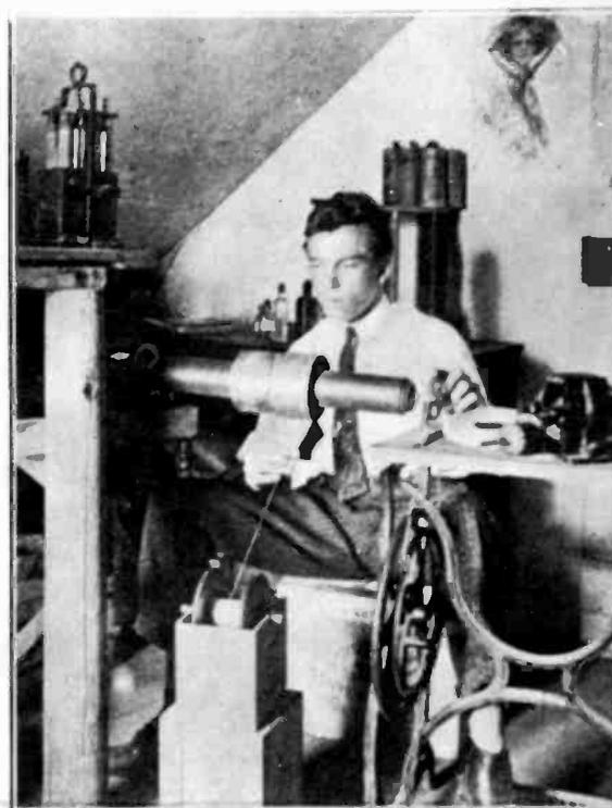
FAITOUTE MUNN, OF EAST ORANGE, N. J., AGE SEVENTEEN, IS HERE SEEN USING AN OLD SEWING MACHINE TO WIND HIS COIL.
