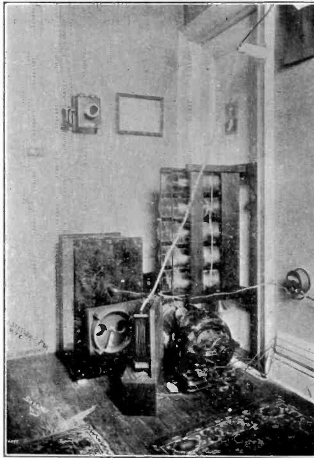
*Transmitter, Station "2PM", which produced the first transcontinental signals in 1916. Note the synchronous rotary gap mounted between motor and generator, large plated Leyden jar condensers and 1 K.W. United Wireless coffin transformer. This was the very latest equipment at the time.*
