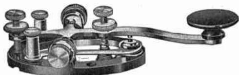
**T**HIS key is especially serviceable for C. W. transmitting sets. The contacts are made of 1/8-inch sterling silver and, besides being interchangeable, are easily replaced. The lever arm is both light and durable and is designed to permit an operator to secure the utmost speed possible. The frame and other metal parts are brass, finely lacquered.
