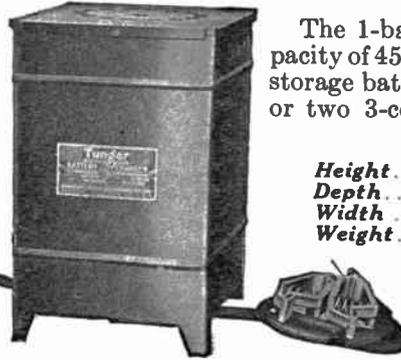
The 1-battery TUNGAR has a capacity of 45 watts and will charge a 3-cell storage battery at 5 amperes or a 6-cell, or two 3-cell, batteries at 3 amperes.
