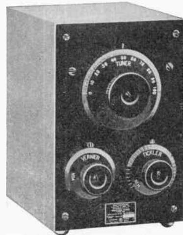
**T**HIS high-grade regenerative tuner has been designed for telegraph and telephone reception of transmitted wave-lengths between 180 and 700 meters, and will therefore receive both amateur and ship signals when used in connection with an antenna having a capacity of 500 micro-micro farads (.0005 microfarad) or more.
