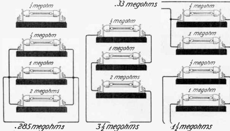
**The Radio Corporation Grid Leak Units are manufactured in the following sizes:**
