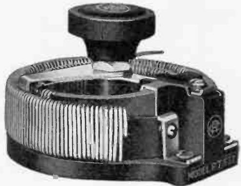
**R**HEOSTAT, Model **PR-535**, consists of a moulded base, approximately 2½ in. in diameter, on which are secured two concentric windings held securely in place by clamping screws. Connection is made to these windings by means of two sliding contacts of phosphor bronze, which form a circuit between the outside and inside windings. They are so shaped as to make continuous contact with at least two turns of wire, thus reducing tube noises during adjustment.
