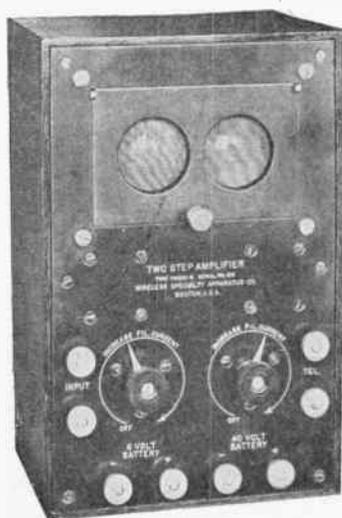
**T**HIS two step amplifier is a compact unit of the resonance low-frequency type. It provides a maximum of amplification due to the transformer design, which is greatly superior for radio reception to other types on the market. The input impedance of each tube is automatically controlled by the filament rheostat.
