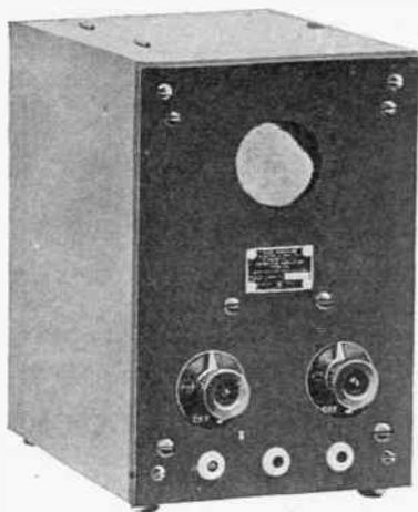
**T**HIS unit is an exceedingly compact detector and two-stage amplifier of the vacuum tube type, and is used when a receiving equipment more sensitive and efficient than a crystal detector is desired. It provides a vacuum tube detector and two stages of audio frequency amplification.
