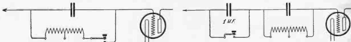
The proper location of the telegraph key in C. W. transmitting circuits is determined by the size of the RADIOTRON power tubes used. In circuits employing one or more UV-202 RADIOTRONS, satisfactory keying can be obtained by inserting the key in series with the grid leak resistance as shown above.
