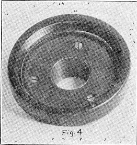
sink the screw holes in the back of the receiver-cap so that when the two are screwed together the screw heads will be flush with the cap (Fig. 4). If you are unable to make this cap, there is a cap on the market made for attaching a receiver to a phonograph that sells for a reasonable price.
