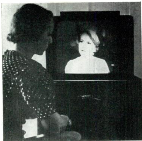
The mirror-lid of this television receiver reflects a picture measuring 12 by 14 inches off a vertically-mounted cathode-ray tube. This set was introduced to the Berlin market and is similar in many respects to models developed in American laboratories.
