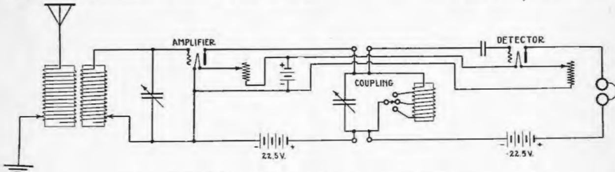
Fig. 2. Complete connections for the radio frequency amplifier
