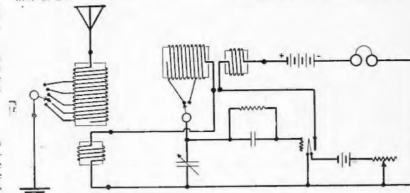
Fig. 3. Connections for the regenerative receiver
