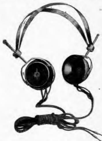
has resulted in the Manhattan Company placing upon the market receivers of their own product. The headband is designed for sanitation, being made of flat spring steel, rubber-janned with no covering. The sliding friction grip method of adjustment is employed. The case proper is flush on the back and the cord tips are concealed within the case. It is made in two types, 2000 and 3000 ohms.
