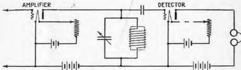
Fig. 1. A simplified circuit of the amplifier
