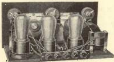
Fig. 4. Illustrating the patented Unipanel tray construction used in all KODEL receivers.
