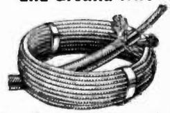
Size 18 stranded inner conductor. Rubber insulated with outer braided shield of tinned copper wire. When used as lead-in, by grounding the outer shield to the car frame, the tendency to pick up ignition noise and other static between aerial and receiver is practically eliminated.
