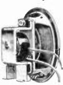
**250 Ohm Field, Voice Coil 1/2", 2 Ohms Impedance**
