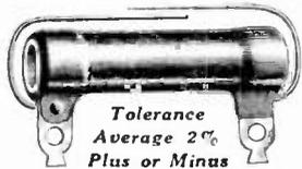
Wire wound on a 1/2" porcelain tube 1 1/2" long with a 1/4" hollow center. Coated with high quality Vitreous enamel and fired at red heat making an enamel coating which is fused tightly to the wire, terminal connections, and base. Either the solder lugs and 1/2" tinned wire leads may be used for mounting in air circuit.
