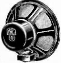
**Model A-12 P.M.**—Equivalent in performance to Model A-12 D.C. Voice coil impedance 8 ohms at 400 cycles. Power handling capacity, 12 Watts (18 Watts peak). Speaker Dia. 12 1/2", D. 7 1/2", complete with output transformer.
