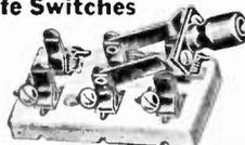
Glazed white porcelain bases. Copper contacts and blades with screw lug connections. Porcelain composition finger holds. Base lengths: S.P.— $2\frac{1}{2}$ "; D.P.— $3\frac{1}{2}$ ". Widths: 1" and 2". Rated 125 V., 25 A. For concealed or open wiring.
