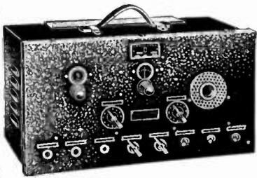
Uses a new simplified method of "wobble" that affords more stable operation and permits either single or double trace calibrated selectivity curve on oscilloscope.
