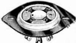
Exceptionally high dielectric strength, low power factor and high electrical resistivity. Easy to mount. Metal adapter plate can be screwed or riveted to panel or removed and socket mounted directly into chassis with wire retainer ring. Socket mounts in 1 1/2" hole (large size seven prong in 1 3/8" hole). Slotted holes in steel adapter plate 1 1/2" to 2" mounting centers. Approved by U.S. Army and Navy. Used by United States Signal Corps and wherever a low loss high quality socket is required.
