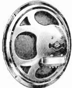
Uses no field current and does not require output transformers. Delivers good volume without distortion. True dynamic tone quality. Chrome steel permanent magnets. Heavy laminated silicon steel armature. 5" and 6" sizes will handle up to 2 watts, 8" size about 3 1/2 watts, 12" size about 6 watts.
