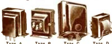
**K6640**—Primary 5000 ohms center tapped. Matches plates of Pushpull 2A3 self bias, P.P. 13's class AB self bias, 48 tetrodes. Secondary tapped at 4, 8, 15 or 500 ohms. Type A. Size: 3 1/2"x2 3/4"x3. List Price, \$4.00. Code T-6754.
