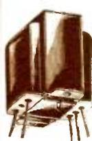
Turn ratio 25 to 1. Impedance ratio 625 to 1. Frequency curve is exceptionally flat from 80 cycles to 5000 cycles. Primary is split 200 ohms each side and the secondary impedance is of the order of 250,000 ohms at 60 cycles and 3 volts A.C. Matches impedance of all standard type, carbon, 2 button microphones. Fully shielded in black enameled steel case. Insulated core coiled 50" leads out of bottom. Size: 2 3/4" high, 2 1/2" wide, 2 1/4" deep. Mic. hole centers 2 3/4".
