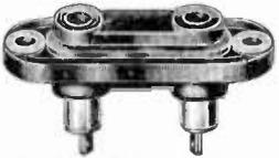
Fully insulated finest quality tip jacks molded in genuine bakelite. Phosphor bronze positive contact for any standard phone tips. Widely spaced solder lugs tinned and pierced. Overall length 2", width 1 1/2". Mounting centers 1 1/4". Will mount in cut out 1 3/8" x 1/2". Priced far below its actual value.
