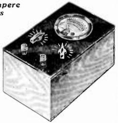
Build a Volt-Ohmmeter using any Weston Model 301, Jewell or Triplett. Patterns 88, 51, 444, 408, 489, 199, 133, 133A, 210, 538, 137, 137A, 374 or Triplett Model 321 meters requiring 1 milliamper for full scale deflection. The simplified dual scale multiplier range circuit is below. Ranges at 1000 ohms per volt—500, 250, 100, 50, 25, 10, and 5 volts; two ohm scales—0 to 1000 and 0 to 1 meg. with mid-scale readings of 50 and 9000 ohms.
