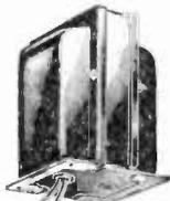
Designed especially to provide proper voltage regulation and filtering required to obtain maximum efficiency from tubes such as type 6L6. Inductance 10 henries at 150 milliamperes. (30.3 henries at 0 ma.) D.C. resistance 200 ohms. 2000 volt insulation. Fully shielded. Sub-panel leads, 8" long. Durable black enameled finish. Size 3 3/4" x 3 3/4" base, 4 3/4" high.
