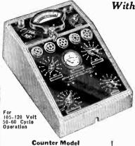
Tests all types of glass bulb and All-Metal Octal tubes without adapters. New laboratory fan type meter with knife edge pointer has English reading scale marked "Poor", "Doubfull" and "Good". Five sockets on panel. Extra points on switches for wiring in sockets to test future new tubes. Only three adjustments for tube quality test. Tests both plates of full-wave rectifiers. Line voltage adjustment meter.
