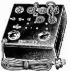
A low priced instrument which provides essential receiver testing and analyzing functions. Uses a sensitive neon glow indicator. Tests all tubes including the new octal Metal Envelope types by the cathode emission method. Requires only three simple adjustments of coded societ leads to make any test. Tube quality is accurately indicated by neon lamp when emission control is properly set. Positive indication of inter-element leakages and shorts up to 6 megohms.
