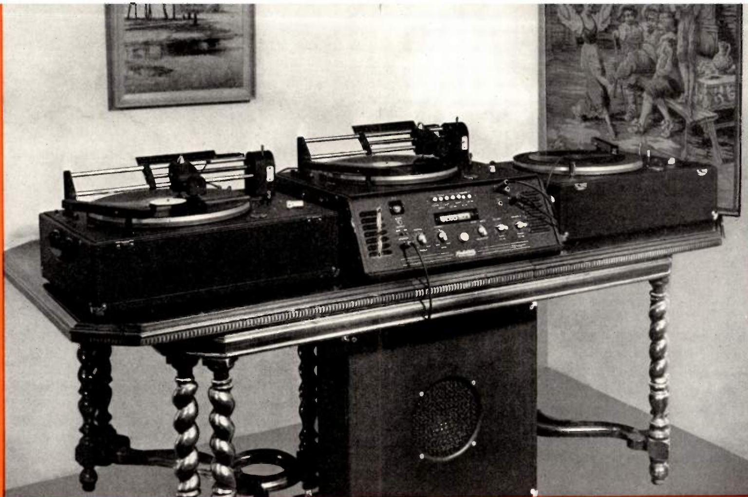
Model RA-16 Dual Speed Recording System as Pictured in Center Size—23" x 25" x 14½" Weight—84 pounds
