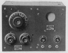
RADIOLA Model R. C. is a modern, compact and efficient Regenerative Receiver with a detector and 2 Stages of amplification incorporated in the same cabinet. It is in fact Radiola R A and D A combined.
