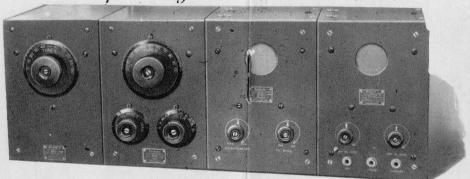
ADIOLA Super Selective Combination consists of Models RT primary coupler; RA secondary coupler; AR 3 stage radio frequency unit, and DA detector, 2 stage audio amplifier illustrated, in the order given, at the head of these pages. It is designed for use with an outdoor antenna for broadcast reception over long distances, and under conditions where extreme selectivity is desired.
