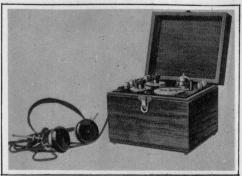
RADIOLA SR. is designed to fill the popular demand for an inexpensive set for broadcast reception with a greater range than a crystal set. Radiola Sr. makes use of the Regenerative Circuit in conjunction with a vacuum tube detector. A big feature of Radiola Sr. is that the filament of the vacuum tube may
