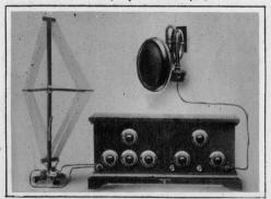
ITH Radiola VI, it is possible to obtain radio entertainment with the entire equipment installed indoors.
