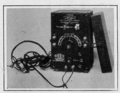
THIS crystal receiver was designed to cover a wave-length range of 170 to 2,650 meters. The set is sold complete with a pair of sensitive telephone receivers.
