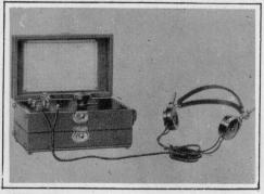
THIS practical receiver covers a band of wavelengths from 180 to 525 meters in two steps. These ranges are from 180 to 300 and 300 to 525 meters respectively.
