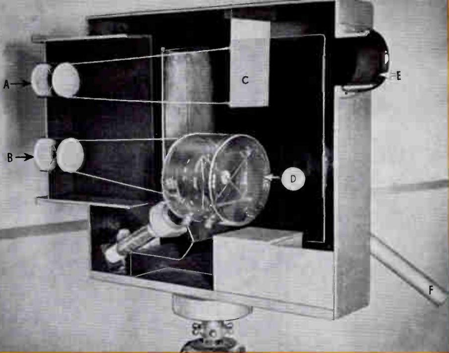
*Simplified cutaway model of television studio camera, indicating principal parts. A—Focusing lens for ground-glass. B—Lens which focuses image on Iconoscope plate. C—Ground glass. D—Iconoscope. E—Viewing aperture which permits operator to see the ground-glass image. F—Focusing handle.*
