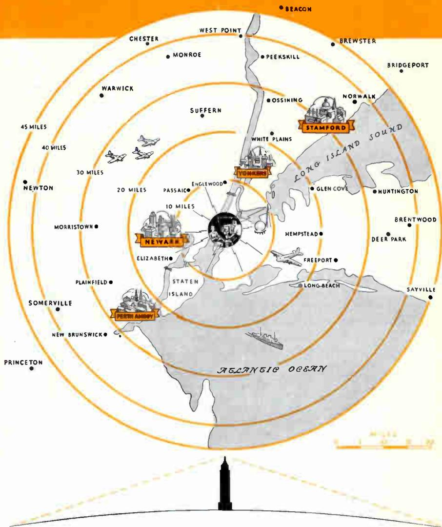
*This sketch illustrates roughly how the altitude of a transmitting antenna determines the area served by a television broadcast. The point where the dotted line touches the earth is the horizon, the theoretical limit of dependable coverage. Roughly, the range of the antenna, 1300 feet above Fifth Avenue, is about as far as your eyes can see from that elevation. (The vertical scale of this sketch is greatly exaggerated.)*
