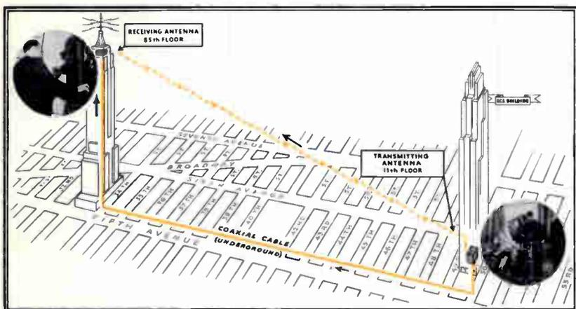
*Sketch indicating how NBC television signals travel from RCA Building Studio 3H (right) to the Empire State Building transmitter (left). The solid yellow line represents a coaxial cable. Television picture signals may also be sent from studio to transmitter by radio waves, indicated by the broken yellow line.*
