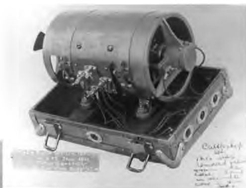
Figure 11. (Right) Motor Generator for long-wave Battleship type set, mounted in a separate case, perhaps to isolate its physical or electrical noise.
