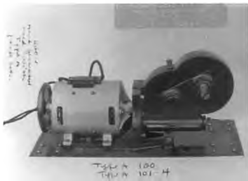
Figure 15. Hand Generator (handles not attached), supplied with Type A pack set made for the USN by N.E. Supply Co., 1912.
