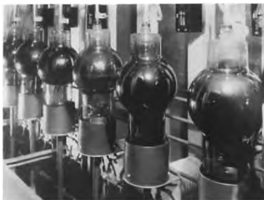
Figure 84. 870 mercury vapor rectifier tubes mounted in the rectifier cabinet of the 500-kW transmitter, 1934.
