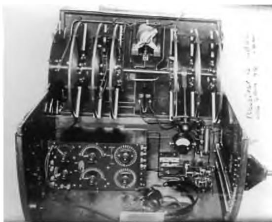
Figure 40: CN 241 by NESCO, with wavechanger and receiver designed personally by George H. Clark. Last of the NESCO spark pack sets for the Navy, made about 1917.
