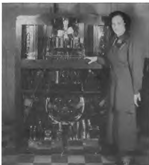
Figure 96. The Crosley "WLW Super Power" deluxe 37-tube radio receiver from 1934.
