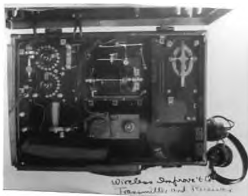
Figure 32. (Right) The Wireless Improvement Company, Type 200-B-1 pack set submitted for Schedule 6896, 1914.
