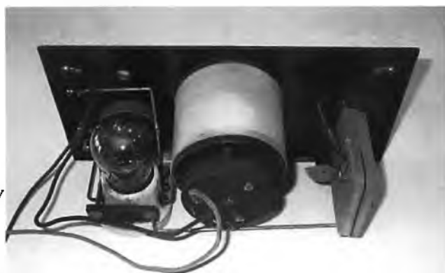
Figure 20. (Right) Crosley Model V Tri-City inside cabinet. (Courtesy of Robert White)
