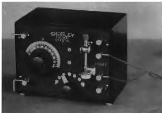
Figure 16. Crosley Crystal receiver Model I, 1922.
