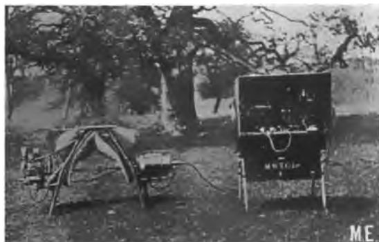
Figure 22. Marconi cavalry portable set. Note the shaft from the gasoline engine passing through the saddle and driving the generator, which is connected to the transmitting set by heavy leads. The saddle is equipped with a steel frame "so that it may be placed on the ground in the least amount of time." The receiving set consisted of a magnetic detector, along with headphones and a means of tuning.
