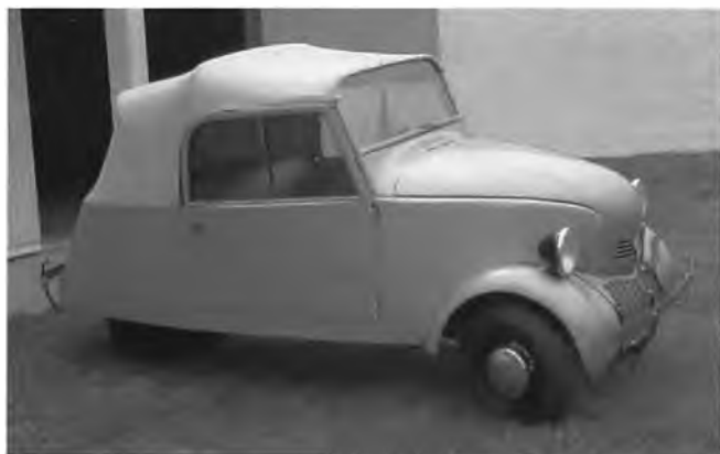
Figure 120. (Left) Crosley Grad automobile, 1939. Note the narrow 18-inch separation between the rear tires.
