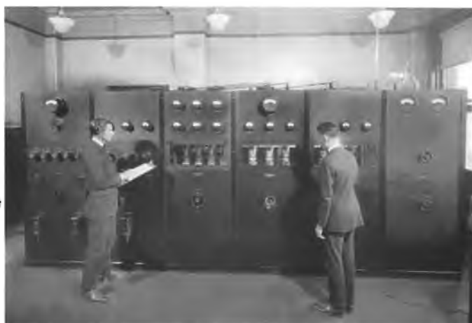
Figure 32. The Western Electric 5-kW transmitter for Crosley radio station WLW at Harrison, Ohio, 1925.
