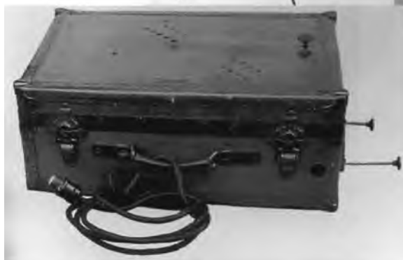
Figure 8. (Left) Sweet type Navy Pack Set. Knobs for generator speed, receiver tuning, and the sending key protrude through the case.
