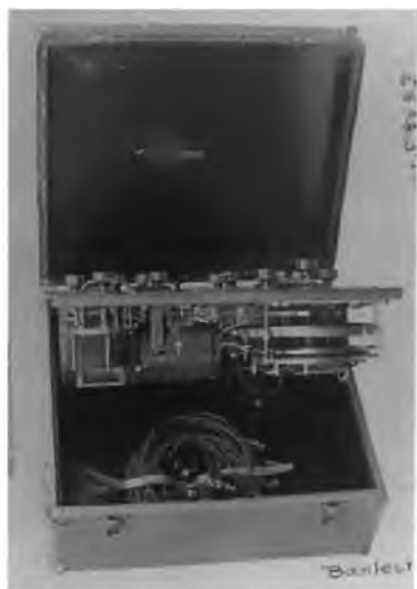
Figure 10. Battleship set, 1912, illustrating method of mounting components and false top.
