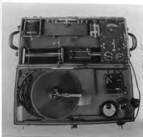
Figure 29. (Left) NESCO Type C transmitting and receiving chest, detail of break type key showing connections for shorting the receiver while the transmitter was in use. This allowed for listening in between transmitting spaces.
