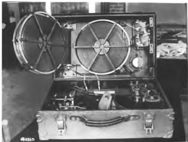
Figure 38: SCR-49, a 1916 model Signal Corps pack set. The receiver was the GE Type D. (Source: August Link.)
