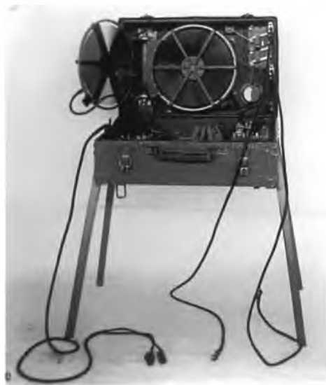
Figure 37: SCR-49 on supporting structure for operation. The supporting structure is the same as the one supplied with Signal Corps Model 1915. (Source: August Link.)
