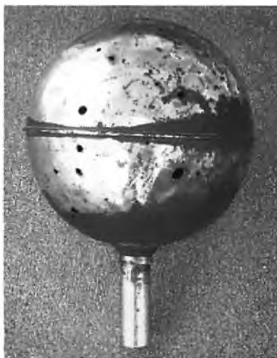
Figure 61. Ball removed from the top of the tower showing lightning strikes on top and bottom.
