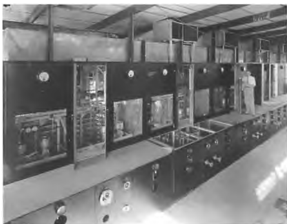
Figure 70. RF power amplifiers for the 50-kW transmitter prior to the installation of the UV-862 tubes, 1934.
