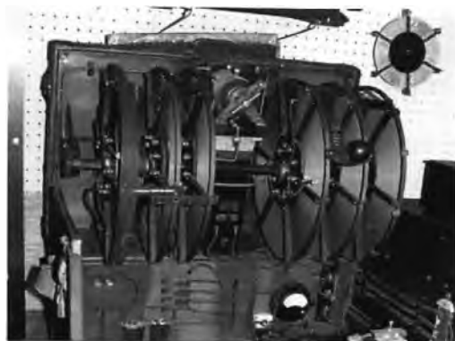
Figure 41: Detail of the special wavechanger made for the CN 241-253 type NESCO pack sets circa 1917. (Source: New England Wireless and Steam Museum)
