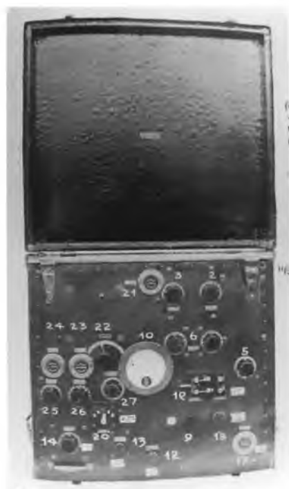
Figure 9. Battleship type NESCO pack set, 1912. Note that all the knobs are on top of a false top so the components remain dry underneath the real top.
