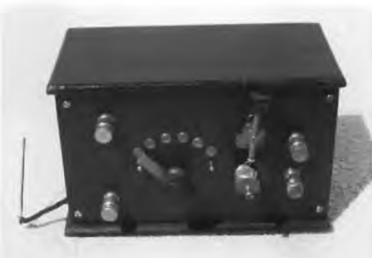
Figure 5. The Crosley Harko crystal receiver, showing the "poor man's buzzer" on the left side, 1921.
