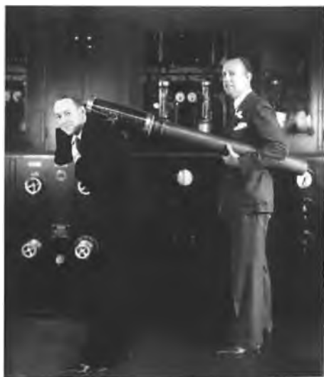
Figure 86. Powel Crosley Jr., and Joseph A. Chambers, WLW Technical Supervisor, hefting one of the UV-862 triodes used in the 500-kW transmitter, 1934.
