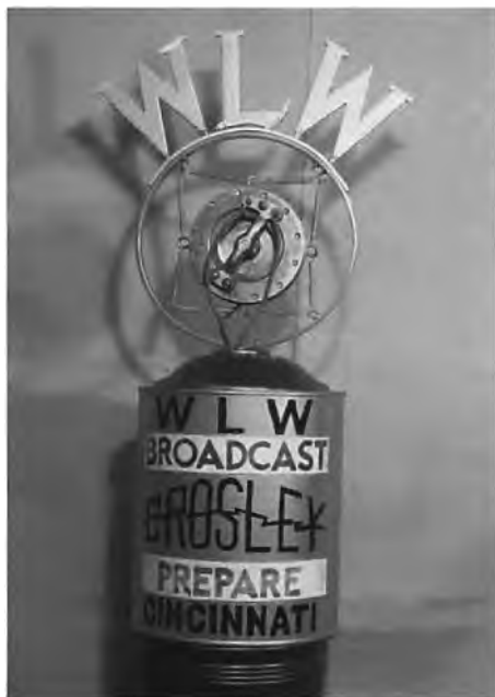
Figure 30. The WLW double-button carbon microphone in 1924.
