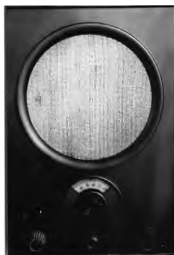
Figure 15. Volksempfänger 301 grille cloth; lighter color version. Note the pattern created with the precisely placed thicker thread which is indicative of a machine-created textile emulating the popular hand made textiles created at the Bauhaus. (Collection and Photograph; Barbara Havranek)
