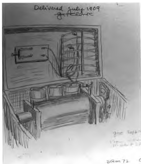
Figure 5. "Fleet" set made by NESCO about 1909 for the U.S. Navy, drawing by George H. Clark. Made up in a large pine box with an open spark gap and zinc electrodes. Only two of these sets were made.
