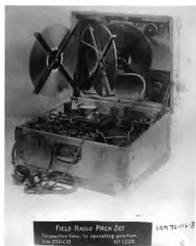
Figure 31. (Left) The WSA Co. "Type No. 250-C-15" Field Radio Pack Set for Schedule 6896, 1914.
