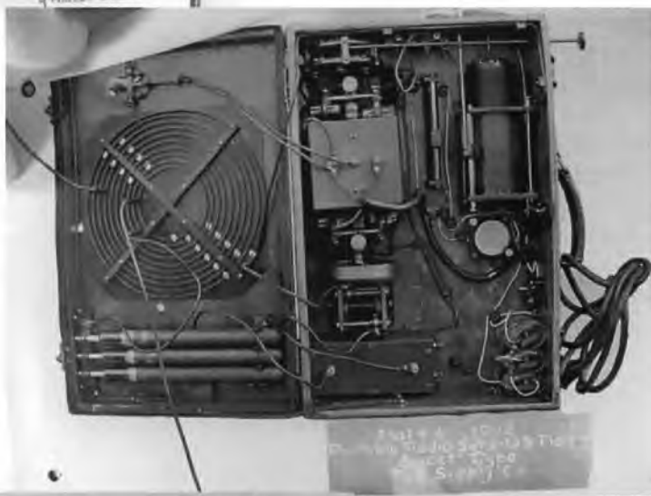
Figure 7. (Below) Sweet type Navy Pack Set. The first quenched gap set for the Navy made by NESCO.
