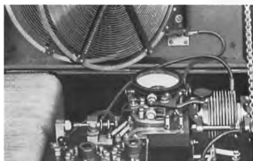
Figure 29. (Left) NESCO Type C transmitting and receiving chest, detail of break type key showing connections for shorting the receiver while the transmitter was in use. This allowed for listening in between transmitting spaces.
