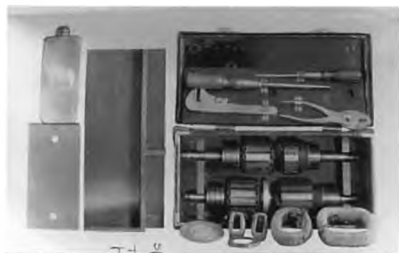
Figure 18. Motor generator supplied with NESCO Type B, C, D and E pack sets.
