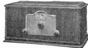
MODEL NR-66 —Single control, 6-tube Neutrodyne. Three stages Neutrodyne TRF (the first stage inductively tuned). Each radio stage completely shielded in separate metal compartment. Equipped with New Freed-Eisemann "Inductor". List Price . . . $125.00
