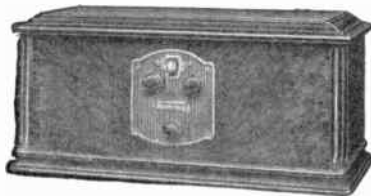
MODEL NR-77 —An advanced 7-tube, single control Neutrodyne receiver. Four stages Neutrodyne TRF and two stages audio frequency supplemented by output transformer. Equipped with Freed-Eisemann "Inductor". Each radio stage individually shielded. Audio frequency stages in separate metal compartment. New type loop. List Price (including loop) $175.00
