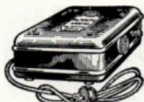
FIG. 114. Tobe Filterette 110-PO. This Filterette is suitable for application to electric refrigerators, fruit juice extractors, adding machines and practically all office appliances.
