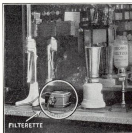
Fig. 31. Battery of drink mixers silenced by Filterette 110-PO.
