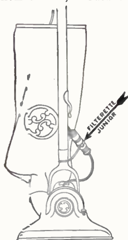
FIG. 21. Filterette Junior inserted in the attachment cord of a vacuum cleaner.
