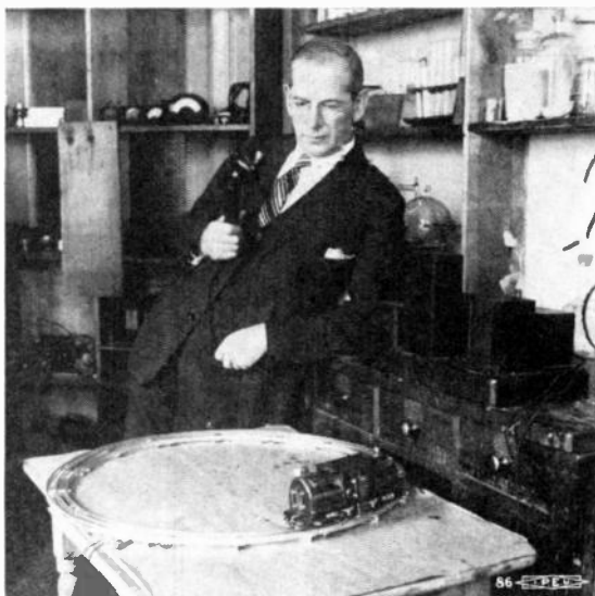
This little train does not talk but it acts humanly. Its movements are controlled entirely by sounds of the voice, stopping, backing and going forward at command. The secret lies in a one-two-three relay coupled to the microphone. W. W. Jones of the General Electric Co. is demonstrating the new toy.
