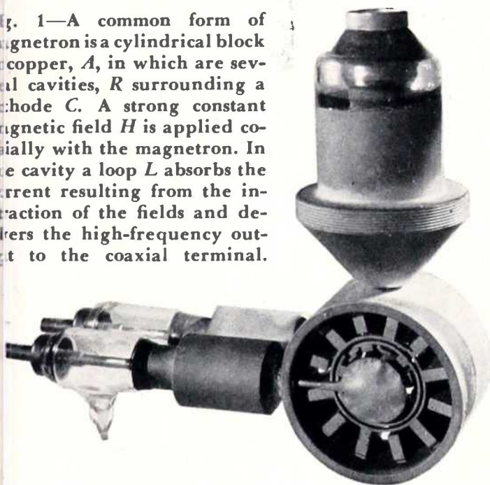
In this 10-cm magnetron the cavities, instead of being holes milled out of a solid block of copper, are formed by brazing vanes into a cylindrical shell. The tube delivers approximately 700-kw peak or pulse power.
