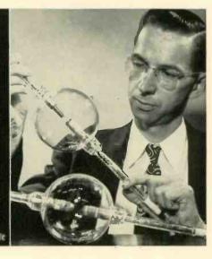
Such are some of the highlights of lamp-making progress. The evolution of lamp-making machines gains stature when it is considered that each of today's machines is capable of producing 8000 to 9000 lamps a day compared with the 300 turned out by the 1910 equipment.
