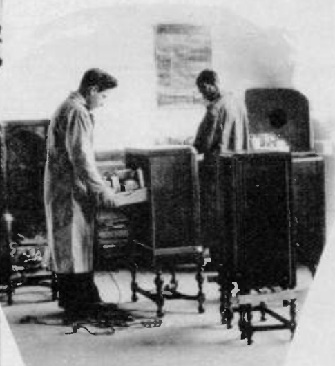
Every radio set goes through a final test of performance and efficiency before leaving our quarters. These men are constantly engaged in this work in our Final Test Dept.
